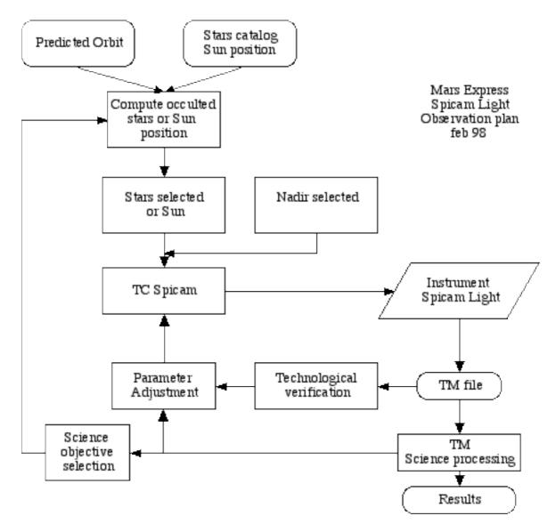
This diagram reflects the Spicav operations (diagram from MEX, valid for VEX). Interfaces during commissioning and routine phases will be described later.
