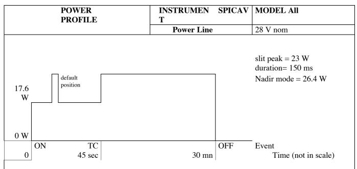
Actuators default position: Nadir configuration ( solar shutter closed, slit on )
