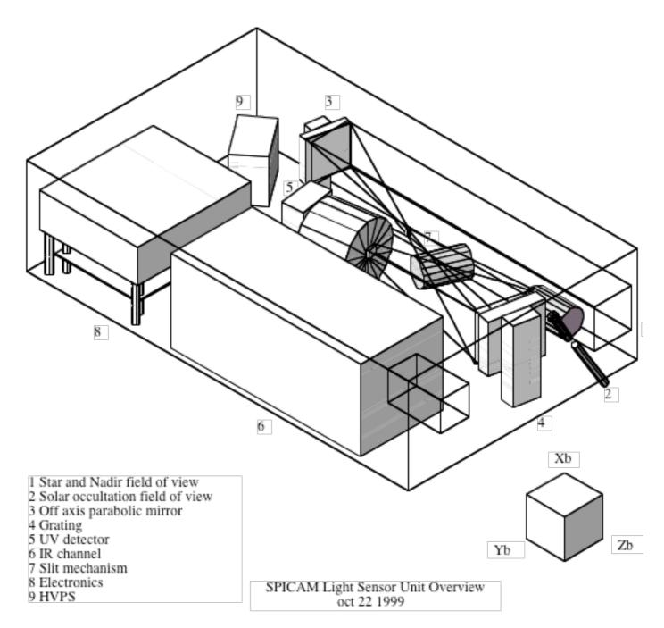
The Spicam part has two openings for Nadir viewing, one for UV channel, the other for IR channel. In addition, the UV and IR channels have an opening for Solar viewing (2).
