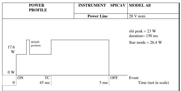
Actuators default position: Nadir configuration ( solar shutter closed, slit on )
