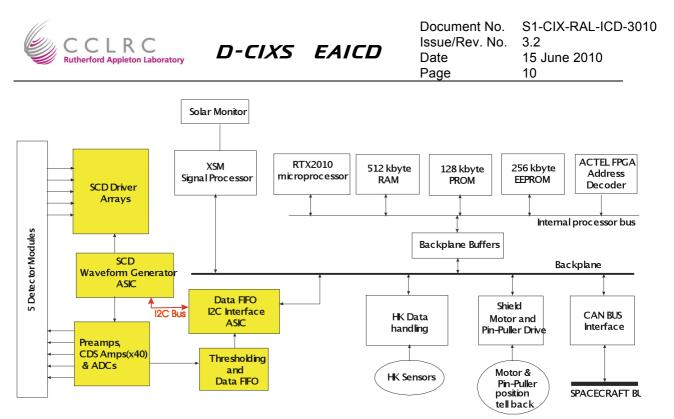
Figure 2-5 Swept Charged Device Readout System
