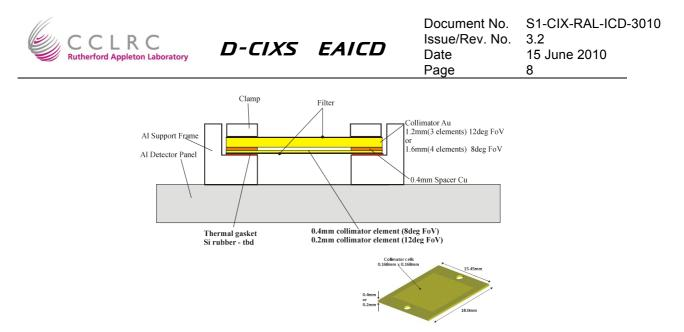
Figure 2-2 Detector Assembly
