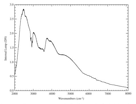
Fig. 13. Average of 200 Internal Lamp spectra. The effect of the mechanical vibration is almost absent.
