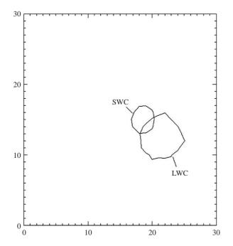
Fig. 6. FWHM for both channels LW and SW channels: the SW is  $1.7^{\circ}$  wide, while the LW is  $2.8^{\circ}$  wide. Note the displacement of the two channels of  $1.8^{\circ}$ . The two channels overlap only partially.
