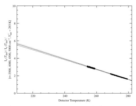
Fig. 11. Linear increasing of detector responsivity with decreasing detector temperature for different wavenumbers ( $\nu = 3500, 4000, 4500$  and  $5000 \text{ cm}^{-1}$ ). Values are normalised with respect to the room detector temperature (293 K).
