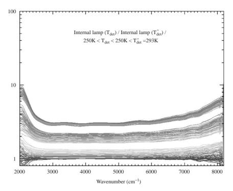
Fig. 10. Responsivity of the detector increase with its cooling.
