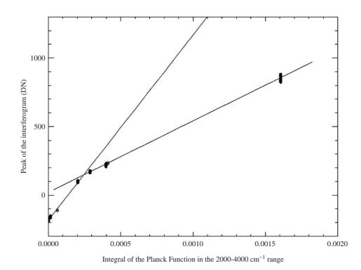
Fig. 3. Linearities of the SW channel in the thermal part. The peak of the interferogram is plotted versus the integral of the Planck function between 2000 and  $4000 \,\mathrm{cm}^{-1}$  for different temperatures (see text for details).
