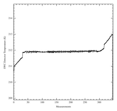
Fig. 1. Short wavelength channel detector temperature during a pericentre pass, Orbit 41, 22 January2004.
