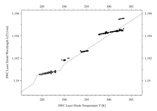
Fig. 7. SW channel laser diode behaviour with temperature.
