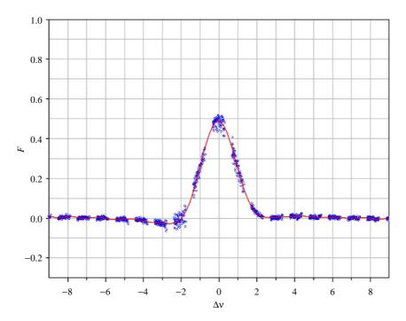
Fig. 9. The same as in Fig. 8, but apodised. Note that the spectral resolution becomes worse by a factor of 2.
