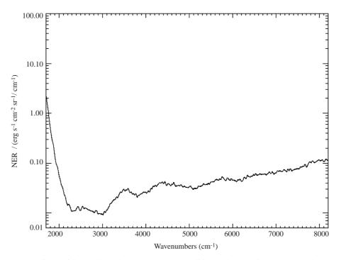
Fig. 16. The Noise Equivalent Radiance of the SW channel at space operating conditions. It is 10–20 times lower than the NER at room temperature (see Fig. 5)
