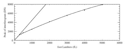
Fig. 2. Peak of symetrised interferogram versus source intensity.
