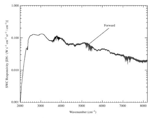
Fig. 4. Responsivity of the SW channel obtained in the Lab at room temperature and in air.
