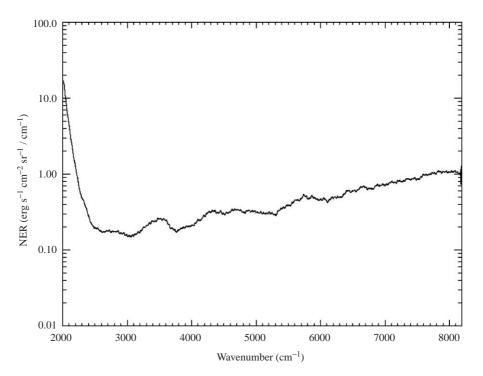
Fig. 5. Noise Equivalent Radiance for the SW channel at room temperature.
