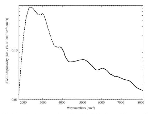
Fig. 15. Total Responsivity of the SW channel at space operating conditions, obtained joining the responsivities computed for the thermal (dashed) and the solar (line) range.
