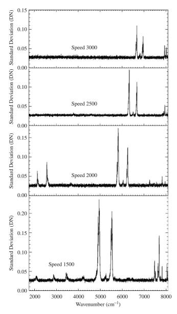
Fig. 12. Standard deviation for averages of 100 Deep Space measurements at different speeds of the double pendulum.
