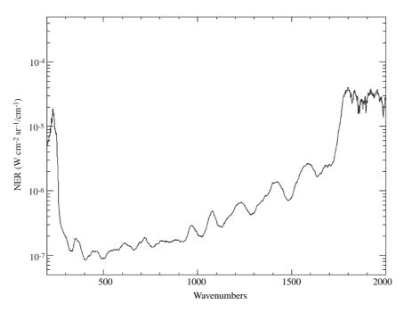
Fig. 8. NER obtained from the internal blackbody measurements in the thermovacuum chamber.
