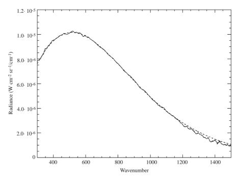
Fig. 12. Radiance of the internal blackbody obtained using Eq. (3.7) (line) compared with a theoretical Planck function of the same temperature (dashed).
