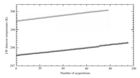
Fig. 3. LWC detector temperature variations during a session of measurements with the IFSI BB at 30  $^{\circ}$ C (bottom) and 50  $^{\circ}$ C (top)—laboratory measurements.
