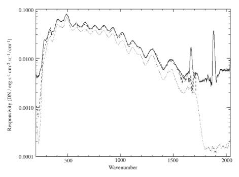
Fig. 9. Comparison between space responsivity (line), laboratory responsivity with IFSI blackbody (dotted) and IKI blackbody (dashed). This last curve has been truncated at 1700 cm<sup>-1</sup> for picture clarity.
