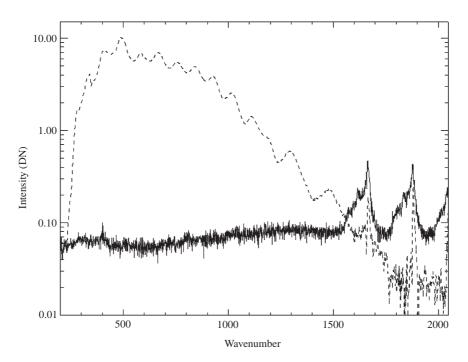
Fig. 1. Deep-space observation. Average spectrum (dashed) and sigma (line) in the LW channel.
