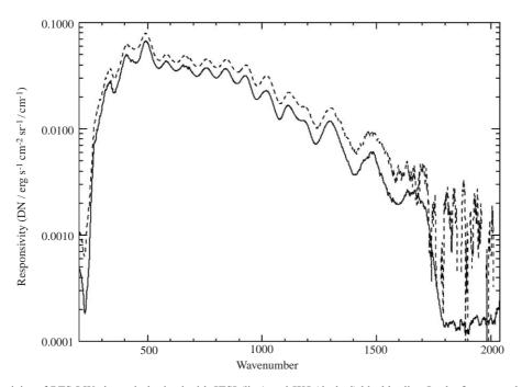
Fig. 5. Average responsivity of PFS LW channel obtained with IFSI (line) and IKI (dashed) blackbodies. In the first case, the source was warmer than the detector temperature while in the second case it was colder.
