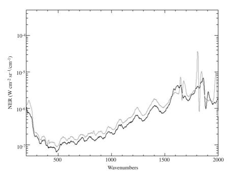
Fig. 15. PFS NER at nominal speed (black) and speed 2500 Hz (grey). The speed has just a little effect on the NER.
