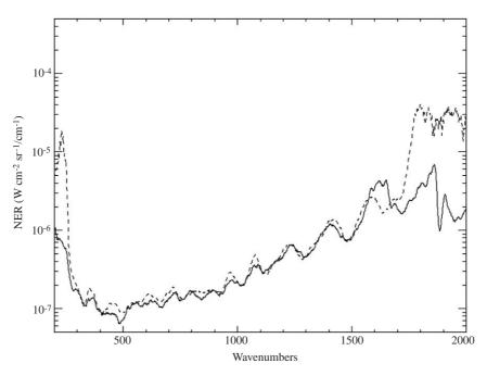
Fig. 13. Comparison between NER computed in space (line) and in laboratory (dashed).
