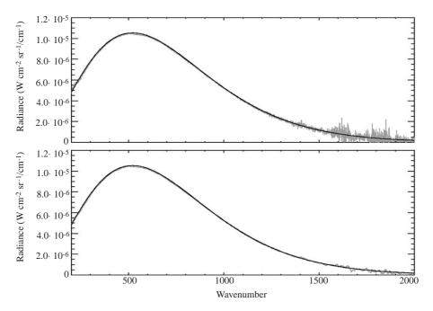
Fig. 10. Top: 50 measurements averaged radiance of the internal BB. Bottom: same curve smoothed over 11 points. Black curves are theoretical Planck functions. Note the perfect matching over the entire range.
