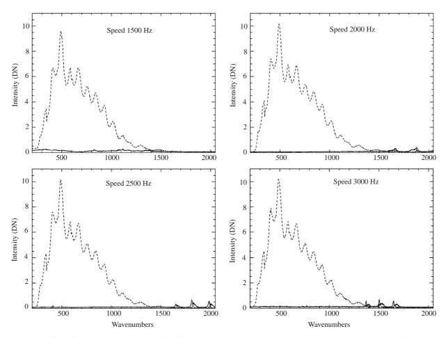
Fig. 2. The effect of the mechanical vibrations for different speeds. Averages and standard deviations are showed. See text for details.
