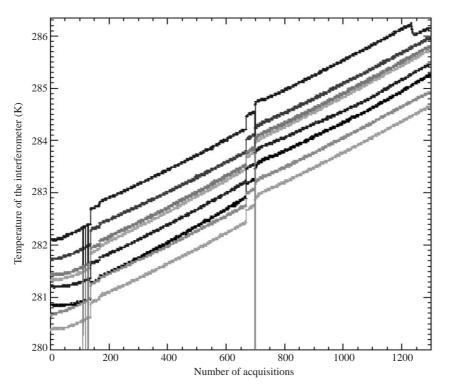
Fig. 4. Temperature of the interferometer monitored by eight thermometers during the NEV activity.
