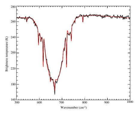
Fig. 19. A single PFS spectrum (black) obtained from apodised (Hamming) interferogram (lower spectral resolution) fitted by a synthetic spectrum (red).
