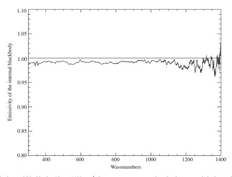
Fig. 6. Emissivity of the internal blackbody. Above  $1400 \,\mathrm{cm}^{-1}$  the measurements are noisy: the detector and the internal BB were very close in temperature.
