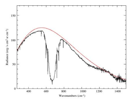
Fig. 17. PFS spectrum (average over 11 measurements) compared with a Planckian.
