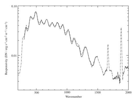
Fig. 11. Comparison between the responsivities obtained with Eqs. (3.6) (dash dot-dot) and (3.7) (line). This last curve is limited in the  $300-1500 \text{ cm}^{-1}$  spectral range, which is less affected by noise.
