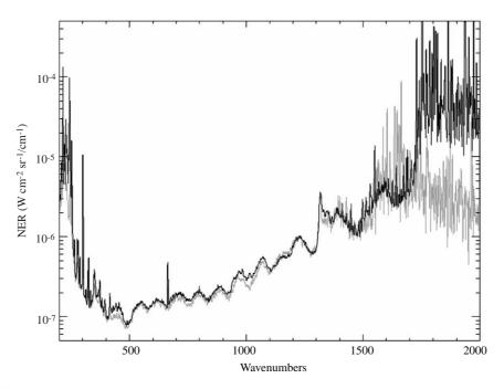
Fig. 7. NER obtained from IFSI (black curve—sources warmer than the detector temperature) and IKI (grey curve—sources colder than the detector temperature) blackbody measurements.
