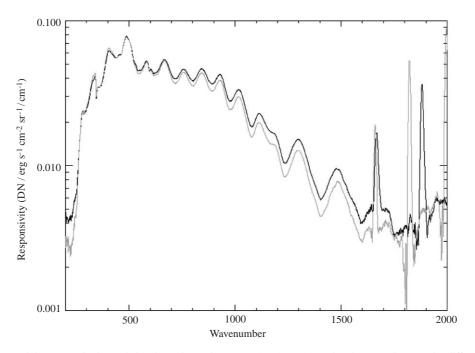
Fig. 14. PFS LWC responsivity at nominal speed (black) and speed 2500 Hz (grey). Eq. (3.6) has been used. Note the difference between the two curves, with the 2500 Hz responsivity being a bit higher before  $500 \,\mathrm{cm}^{-1}$  and lower above.
