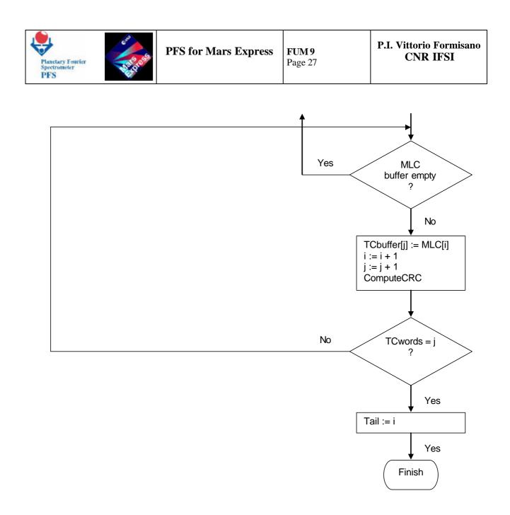
At this moment the whole Telecommand has been received in the buffer *TCbuffer*. The decoding of the Telecommand can be illustrated by the following flow diagram.
