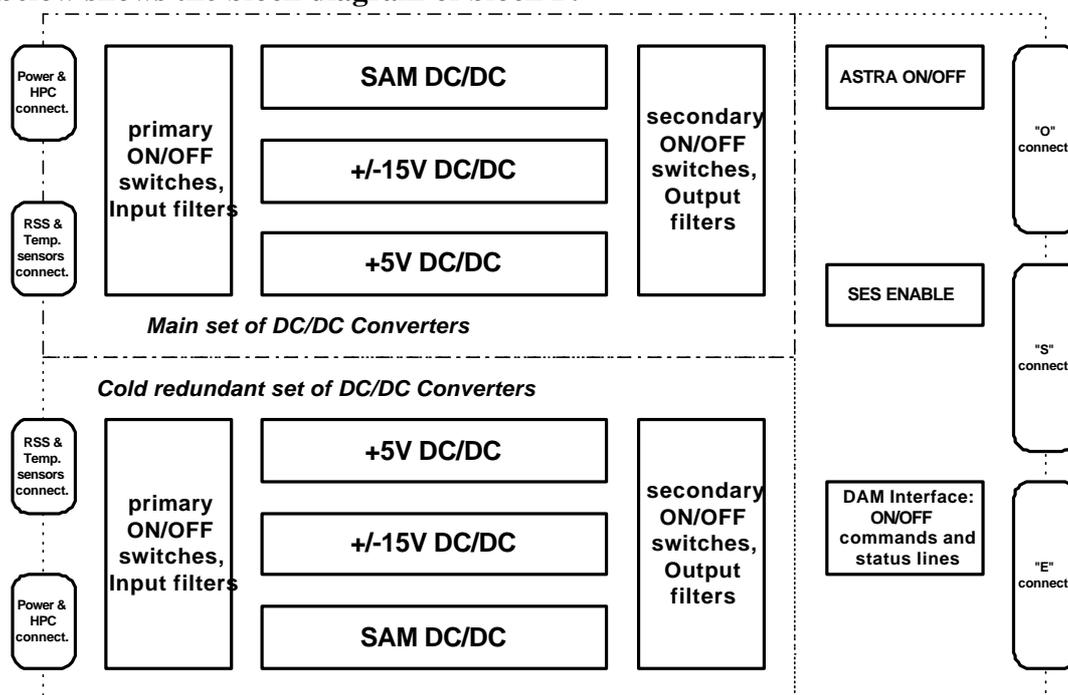
Each of independent converters works at 131 kHz with variable pulse width. Siliconix Si9110 is used as PWM controller, the feed back loop is closed magnetically. Overvoltage and overcurrent protections are built-in.
