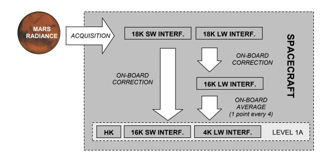
Fig.2 PFS data acquisition and processing scheme.
