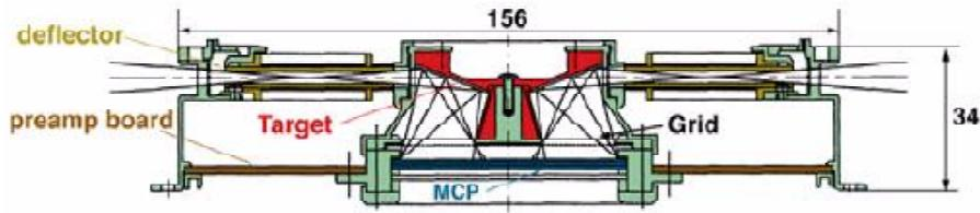
**Figure 1.** *Cut-away view of the NPI sensor*
