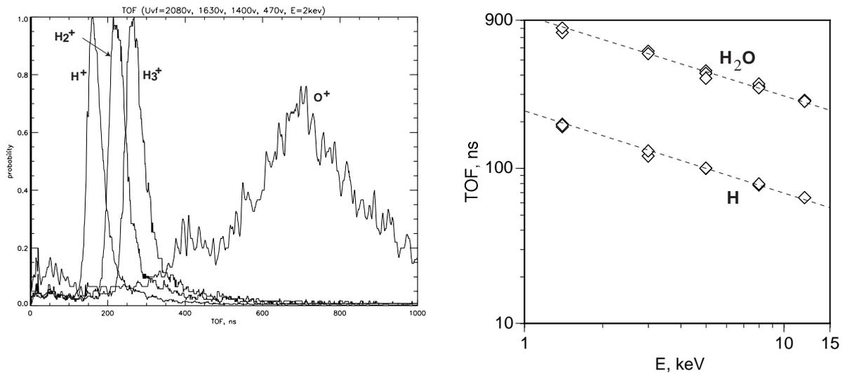
**Figure 7.** Mass resolving capability of the NPD sensors using pulse-height analysis of the STOP MCP-detector (left) and time-of-flight analysis (right)
