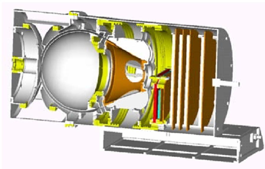
**Figure 4.** *Cut-away view of the IMA sensor*
