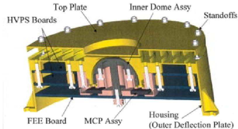
**Figure 3.** *Cut-away view of the ELS sensor*
