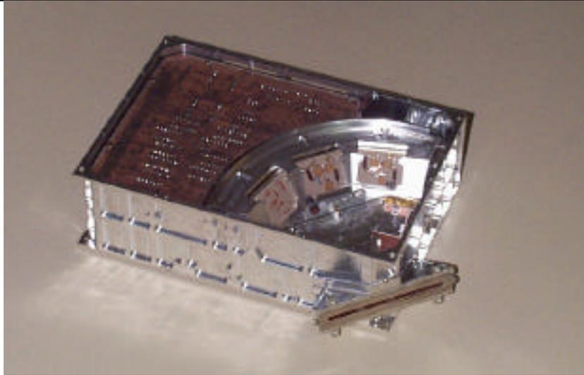
**Figure 11.** Technological model of the NPD sensor
