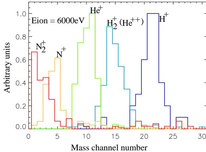
**Figure 8.** *Calibrated Ion Mass Analyzer mass resolving capability of 6 keV ions*
