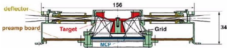
**Figure 1.** *Cut-away view of the NPI sensor*
