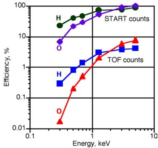
**Figure 6.** Efficiency curves for the START and STOP sectors of the NPD instrument.
