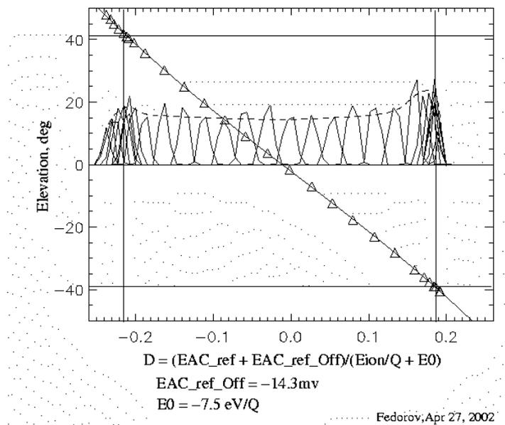
**Figure 8.** *Calibrated elevation angle response of the Ion Mass Analyzer*
