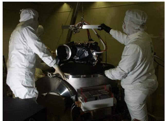
Figure 36. OSIRIS in ground calibration.
