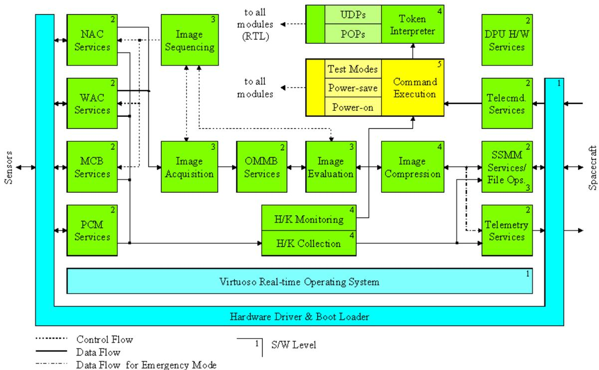
Figure 34. Interaction between software modules within OSIRIS.
