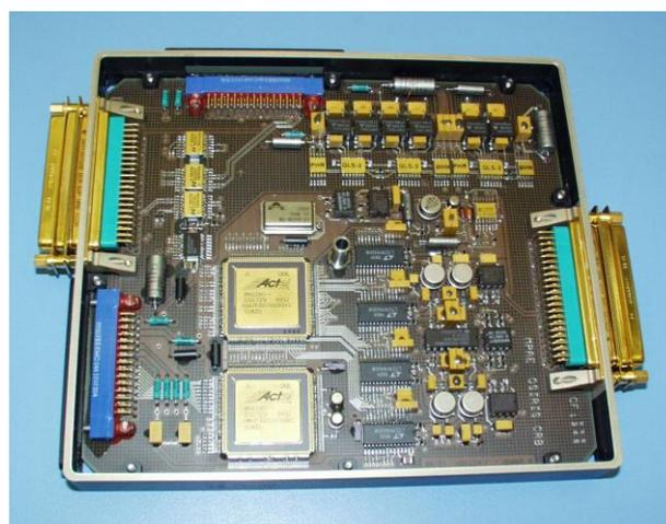
Figure 23. The CCD Readout Board.
