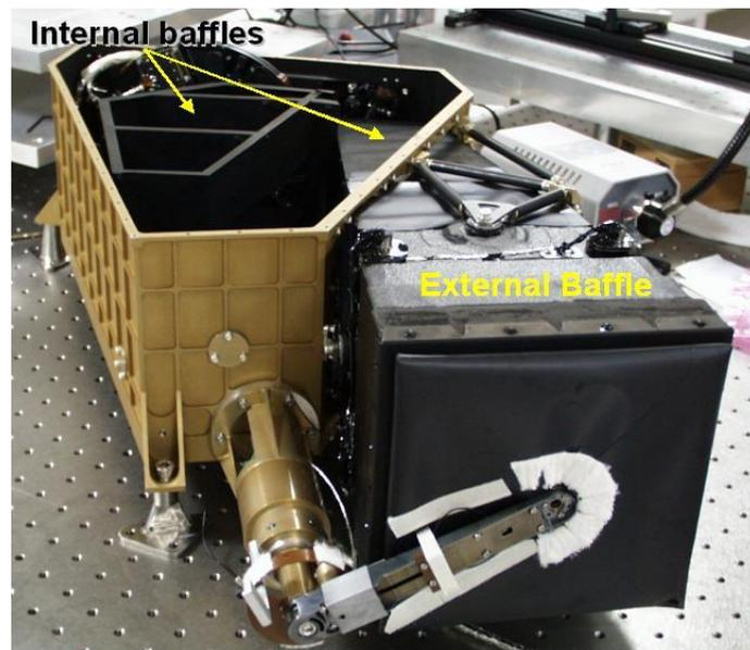
Figure 14. Concept and view of the WAC baffle.
