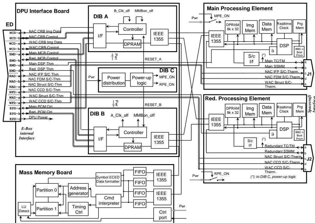
Figure 26. Block diagram of the OSIRIS DPU architecture.
