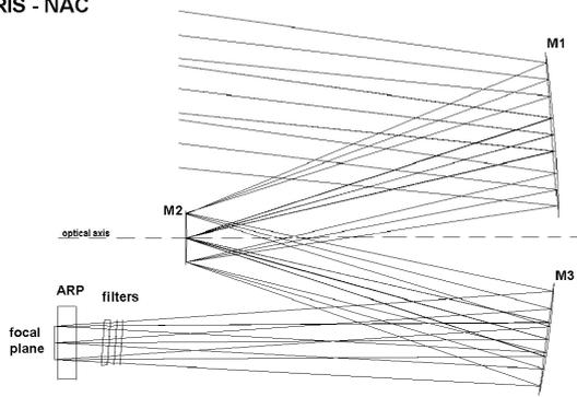
Figure 6. Ray paths through the NAC optical system.
