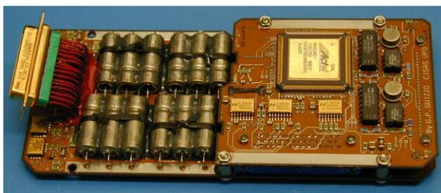
Figure 20. Shutter electronics board.
