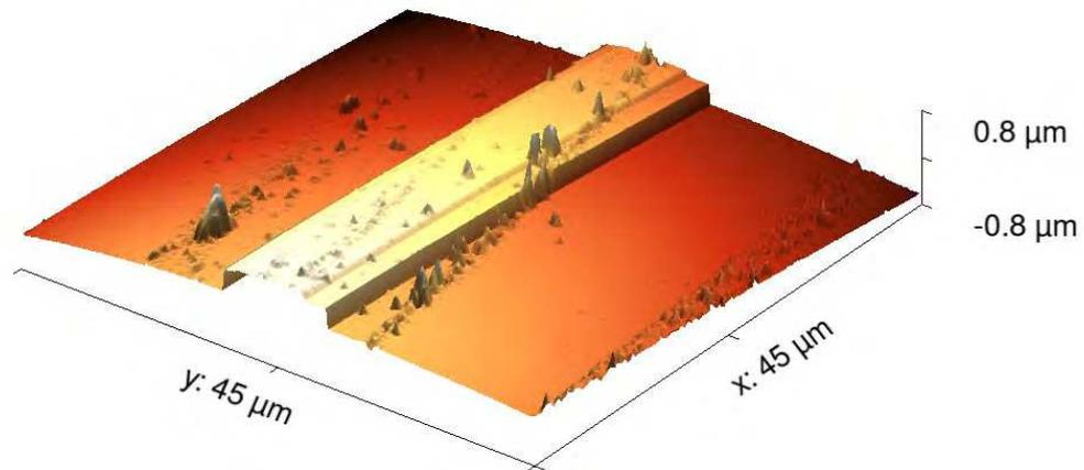
Figure 2. 3D image of STP004-6 showing odd height feature at centre of target and contamination features.
