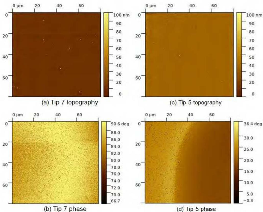
Figure 24: Comparison of tip 7 (a, b) and tip 5 (c, d) topography and phase channels, revealing a distorted scan with the higher Q-factor tip 5 at the right half of the scan. The phase image is showing a severe transition from the left half of the image to the right.
