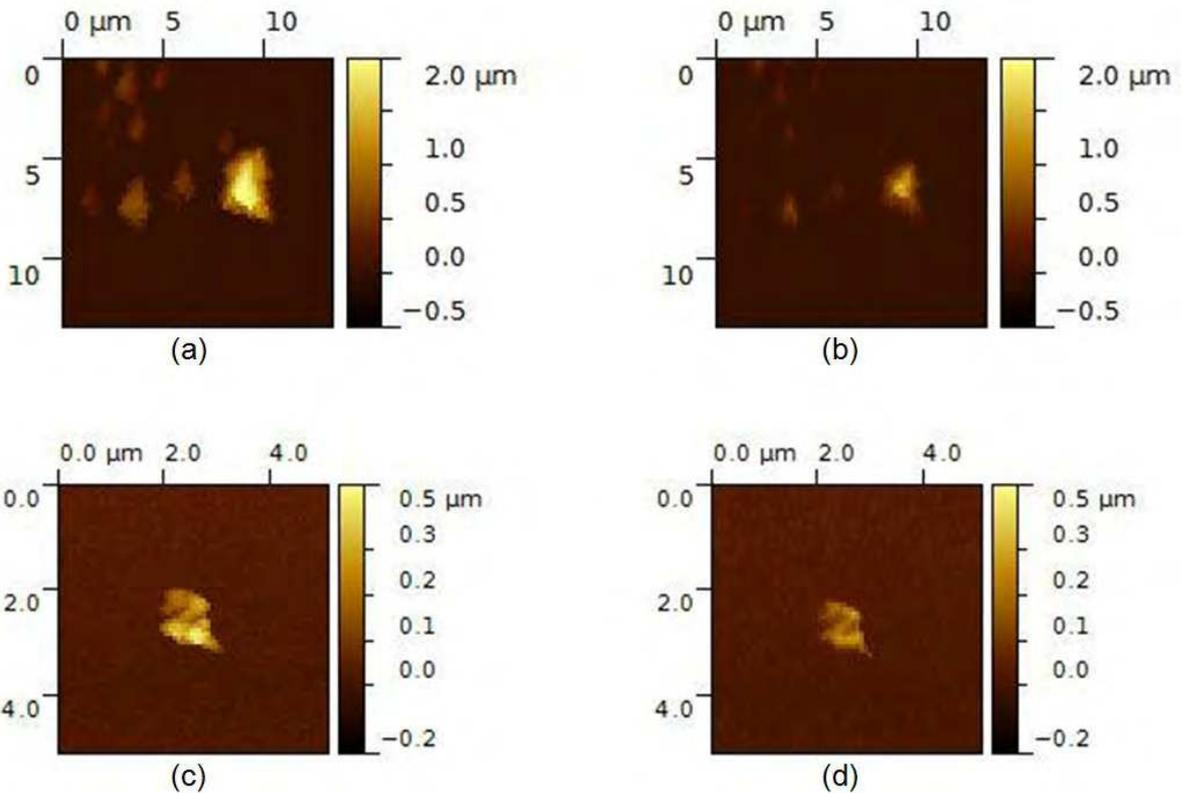
Figure 21: Topography image of a cometary particle with tip 7 (a) and with tip 9 (c). The particle size is in both cases in the order of 2-4 μm and the size is from approximately 450 nm to 2 μm for the particle in (c) and (a) respectively. (b) and (d) show the deconvoluted image where the tip was taken from figure 3.03. Both show a decreased structure height and other artefacts.
