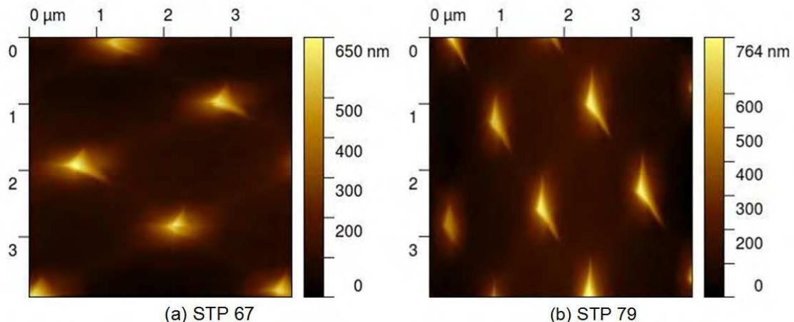
Figure 2: Tip images of tip 8 from STP 67 (a) and STP 79 (b) revealing no severe change of the tip shape after 10 scans in contact mode at a silicon facet.
