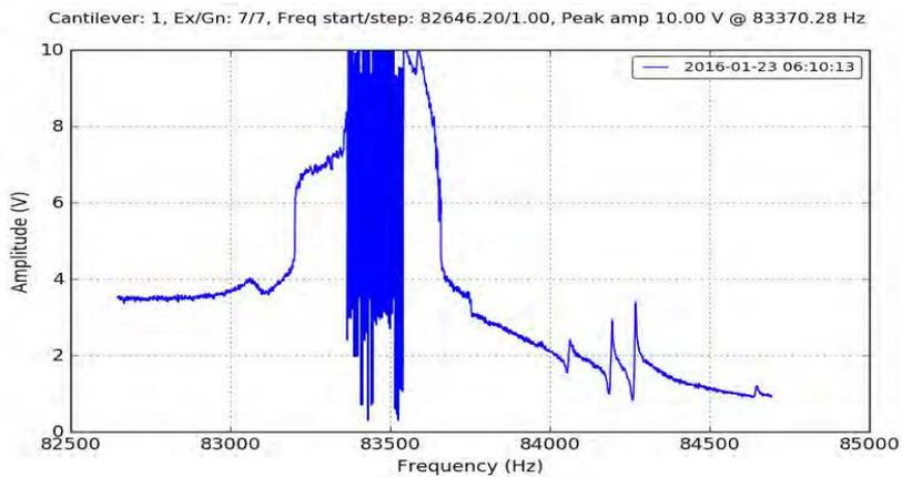
**2016-01-23 06:14:28 : Z piezo / strain gauge tests**
