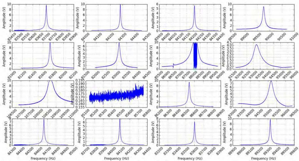
2015-10-28 05:25:52 : 10 high excitation resonance sweeps to shake off material from tip
