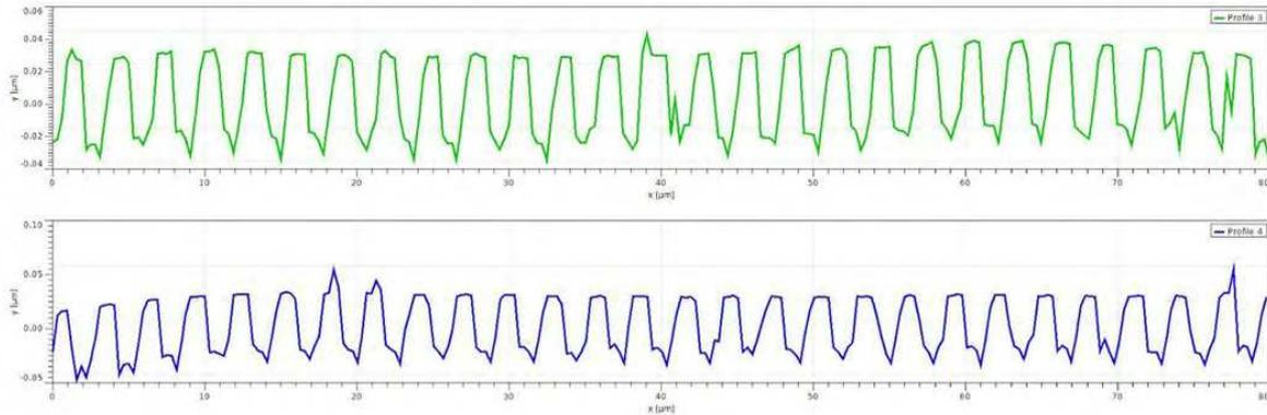
Figure 17: In (a) and (c) open loop topography image and line cross sections and (b) and (d) hybrid mode topography image and line cross sections are shown for revealing the different dimensions of the calibration standard structures.
