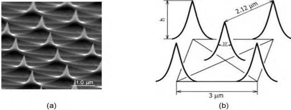
Figure 19: Tip imaging sample mounted at both the flight spare and the flight model. (a) SEM image and (b) schematic illustration showing the dimensions of the sharp tips used for imaging of the AFM tip.
