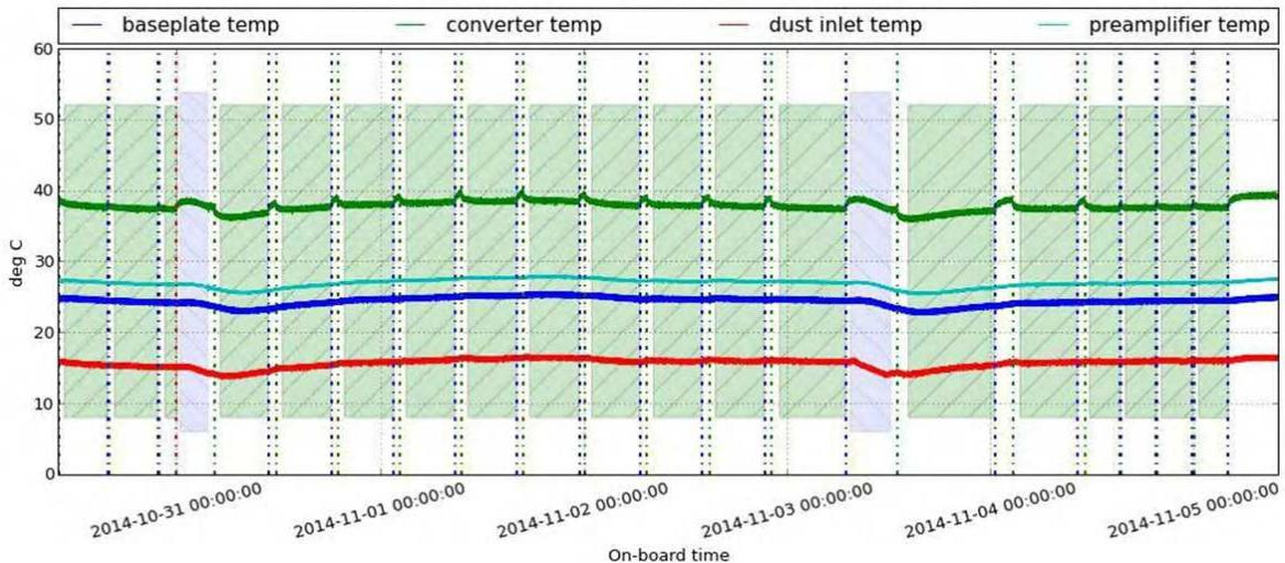
Figure 8: Temperature of the four sensors during STP 26 with most of the time used for scanning (green blocks). At the beginning of the first OCM (blue block) a scan gets aborted due to little time left and MIDAS going to a safe state during the OCM. After both OCM a small increase due to the approach can be observed and after each scan the temperature increases also for approximately 1 °C.
