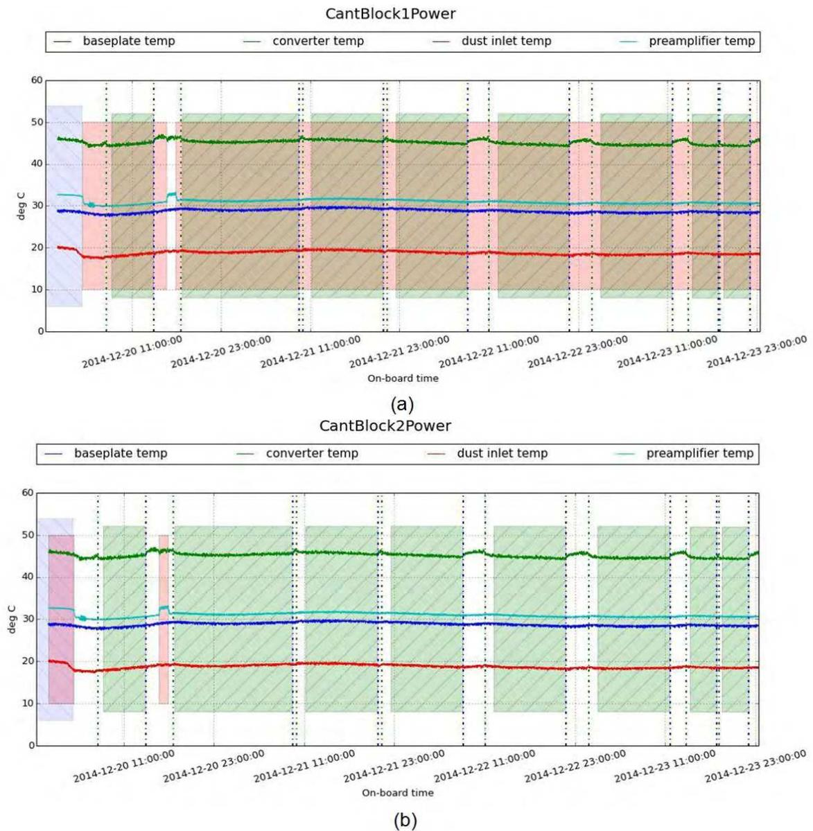
Figure 7: Marked in red is the power status of the cantilever block 1 (a) and 2 (b), revealing a temperature jump by switching between those two, especially at the preamplifier temperature.
