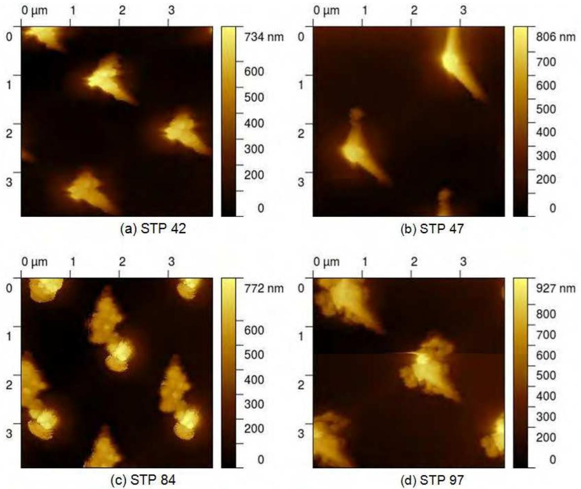
Figure 23: Tip 9 tip images from diverse STPs revealing a different amount of contamination, but tip wear seems not to be dominant.
