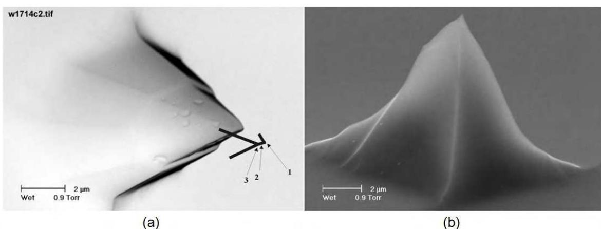
Figure 18: SEM images of the AFM tip before (a) the last etching step and (b) the final version of one tip at the flight model, revealing the tip shape to be formed out of a knife blade form to the final sharpness.
