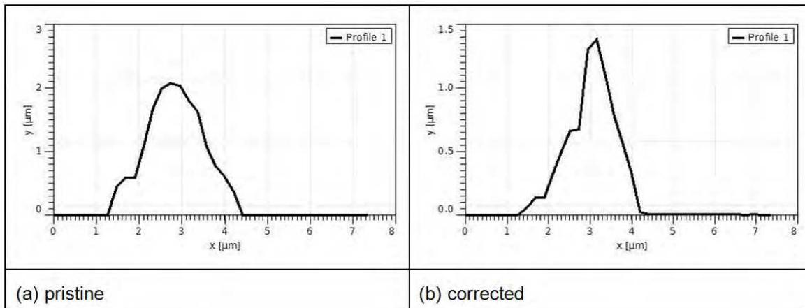
Figure 22: Line cross sections of the uncorrected (a) and corrected (b) particle showing a decreased particle height and an additional step induced at the post processing.
