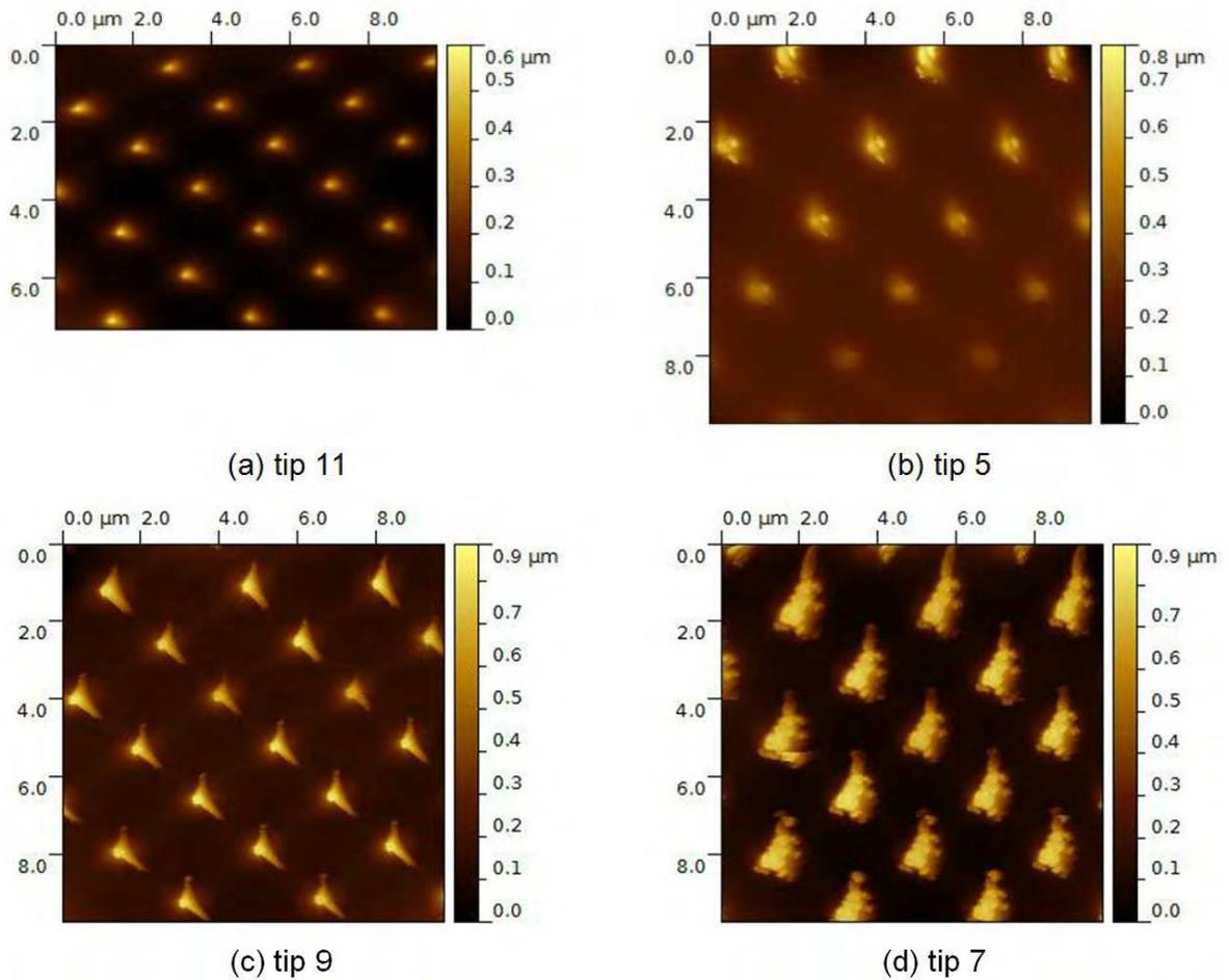
Figure 20: Tip image of tip 11, 5, 9 and 7. In (a) tip 11 shows nearly no wear and a very sharp and uncontaminated tip. Tip 5 (b) is contaminated with a few particles, but some change in image quality from top to bottom can be observed here. Tip 9 (c) shows a plateau and a blunt tip. Tip 7 (d) shows the most contaminated and worn status.
