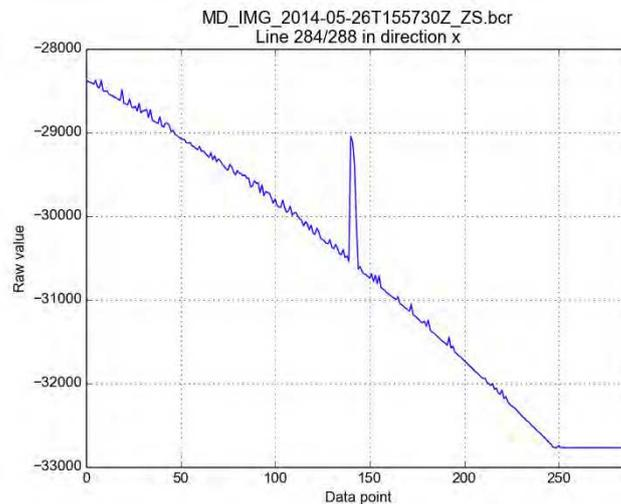
Figure 1. Z piezo extension (y axis in raw instrument values) during scan STP004-3, showing Z piezo reaching maximum extension towards the end of the scan.
