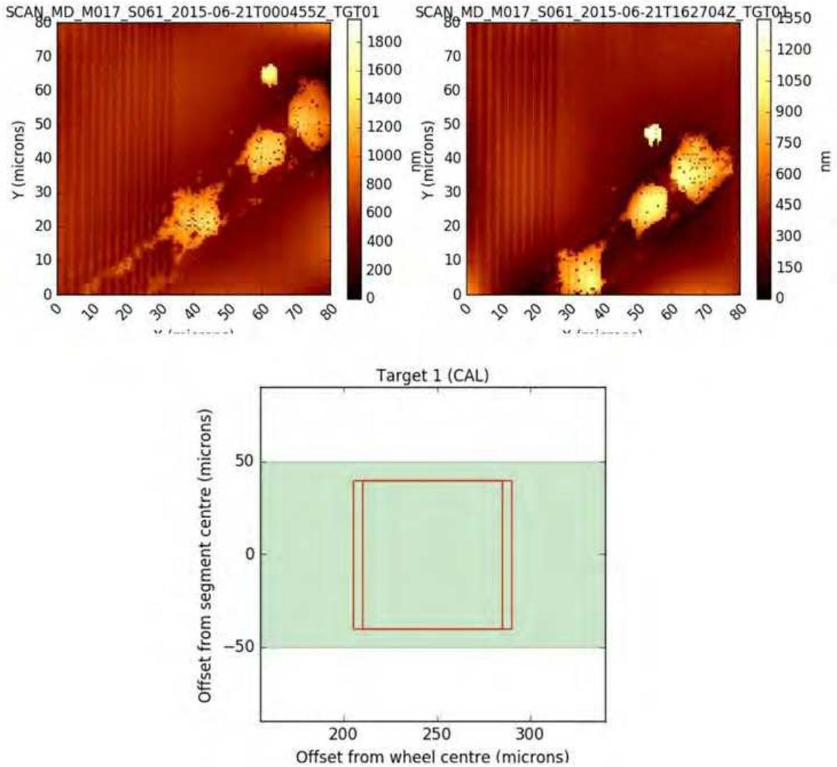
Figure 27: tip 10 (top left) and tip 15 (top right) scan of the edge finding feature, revealing a correct offset in X direction, but showing an offset in Y direction of approximately 15-20  $\mu\text{m}$ . The bottom illustration is showing the X corrected positions, but the nominal Y position is still showing the same value, which is clearly not the case when looking at the two scans.
