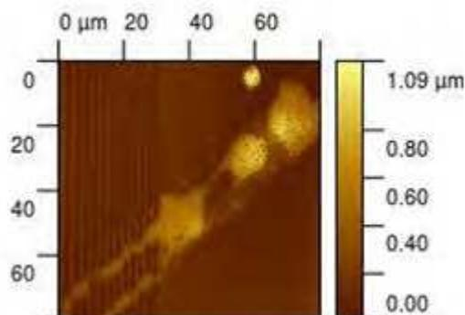
Figure 26: Topography scan of a noticeable structure, which was found at the Z calibration target at the end of the linear grid and used as a marker position to re-calibrate the linear stage.
