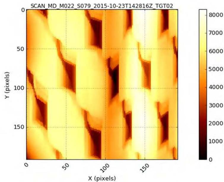
(b) topography image of the XY calibration target
