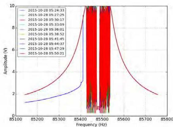
**2015-10-28 05:57:32 : Tip calibration of cantilever 10 after vibrating to clean**
