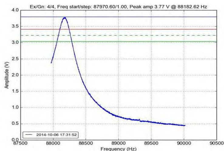
Figure 1: A frequency scan of cantilever 7, used for the majority of scans post -hibernation until the end of 2014. The blue line represents the peak amplitude, the red line the working point (driving amplitude/frequency) of 90% peak and the green line is the set-point of 80%. A re-tune threshold of 85% is given by the dashed line.
