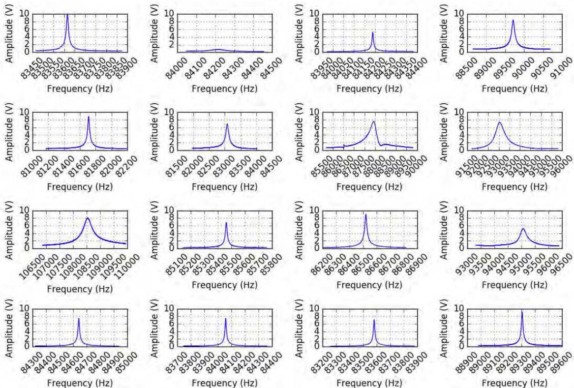
**2016-05-11 05:58:52 : Frequency tests of cantilever 2**
