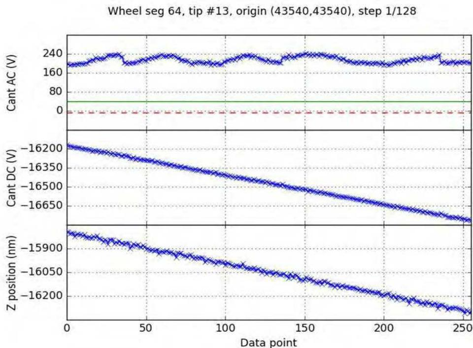
Figure 4: Raw (uncalibrated) control data for a line scan with tip 13 and a wrongly calculated set-point. Note that both the Z position and cantilever DC signals have minimum possible values of -16384, and hence this shows that the piezo was fully extended, resulting in maximum deflection of the cantilever.
