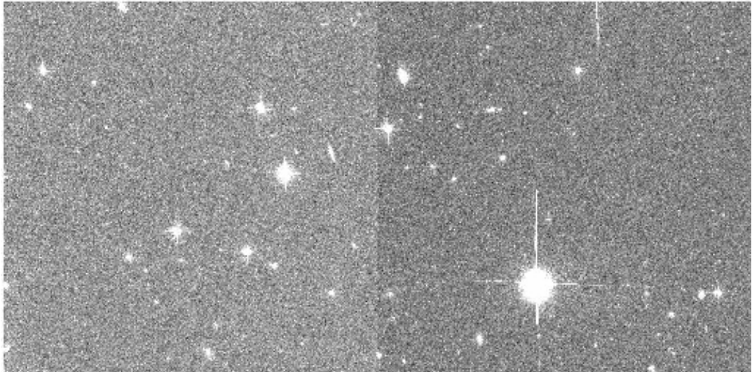
Figure 4.2: Calibrated WFC1 Image Showing the Quadrant-to-quadrant Jump
