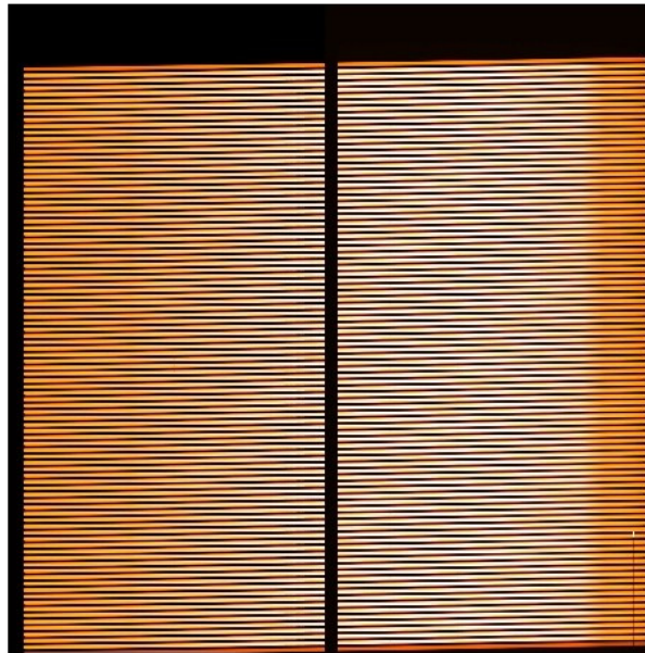
Figure 5.1.- Example image taken in fast readout mode, where many individual narrow-strip images are combined in a single detector readout.
