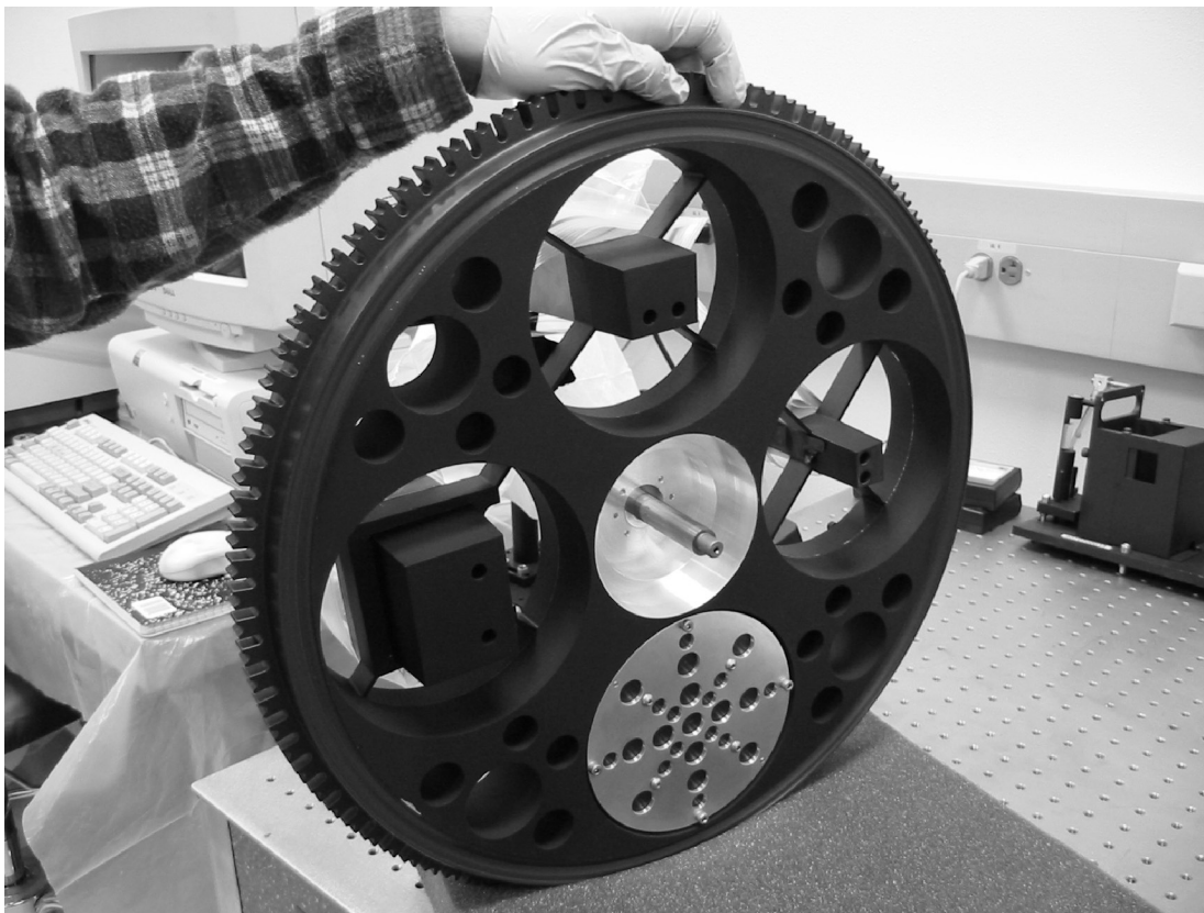
FIG. 5.—NIRI beam-splitter wheel during assembly, seen from the bearing surface ( bottom ). The pinhole mask ( bottom ) is used for instrument alignment and image quality checks. The large pick-off mirror for the f/6 camera is to the left; it effectively blocks all the light from continuing on into the OIWFS. The f/14 pick-off mirror ( top ) and f/32 pick-off mirror ( right ) allow the selection of a guide star very close to the science field.
