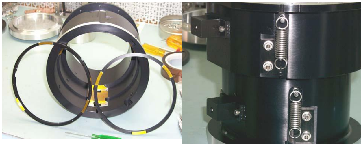
Figure 7. Camera barrel parts (left) and assembly (right). The left-hand picture shows the front half of a camera barrel showing hard points and two axial rings. The right-hand panel shows part of the assembled camera. Note the springs applying the axial forces and the housings for the radial spring plungers (on left side of barrel).
