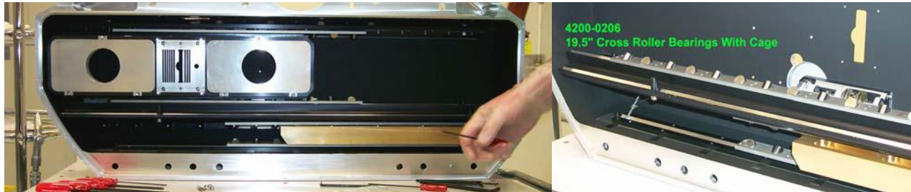
Figure 6. Front of slit slide, showing slit and IFU carrier (top, left) and counterweight (bottom, left). The drive is shown (right) with the slide removed. The picture shows dummy IFU units; see [11].
