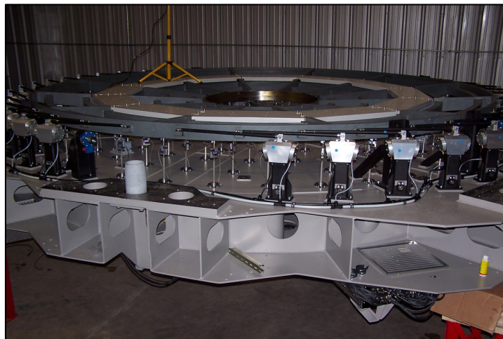
Figure 16. M1 Supports integration in M1 Cell
