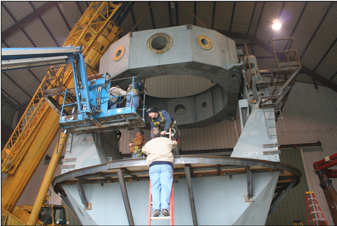
Figure 5. Mount trial assembly activities at GDST's fabrication facility in Wortham, TX
