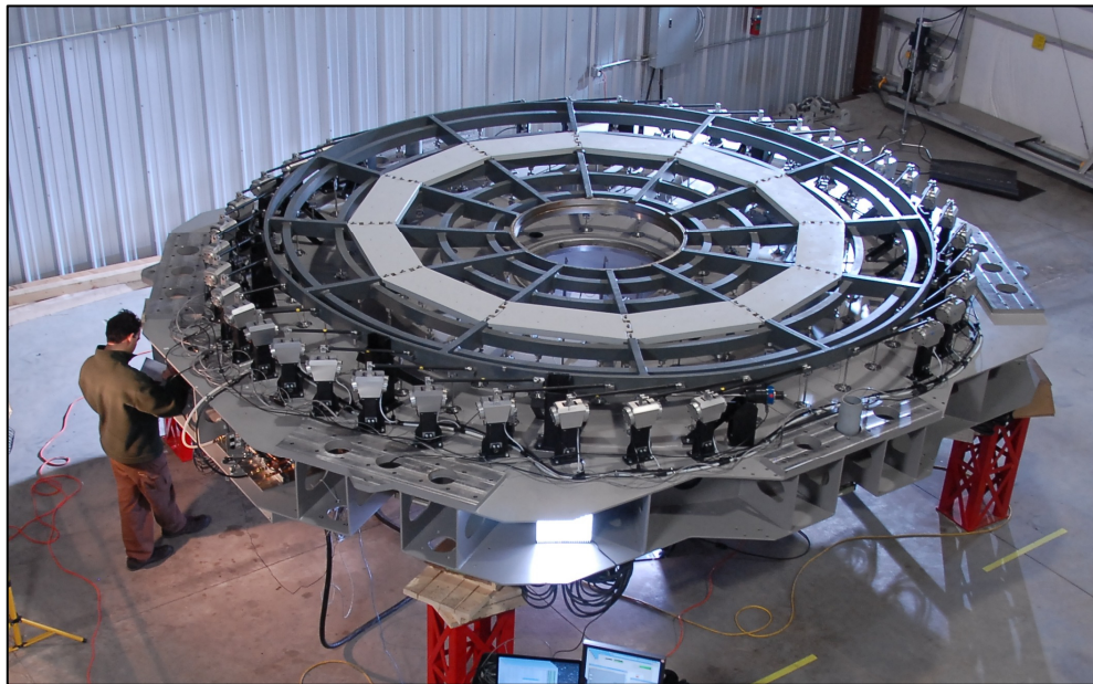
Figure 9. M1 support trial assembly at Pulliam Airport hangar in Flagstaff, AZ
