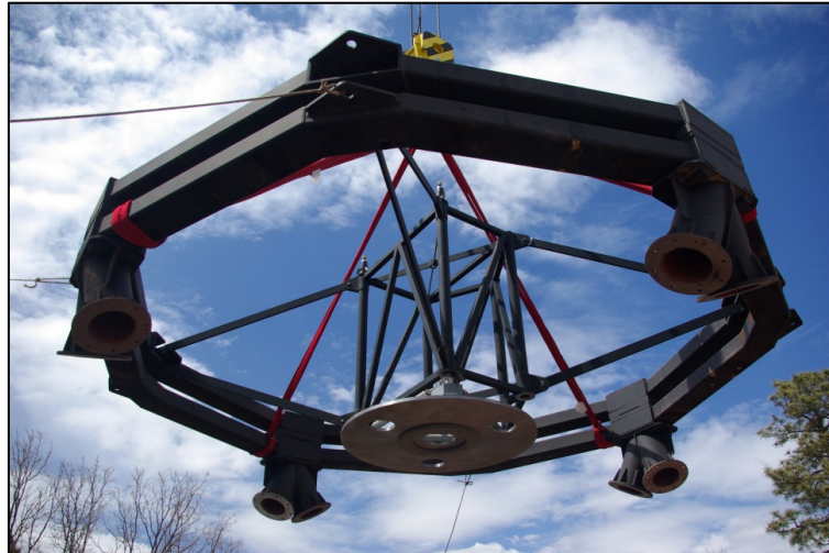
Figure 12. The M2 top end assembly with secondary mirror simulator
