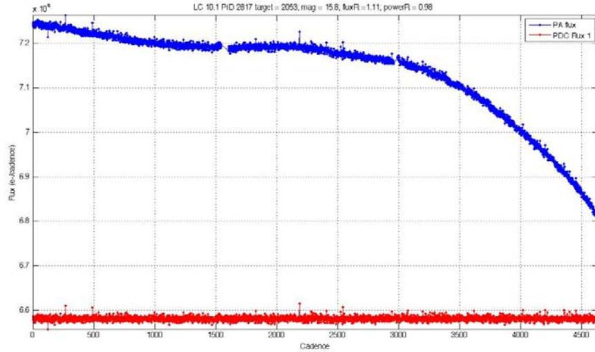
**Figure 7-7.** Q5 example of PDC removal of trends and discontinuities from the light curve of a quiet star with  $Kp = 15.8$ . The noise in the corrected light curve is only 11% greater than the noise expected from the calibrated pixels, a considerable improvement over the uncorrected light curve.
