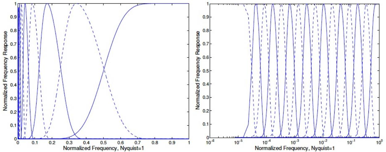
**Figure 8.4.** Frequency responses of the filters in the octave-band filter bank for a wavelet expansion corresponding to the signal flow graph in Figure 8.3 using Debauchies’s 12-tap filter. Left: frequency responses on a linear frequency scale. Right: frequency response on a logarithmic frequency scale, illustrating the “constant-Q” property of an octave-band wavelet analysis.
