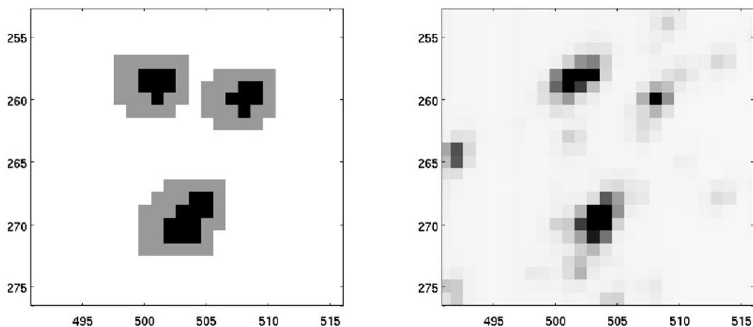
**Figure 4.4.** Left: Examples of the masks (grey) selected once the halo and undershoot column is added to the optimal aperture (black). Right: A flight image showing the targets captured by the masks on the left.
