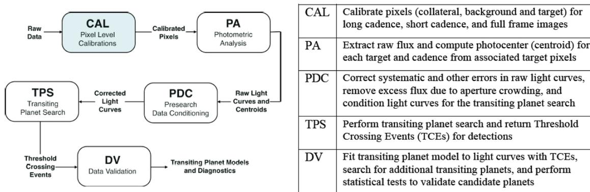
**Figure 5.1.** An overview of the science data flow in the SOC Pipeline is shown (left), along with a description of the primary functions of each component (right).
