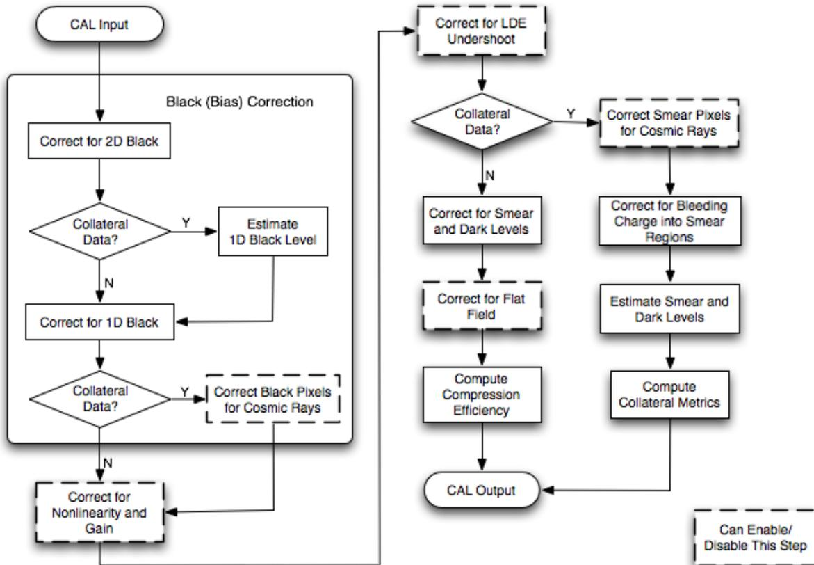
**Figure 5.4.** Data flow for calibrating collateral and photometric pixels. Dashed boxes indicate corrections that can be disabled in the Pipeline.
