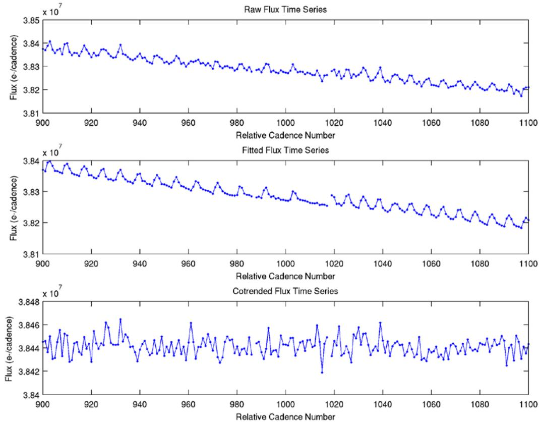
**Figure 7.6.** A 200-cadence segment of a raw flux time for a quiet long cadence target in Q1 is shown in the upper panel. Oscillation in the light curve is due to cycling of a reaction wheel heater outside the photometer. The least squares fit of the synchronized ancillary data to the raw flux is shown in the middle panel. The corresponding segment of the fit residual with mean level restored is shown in the lower panel.
