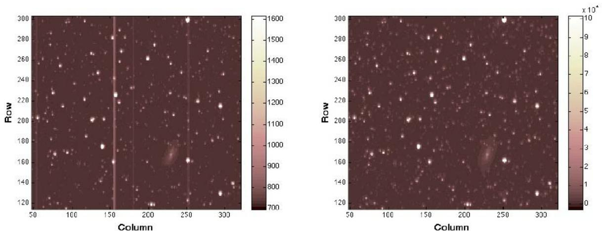
**Figure 5.8.** A portion of an uncalibrated FFI (in units of ADU/cadence, left) and the calibrated image (in photoelectrons per cadence, right) demonstrate the removal of smear from several columns.
