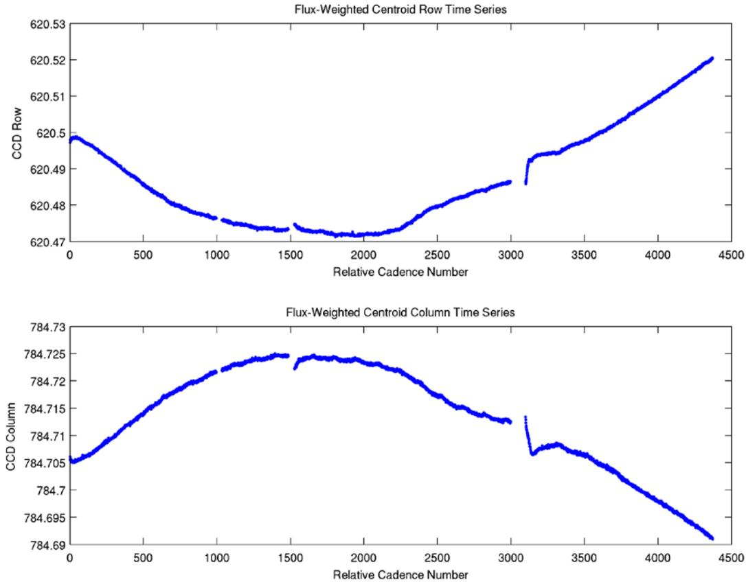
**Figure 6.6.** Flux-weighted centroid row and column time series for the PPA\_STELLAR target also shown in the left panel of Figure 6.4 and the upper panel of Figure 6.5. The data gaps are due to a loss of fine point anomaly and monthly data downlinks. Transients are due to focus changes that result from thermal changes in the photometer.
