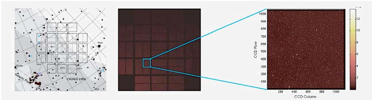
**Figure 5.2.** A celestial view of the *Kepler* focal plane (left), the first light image (middle), and a calibrated FFI from Q4 data (right, in units of  $10^6$  electrons/cadence) of module/output = 17/2 (channel 58) are shown.
