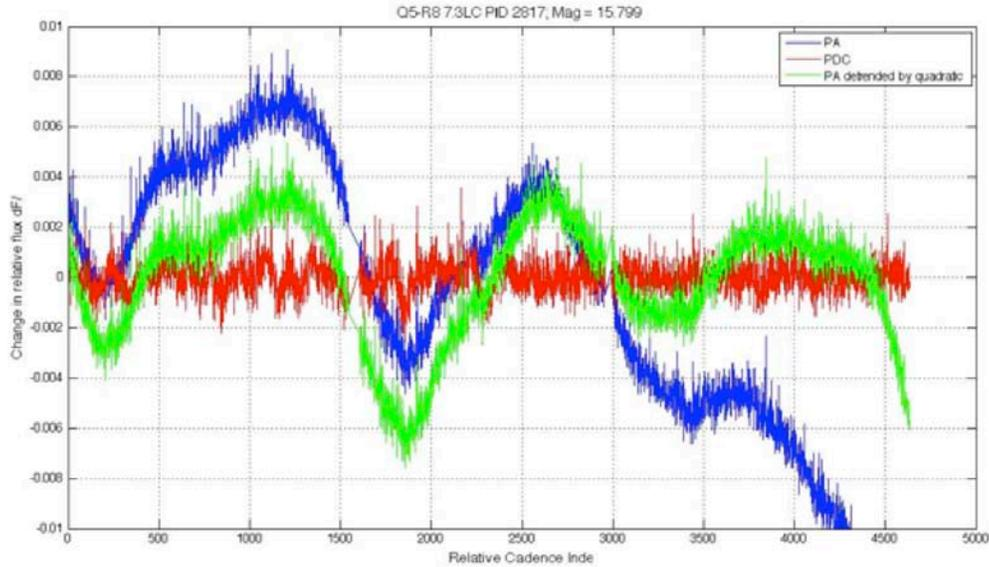
**Figure 7-13.** Q5 example of PDC removal of harmonic stellar variability. The amplitude of the variability with respect to a quadratic trend is  $\pm 0.54\%$ , just over the 0.50% threshold, before initial cotrending. Standard cotrending eliminated the variability but increased the noise, which PDC did not detect in this case. If PDC had detected the increase in noise, it would have retained the result of the harmonic-removed cotrending, and restored the harmonic content before export to MAST.
