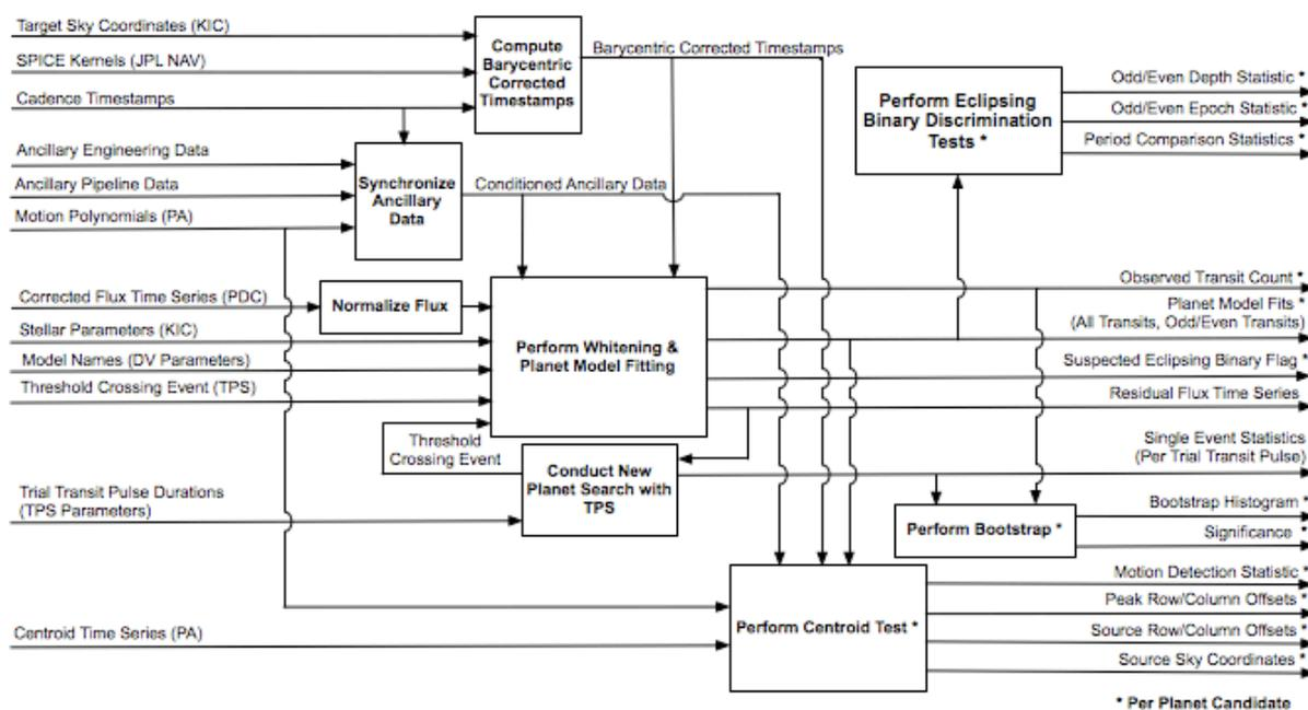
**Figure 9.1.** Data flow diagram for the Data Validation (DV) component of the *Kepler* SOC Pipeline. Processes performed for all planet candidates associated with each DV target and outputs produced for all planet candidates are shown with asterisks. Inputs are obtained from the *Kepler* DB and outputs are written to the *Kepler* DB.
