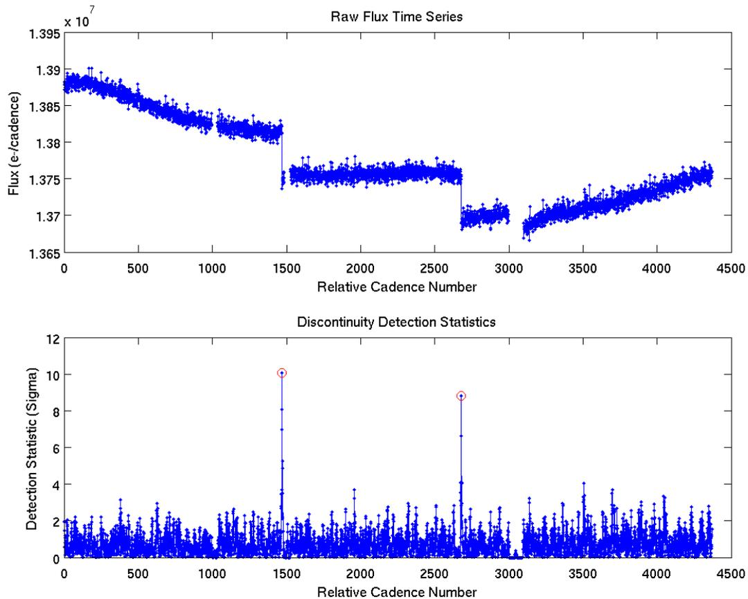
**Figure 7.3.** A raw flux time series with two random discontinuities is shown in the upper panel. The detection statistics formulated by correlating the second derivative of the time series with the discontinuity template are plotted in the lower panel. The detection statistics are circled for the cadence indices returned by the detector.
