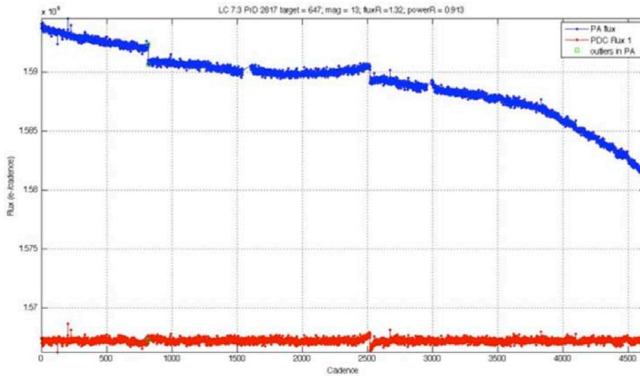
**Figure 7-10.** Q5 example of an unidentified and hence uncorrected target-specific discontinuity, located at cadences 800 and 2500.
