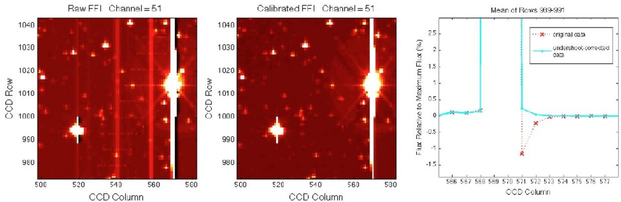
**Figure 5.7.** A close-up, stretched image of two saturated target stars that show pixel undershoot signatures resulting from bright-to-dark pixel transitions in the direction of the serial readout (left panel), and the calibrated image (middle). The mean of three pixel rows is shown for one target (right) with the undershoot response (the negative spike) along with the corrected pixel values.
