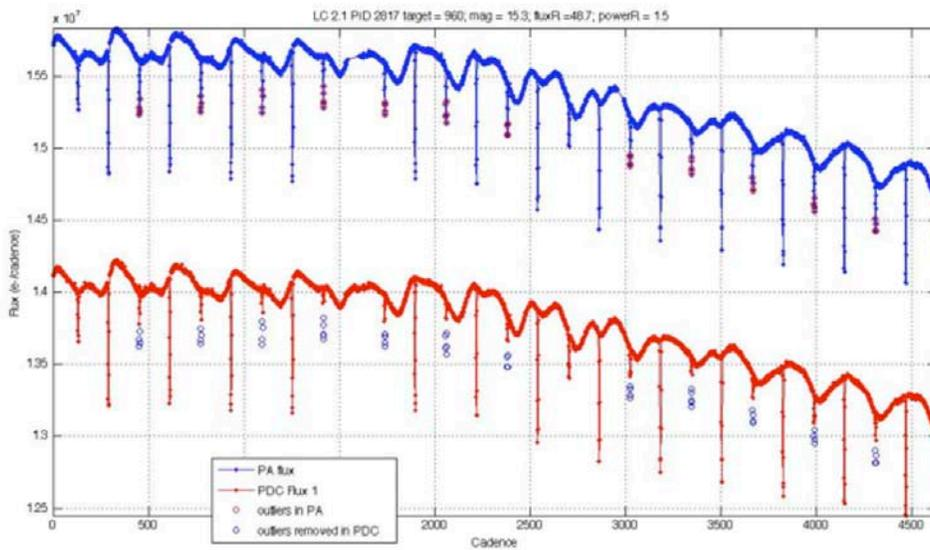
**Figure 7-12.** Q5 example of PDC mis-identifying an eclipse as an outlier.
