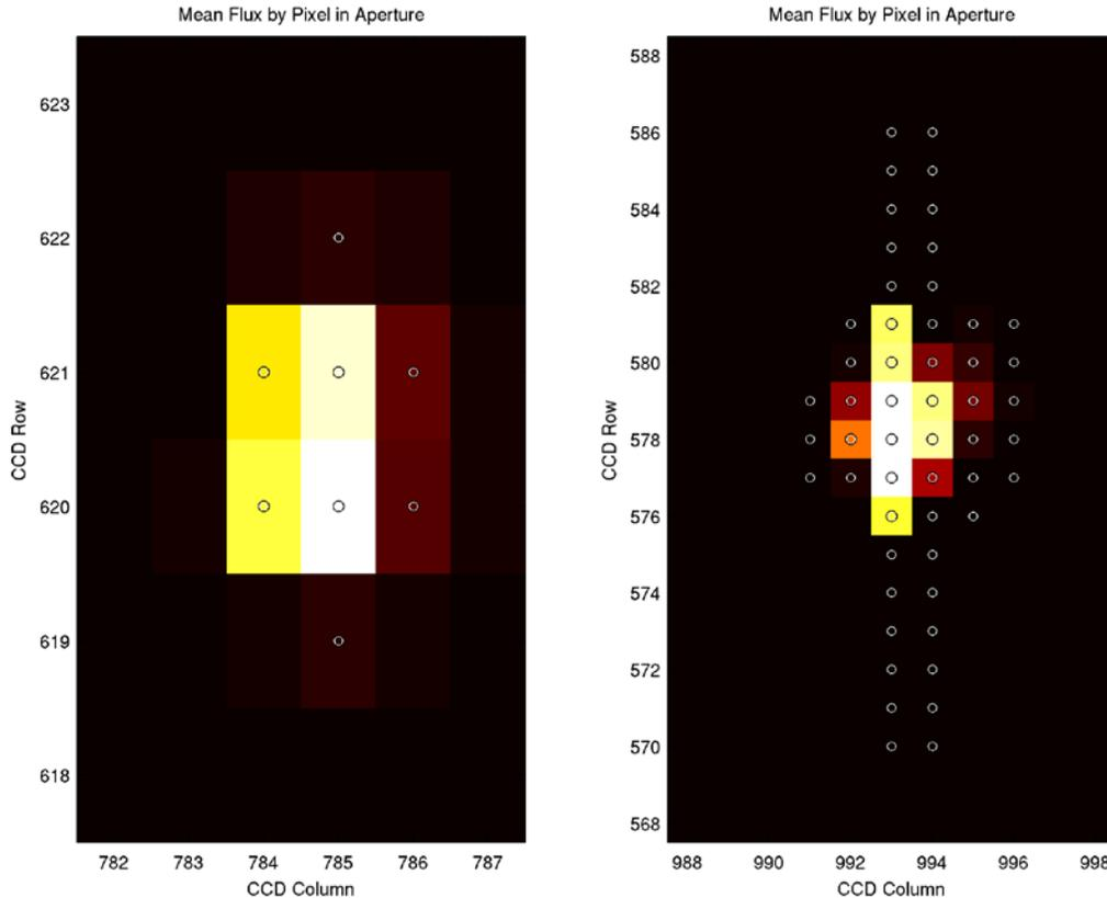
**Figure 6.4.** Mean flux levels for pixels in two target apertures. The PPA\_STELLAR target on the left is 13th magnitude. The saturated target on the right is 10th magnitude. Pixels in the optimal aperture for each target are indicated with circles. The color map range for the saturated target is nearly ten times larger than that of the PPA\_STELLAR target.
