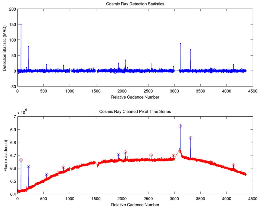
**Figure 6.3.** Cosmic ray detection statistics for a single Q3 pixel time series are shown in the upper panel. The target pixel time series before and after cleaning are shown in the lower panel. Cosmic ray events in the original pixel time series are circled. Flux transients following the monthly downlinks near cadences 1500 and 3000 are thermally induced.
