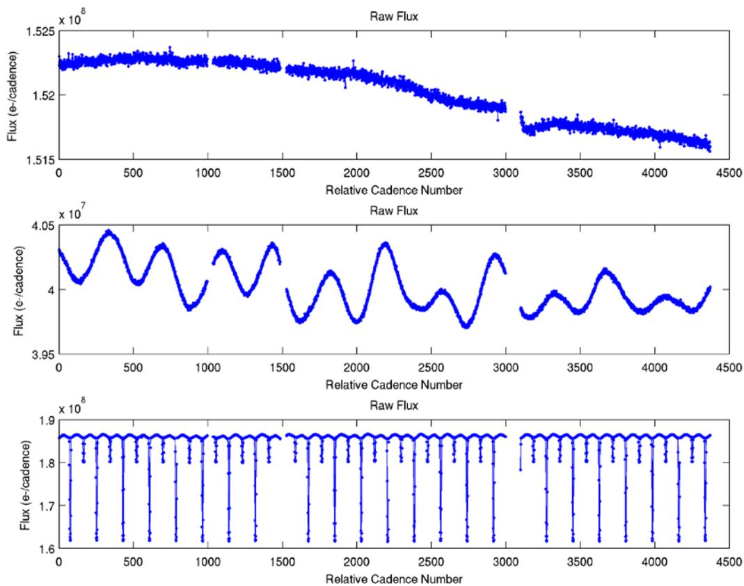
**Figure 6.5.** Raw flux light curves for representative targets computed by SAP in Q3 for module output 7.3. A quiet PPA\_STELLAR target is shown in the upper panel, a variable target in the middle panel, and an eclipsing binary in the lower panel.
