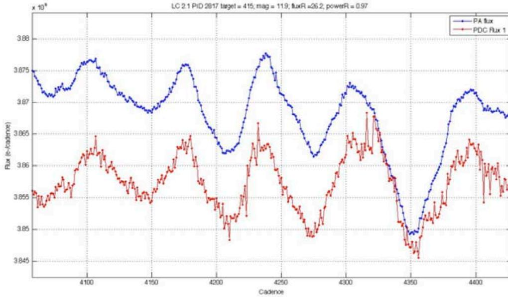
**Figure 7-11.** Q5 example of PDC adding short-period noise to a light curve, which it did not identify as a bad cotrend.
