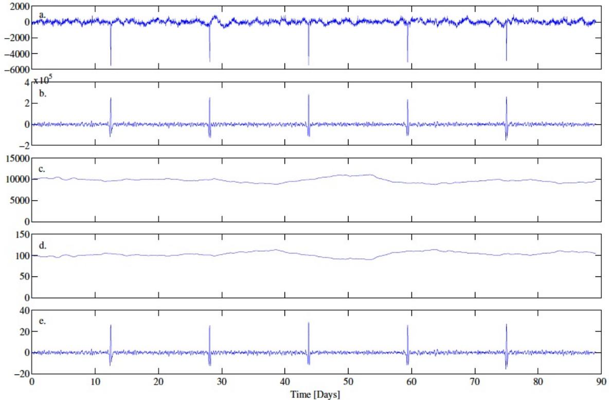
**Figure 8.5.** Calculation of CDDP for one target star. (a) Normalized target flux in parts per million (ppm). (b) Correlation time series  $N(n)$  from Eq. 8-7. (c) Normalization time series  $D(n)$  from Eq. 8-7. (d) Three-hour CDDP time series. (e) Single-event statistic time series,  $T(n)$ . In all cases, the trial transit pulse,  $s(n)$ , is a square pulse of unit depth and three-hour duration.
