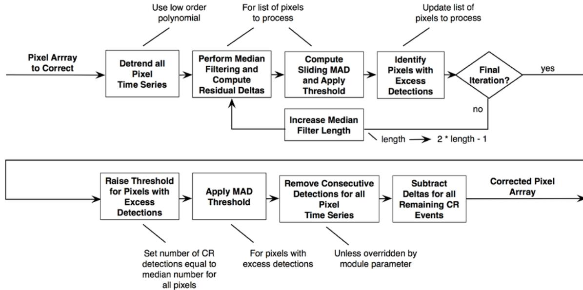
**Figure 6.2.** Flow chart for the cosmic ray cleaning algorithm. The loop in the upper path is executed twice in the current PA release.
