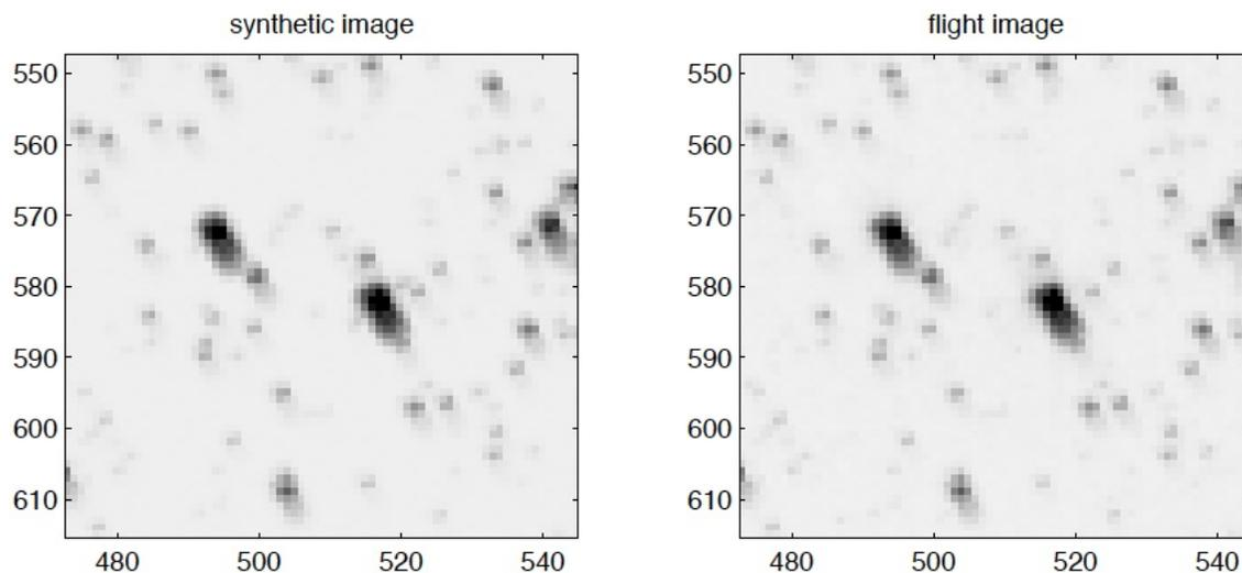
**Figure 4.1.** A comparison of a synthetic image (left) and a flight image of the same region of the sky, near the edge of the *Kepler* FOV where the PRF is large. For purposes of comparison with the sky image, the synthetic image is computed for a short time interval so it is not smeared by DVA.
