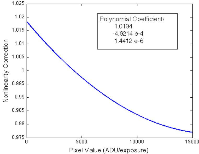
**Figure 5.6.** The nonlinearity correction, shown for a sample CCD channel, is the fractional deviation from the linear electrons-to-ADU transfer function at each pixel value.
