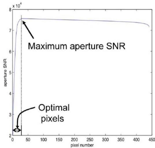
**Figure 4.2.** The aperture SNR curve built up as pixels are added in order of decreasing pixel SNR. The optimal set of pixels is the set at the maximum of this curve.
