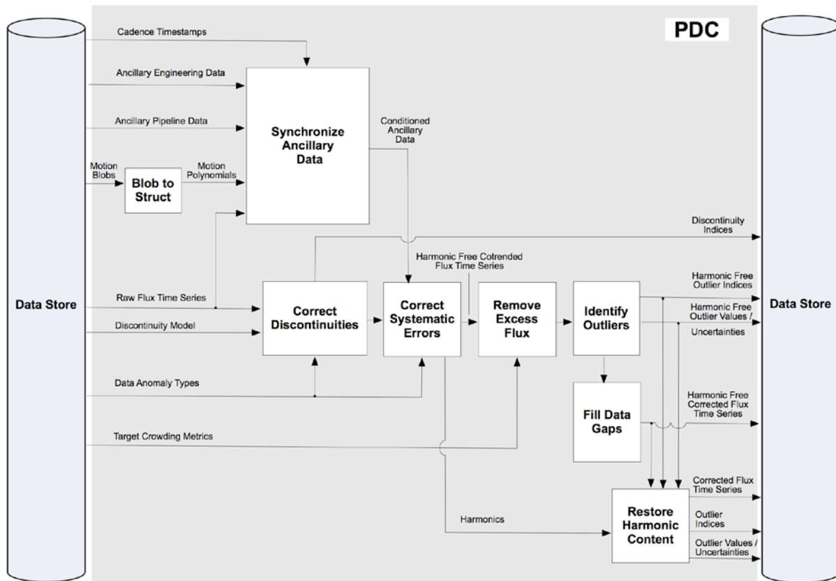
**Figure 7.1.** Data flow diagram for the Presearch Data Conditioning Pipeline module. Inputs are shown at the left and outputs are shown at the right. Inputs are obtained from the Data Store and outputs are written to the Data Store
