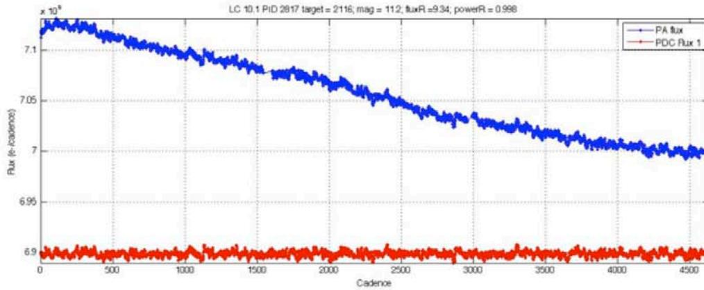
**Figure 7-9.** Q5 example of PDC correction of a non-harmonically variable star. The RMS of the corrected (red) curve is about 9x the noise calculated from the read and shot noise in the calibrated pixels, and is believed to be almost entirely due to intrinsic stellar variability.
