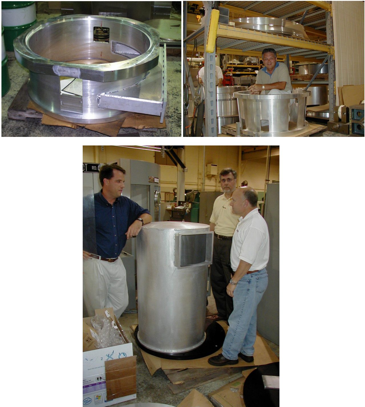
Figure 8 – FLAMINGOS-2 major dewar mechanical components: (Top left) MOS dewar vacuum jacket; (Top Right) Mechanical interface between the MOS and main dewars with the project manager Roger Julian for scale; (Bottom) main dewar vacuum jacket mounted on the bulkhead plate and main dewar lid. For scale, UF mechanical engineer Jeff Julian (left) is 190cm tall.
