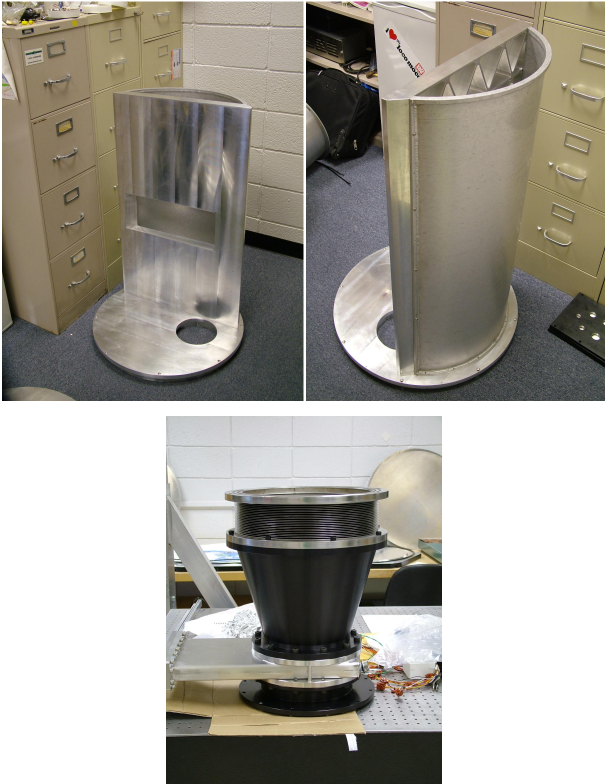
Figure 9 – (Top left/right) FLAMINGOS-2 cryogenic optical bench assembly. (Bottom) Vacuum interface and gate valve between the MOS and main dewars.
