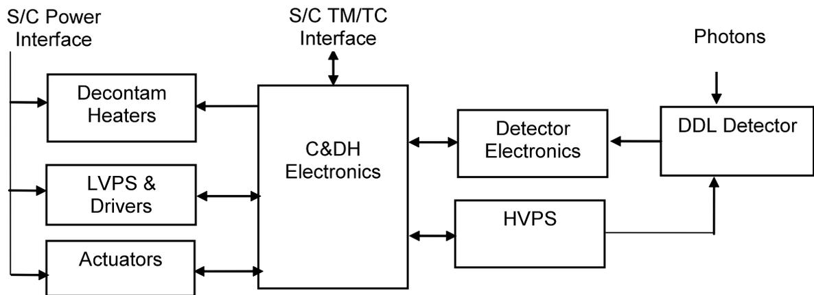
Figure 1.3-4. Block diagram of Alice.
