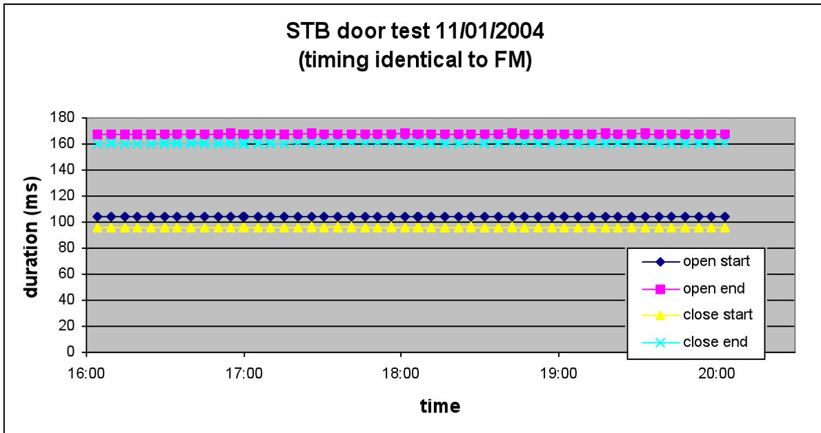
Below we show the plot of all aperture door performance tests that have run since launch through passive checkout PC3:
