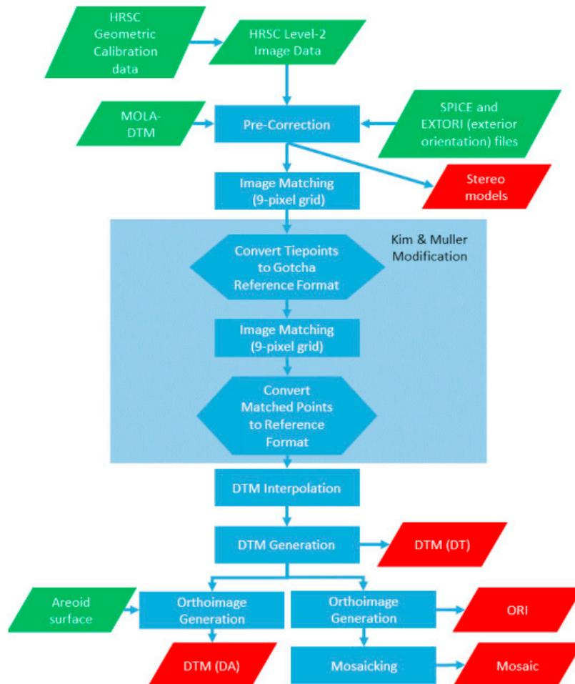
Figure 1 Schematic of modified DTM production algorithm based on DLR-VICAR (Kim and Muller, 2009; Putri, et al., 2019)
