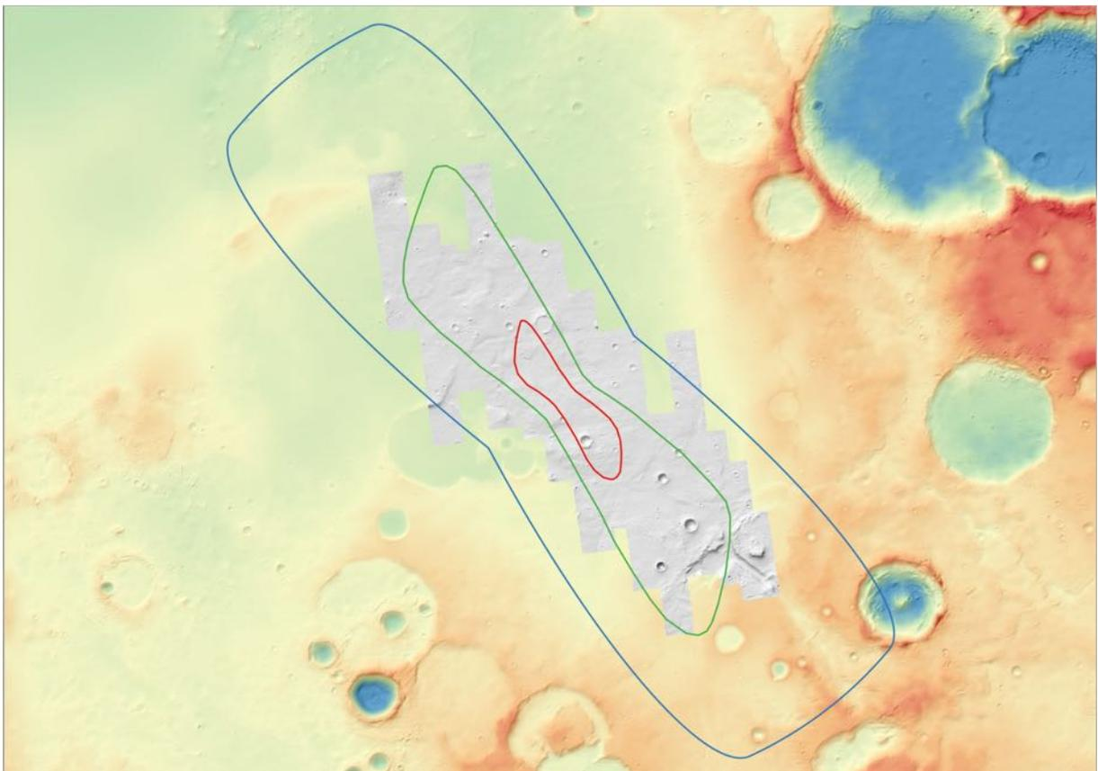
Figure 7. HiRISE MADNet 1.0 0.5m DTM superimposed on MADNet 1.0 CTX 12m DTM superimposed on MADNet 1.0 HRSC 25m DTM all using the same colour hill-shaded parameters with reduced colour for the HiRISE showing the 1-sigma (in red) and 3-sigma (in green) landing ellipse as of the date of this document and the geological mapping area (in blue).
