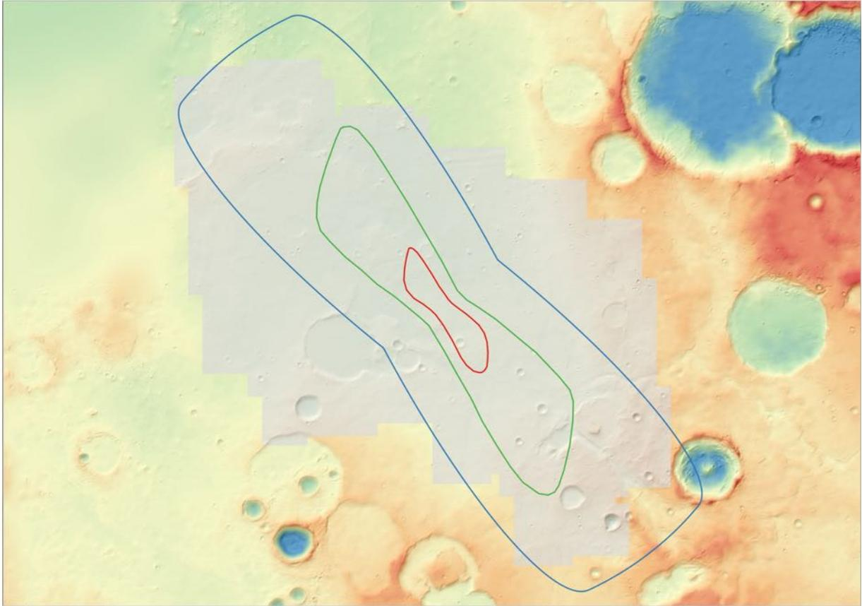
*Figure 6. Colourised and hill-shaded CTX MADNet 12m DTM superimposed on top of HRSC MADNet 1.0 25m DTM showing the 1-sigma (in red) and 3-sigma (in green) landing ellipse as of the date of this document and the geological mapping area (in blue).*
