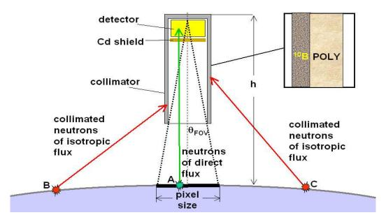
Figure 2-5 Collimation principle diagram
