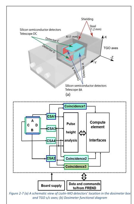
measured in each pair of parallel detectors in coincidence mode are recorded separately and used to obtain the LET spectrum in that direction
