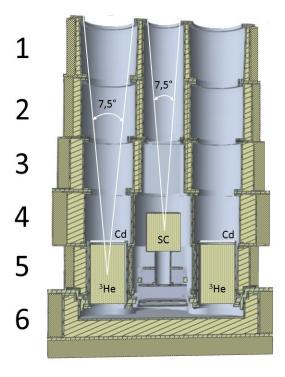
Figure 2-6 Collimator cross-section
