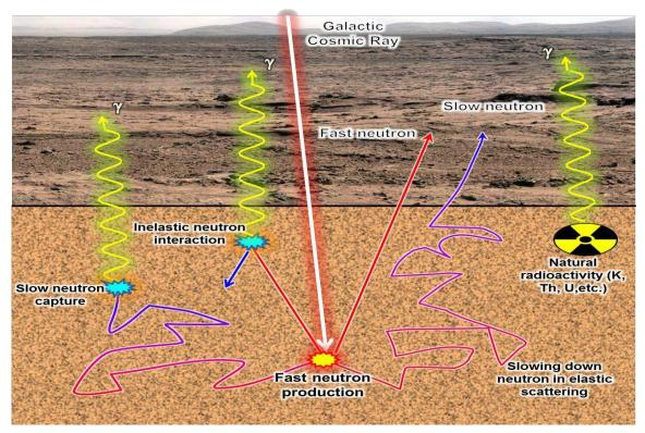
Figure 2-1 FREND measurement physical principle
