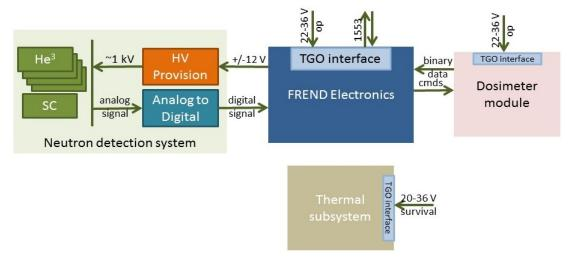
Figure 2-8 FREND Digital Electronics block diagram
