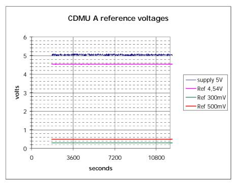
Fig 4.9: CDMU A Voltages (5V is not stabilized)
