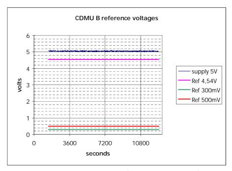
Fig 4.10 : CDMU B Voltages (5V is not stabilized)
