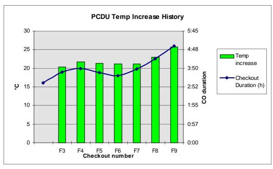
Fig 4.13: initial PCDU temperature evolution wrt checkout duration
