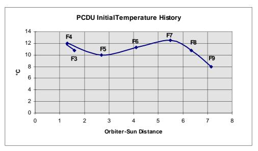
Fig 4.12: initial PCDU temperature evolution
