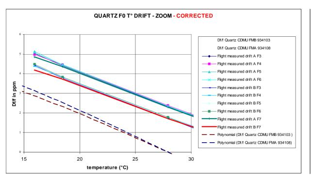
Fig 4.11 : Computed CDMU A & B Data clock drift wrt CASSINI RTI
