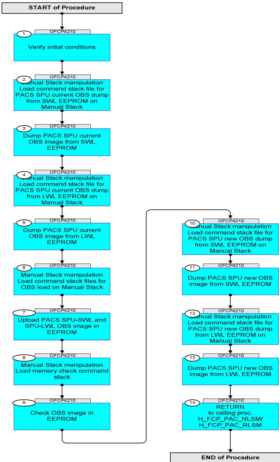
Load PACS SPU OBS in instrument INIT mode
