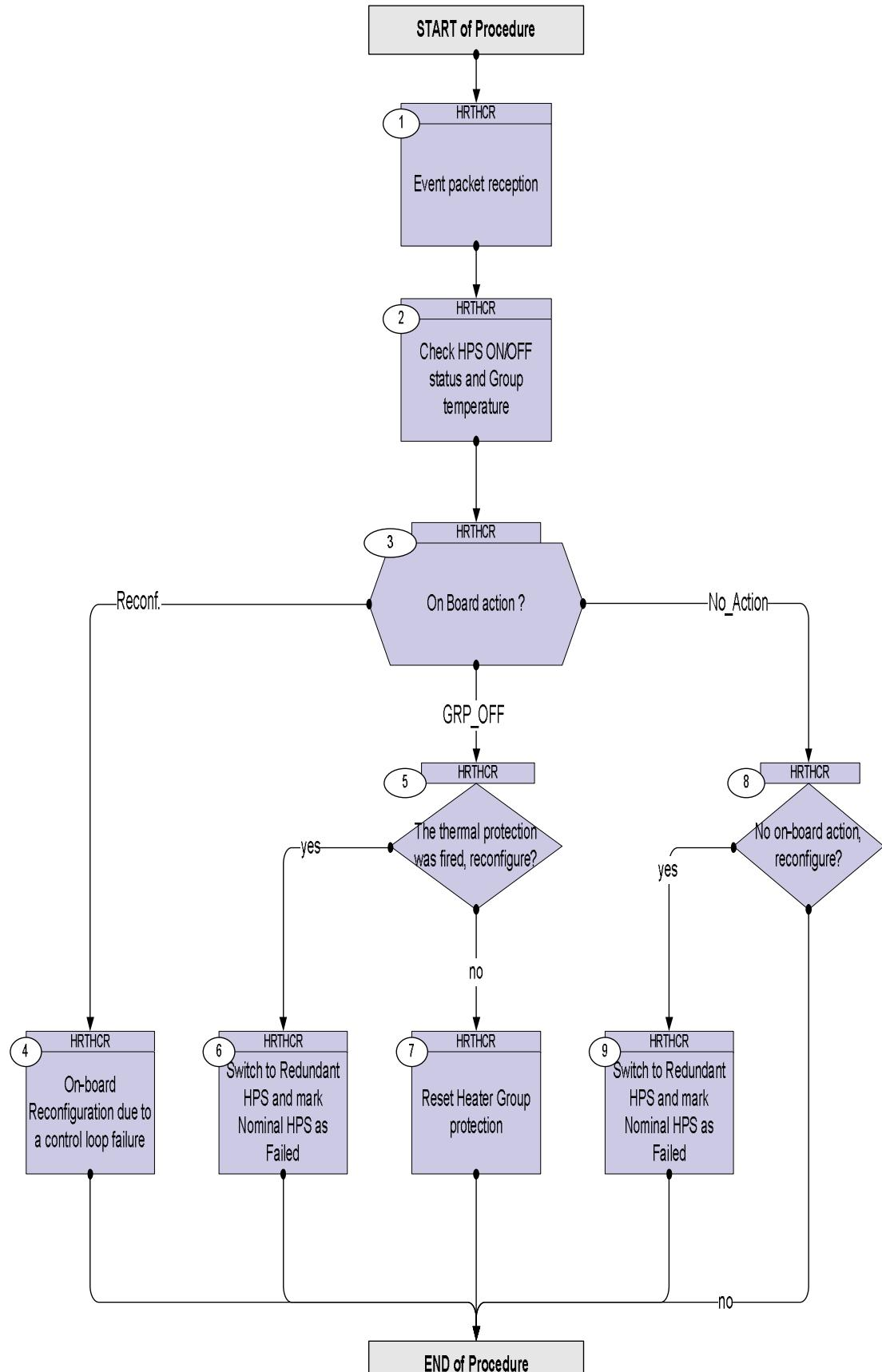
Configuration check after HCS high dissipation detection
