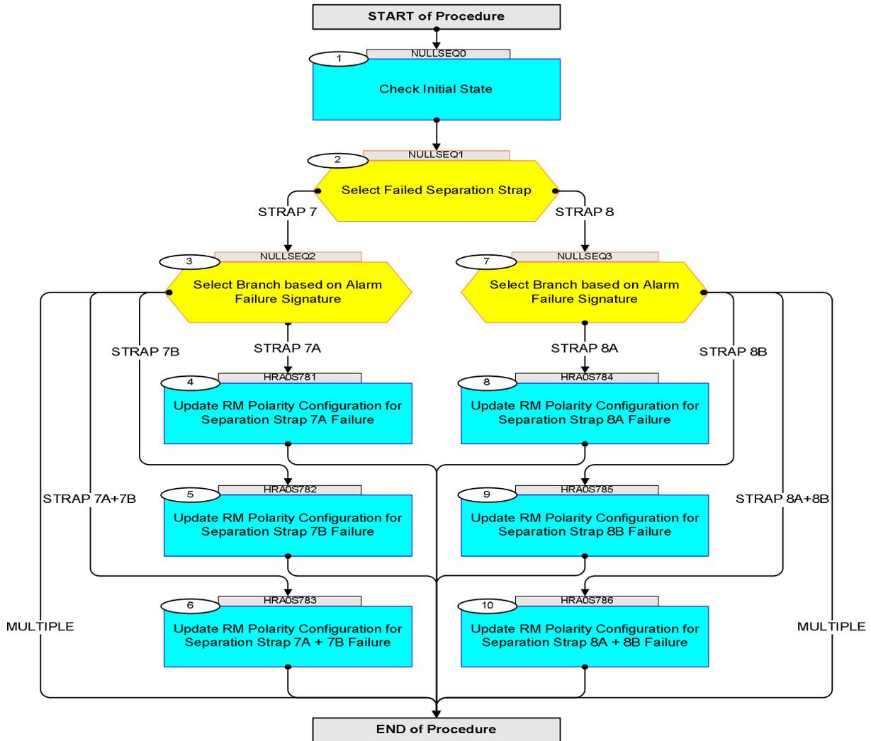
Recovery from Separation Straps 7 or 8 Failure
