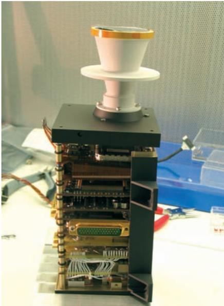
Fig. 4. VMC with one side of the housing removed, showing the CRE, DPU and POC boards (top to bottom).
