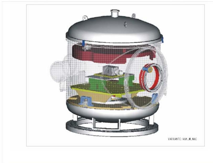
Figure 4.9 VMC mounted in TV chamber during calibration
