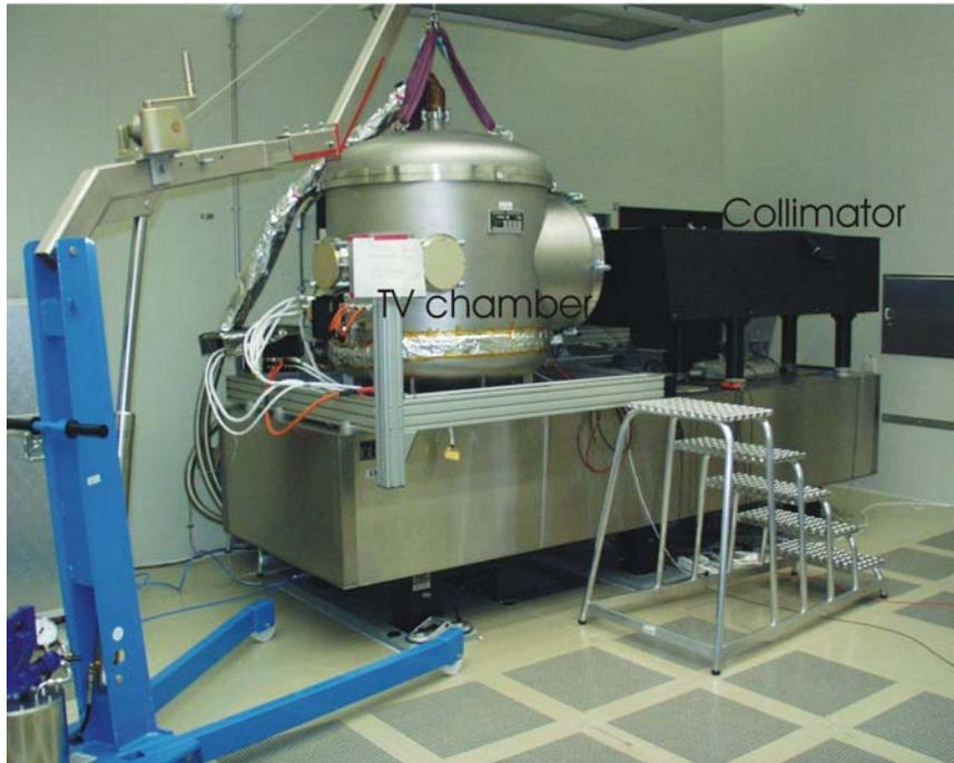
**Figure 4.5** Calibration Set-up (side view) used for geometrical and spectral calibration @ MPS
