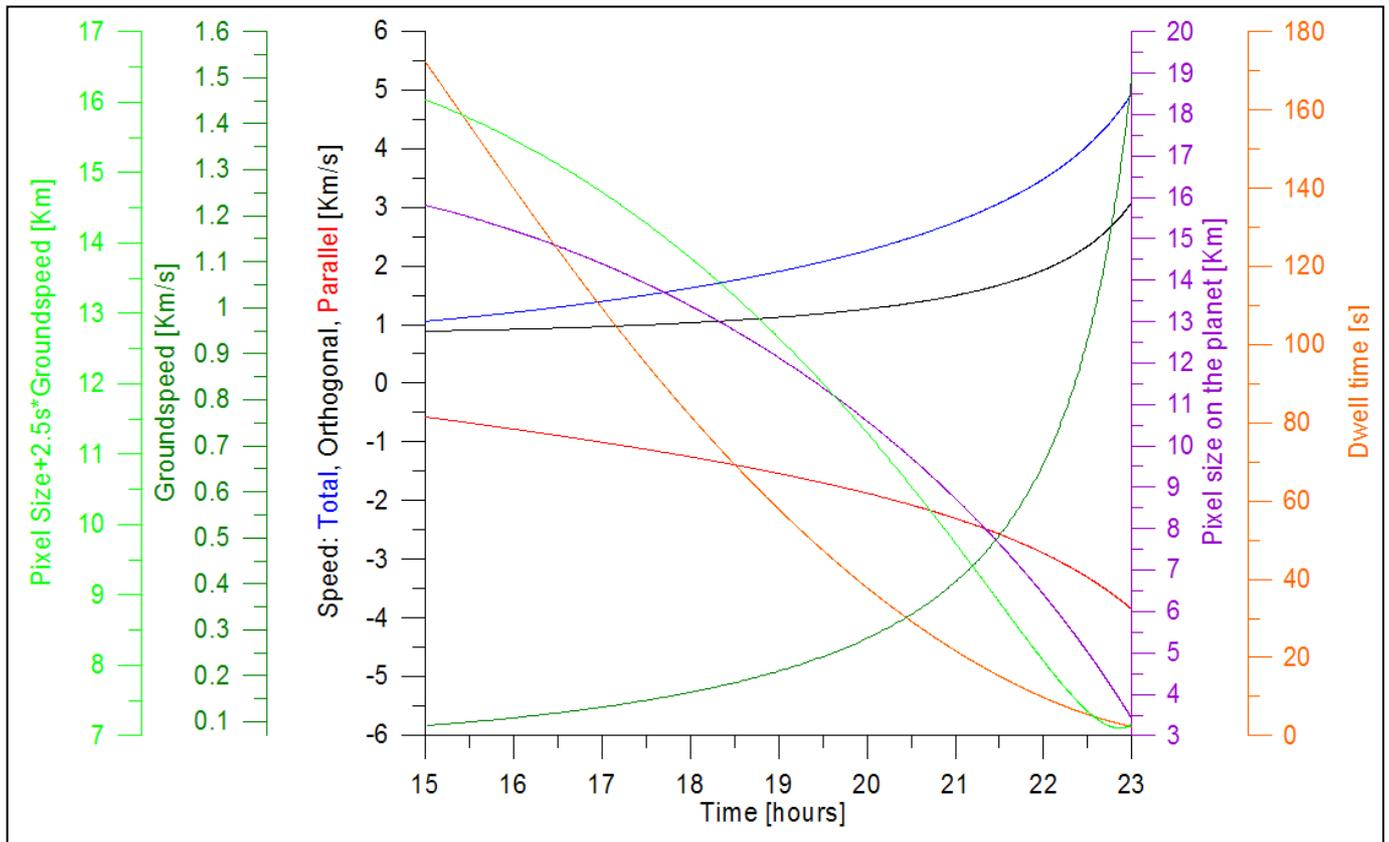
Fig. 4.3.11.2-1: Main observation parameters for VIRTIS in the science case 2
