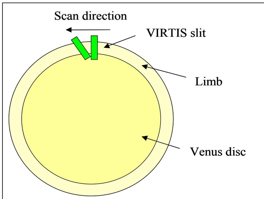
Fig. 4.3.11.7-4: Geometry of the VIRTIS slit wrt Venus limb and disc
