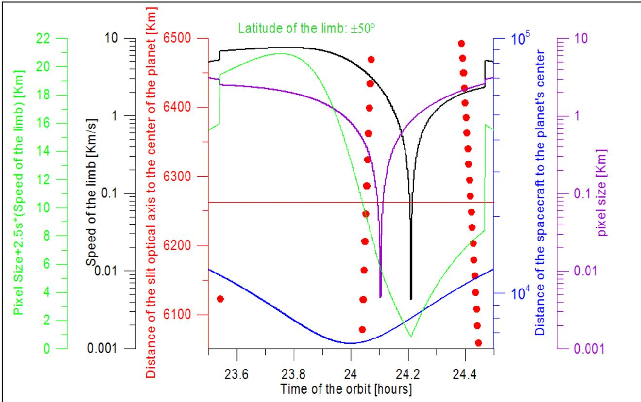
Fig. 4.3.11.7-3: Main observation parameters for VIRTIS in the general science case 7, limb @  $\pm 50^\circ$
