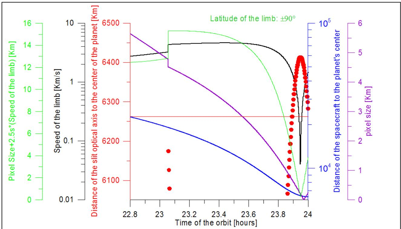
Fig. 4.3.11.7-2: Main observation parameters for VIRTIS in the general science case 7, limb @ +90°
