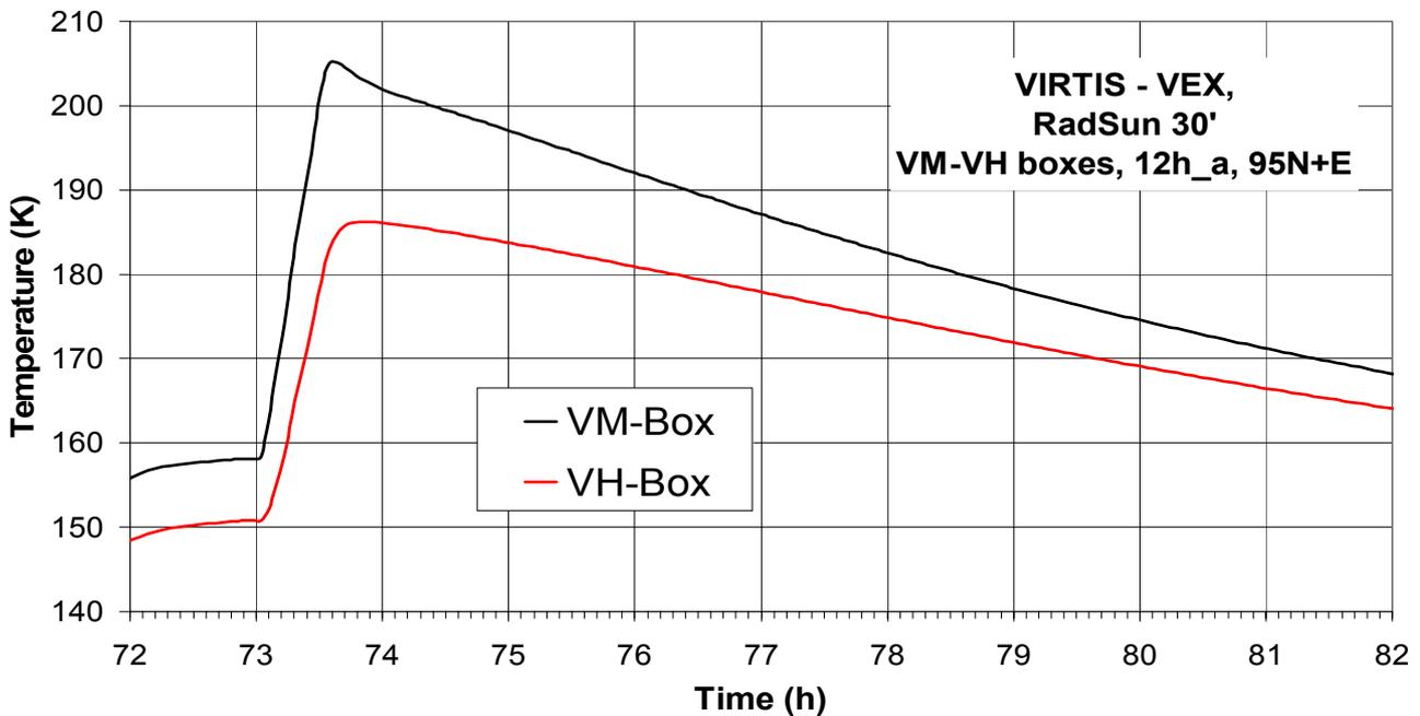
Figure 4.3.1.7-3 : Average temperature of the cold boxes during deicing (sizing case at 12h). The exposure of radiator starts at 73h time. The temperature of the cold boxes is reasonably safe and well within the non-operational range to support safely the deicing procedure.
