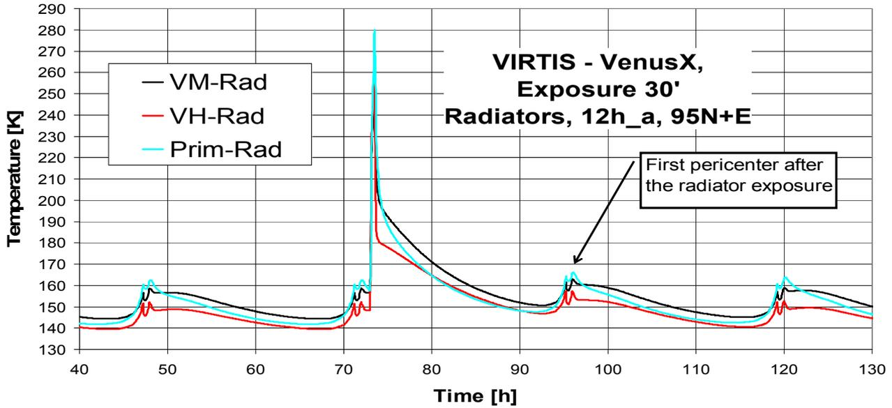
Figure 4.3.1.7-2 : Average temperature of the radiators for several orbits, sizing case at 12h. The exposure of radiator starts at 73h time. In the successive orbit after the deicing, the thermal regime is close to be reestablished. A case 3 observation, for example, would be possible.
