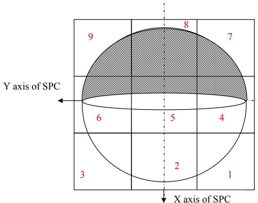
Figure 4.3.11.3-2 : SPC repointing strategy with numbered sequence for VIRTIS in the science case 3. The dark side of Venus is on top and the radiator (-X) is pointed to the shadow. The ellipse about the center is due to the fact that the ground track at the apocenter is at about 80°S and not at 90°S.
