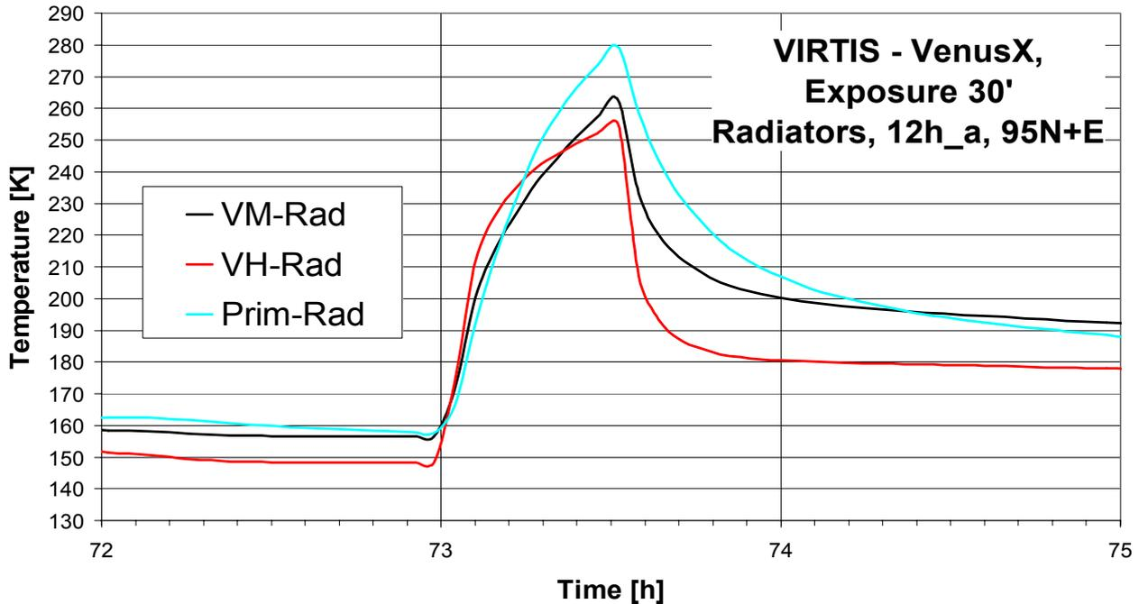
**Figure 4.3.1.7-1 : Average temperature vs time on the three pieces of the VIRTIS radiator. The configuration is for sizing case (case 1, 12h) and exposure time is 30' starting 1 hour after pericenter. A temperature of the order of 250K as for Rosetta is considered sufficient for deicing of radiator.**
