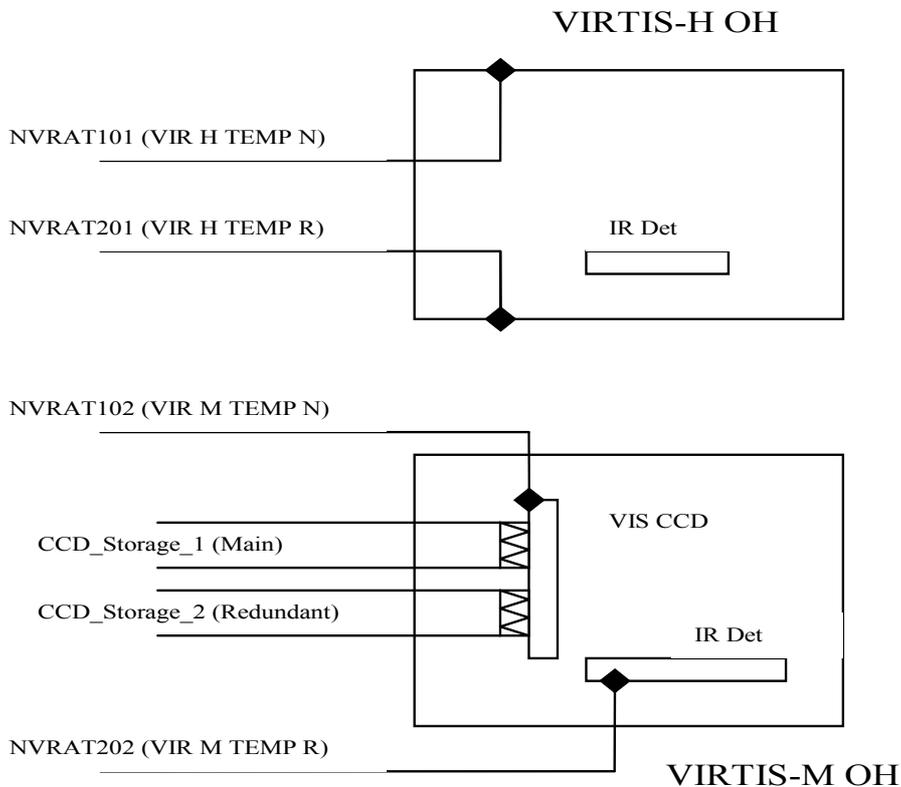
Figure 2.4.4-1 : VIRTIS CCD\_storage heaters & S/C powered thermistors location
