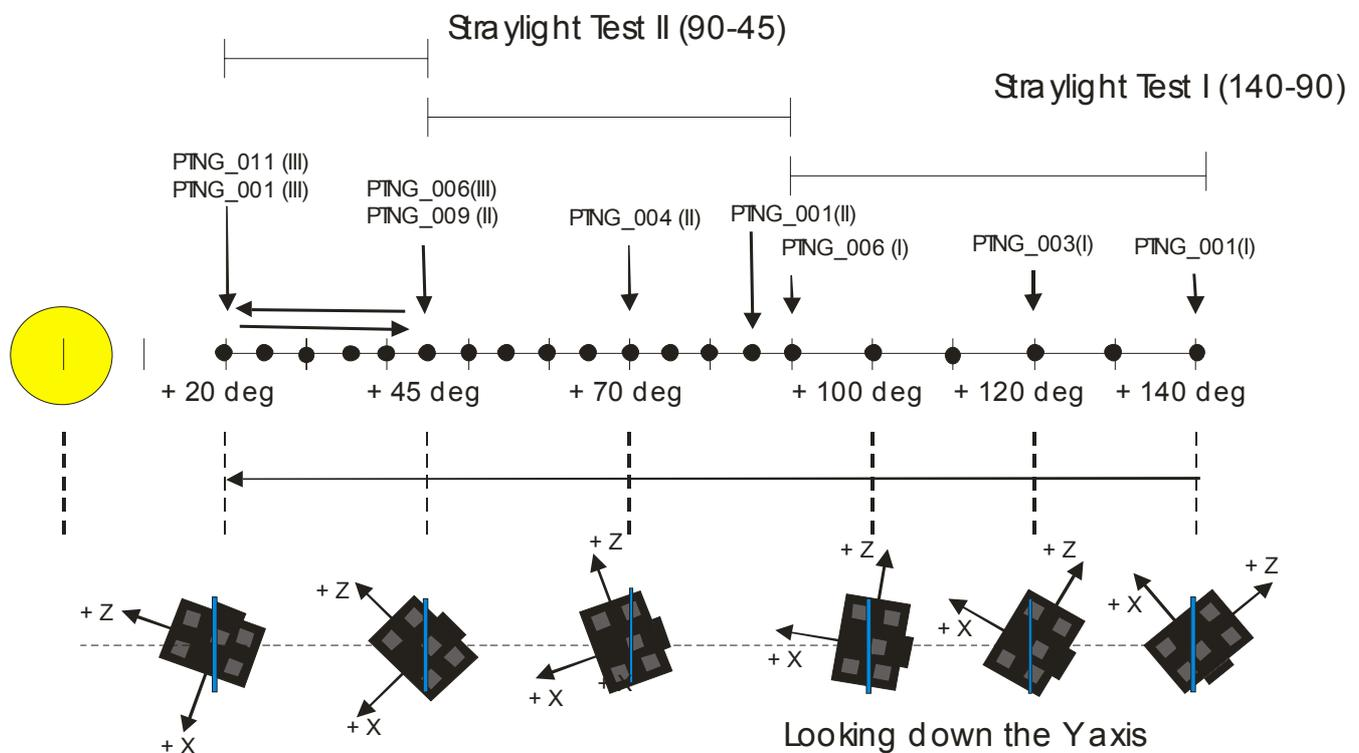
**Figure 4.3.1.2-1 : possible starting point of a procedure for straylight measurements. We propose to apply the procedure also for different angles around X axis (detail TBD, still under discussion with VSOC)**
