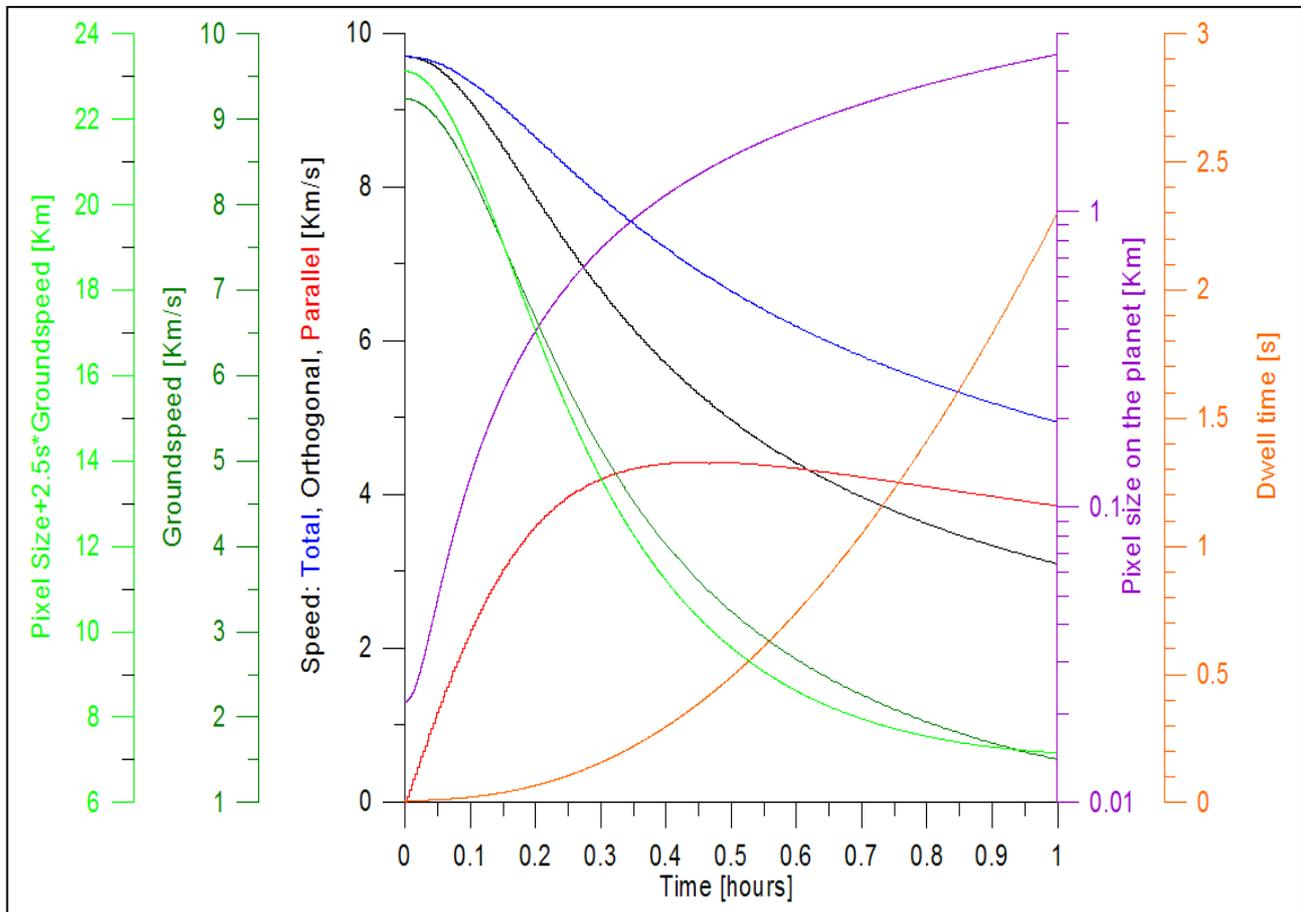
Fig. 4.3.11.1-1: Main observation parameters for VIRTIS in the science case 1
