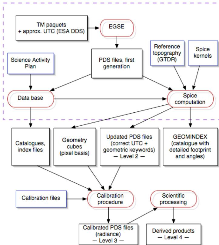
Figure 1: VIRTIS VEx processing pipe-line
