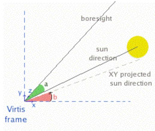
Figure 4: Sun direction in the instrument frame
