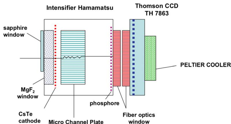
**Figure 2.** Sketch of the SPICAM UV detector. It combines a UV image intensifier from Hamamatsu, transforming each UV photon at the entrance into a pulse of green light generated by the phosphor. Then the image is conveyed through two blocks of fiber optics, one included in the Hamamatsu detector, the other one being attached to the Thomson CCD (by Bill Sandel at LPL). The sapphire window is placed to block second order of grating diffraction.
