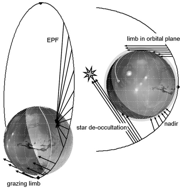
**Figure 6.** Sketch of various modes of observation of SPICAM. In all cases, the black line indicates the LOS of SPICAM to the target. Except for the usual nadir orientation and the special case of EPF (Emission Phase Function), the spacecraft is drifting along the orbit, keeping a constant celestial orientation, which allows us to scan across the target (limb) or to perform an occultation of star or Sun.
