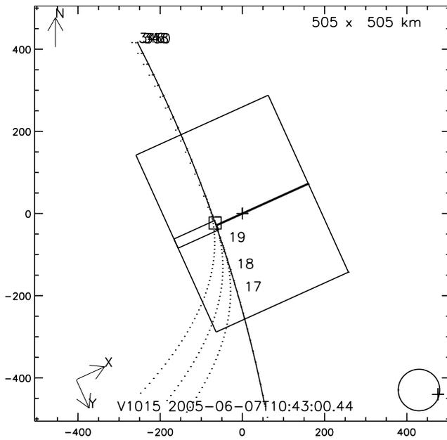
**Figure 15a.** Geometry of a special limb observation to study stray light generated in the spectrometer. The limb of the planet was Sun illuminated and is represented as a curved solid line. The full rectangle represents the whole CCD FOV, with the contours of the slit in the middle. The slit was placed perpendicular to the limb of the planet, with the large part of the slit on the bright part of the limb.
