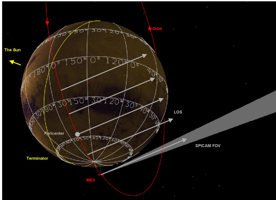
**Figure 7.** Geometry of grazing limb observations, which allows us to maximize the time spent to observe the limb. The spacecraft is oriented with the +Z axis (SPICAM LOS) fixed inertially, scanning the limb twice. In this case, the LOS was perpendicular to the velocity vector at pericenter, for an optimum vertical resolution at the limb.
