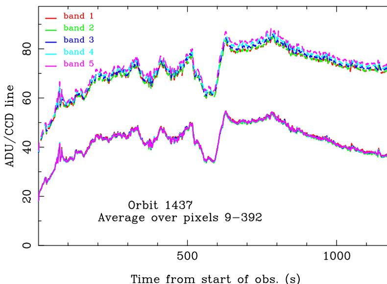
**Figure 18.** The upper curves (dashed lines) are raw data for the five bands at orbit 1437 across Olympus Mons (intensities integrated over the whole spectrum). They are slightly different. The lower curves (solid lines) are the same data after subtraction of offset, Dark Charge, and internal stray light. After the correction, the five bands have exactly the same intensity, which was not the case before the correction.
