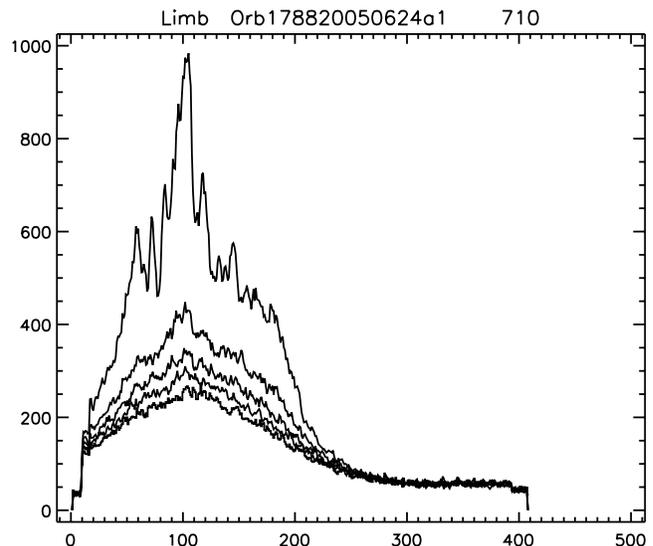
**Figure 15b.** During the one second exposure corresponding to the geometry of Figure 15a, the 5 spectra recorded at 5 points of the narrow slit are represented. The nearest point to the limb sees a normal solar spectrum (scattered by dust at the limb), while the others, further away, see only stray light generated through the large portion of the slit. A series of such measurements allowed us to characterize the stray light and correct for it.
