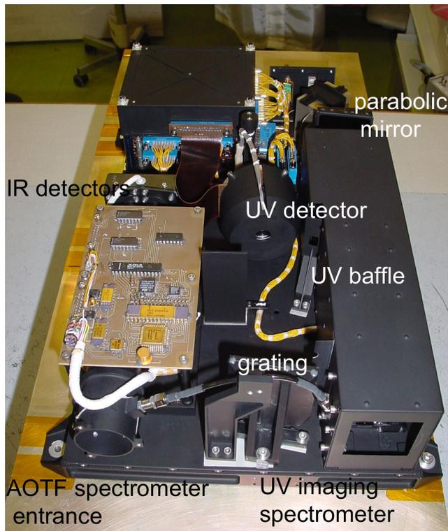
**Figure 3.** SPICAM sensor unit with the two UV and IR spectrometers, side by side. The entrance of the UV spectrometer baffle is on the right ( $5 \times 5$  cm, giving the scale), while the entrance of the AOTF IR spectrometer is on the left side.
