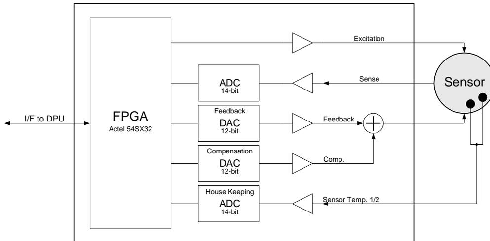
Figure 5. Block diagram of sensor electronics
