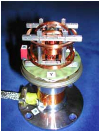
Figure 4. Photo of the magnetometer sensor
