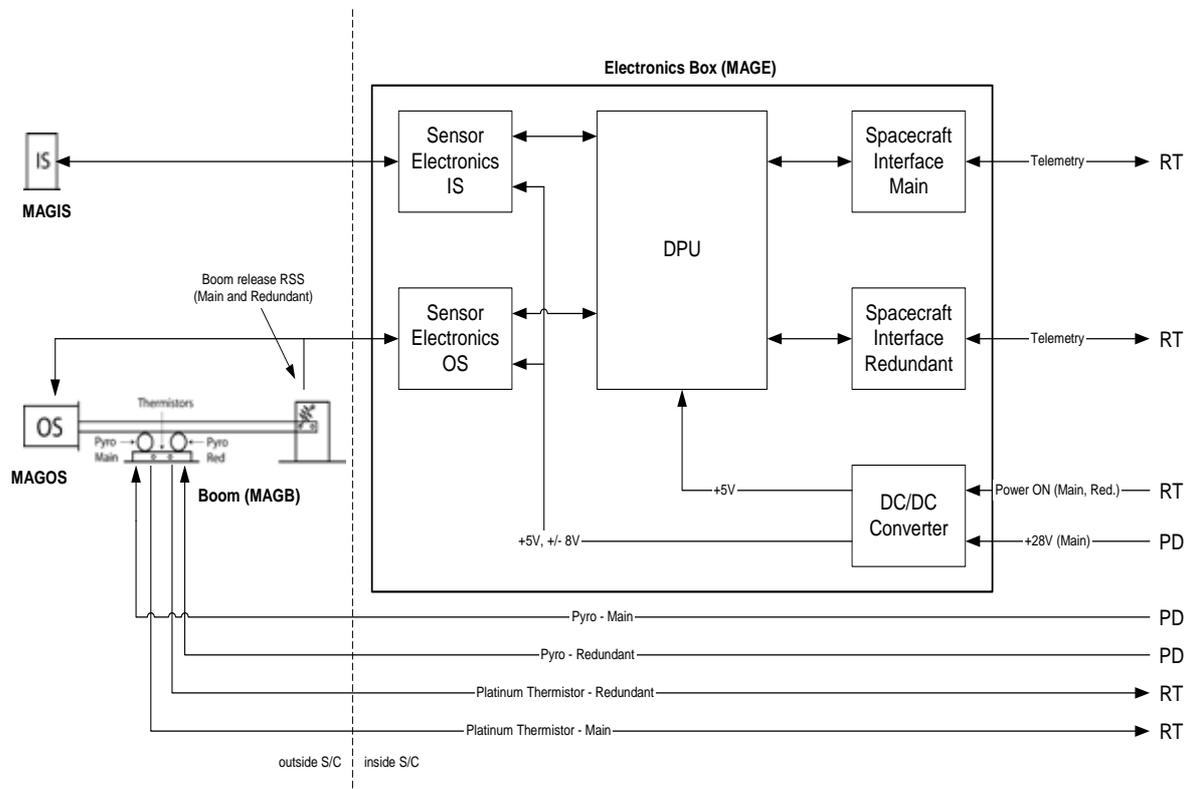
Figure 2. Block diagram of the magnetometer onboard Venus Express
