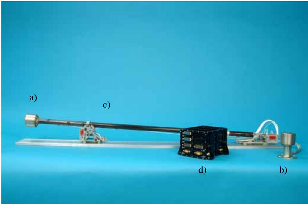
Figure 3. MAG FM: a) outboard sensor, b) inboard sensor, c) boom with launch lock and hinge and d) electronics box
