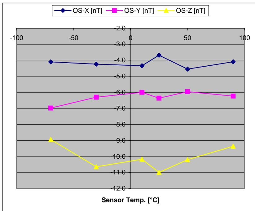
Figure 6. Offset as function of sensor temperature for MAG outboard sensor
