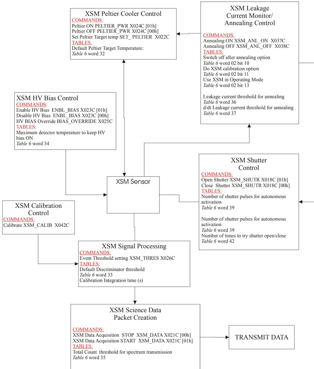
**Figure 5-17 XSM Control Parameters**
