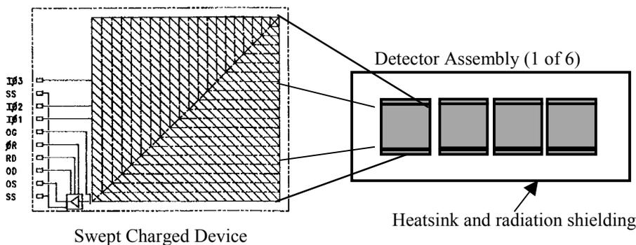
**Figure 5-3 Detector Configuration**
