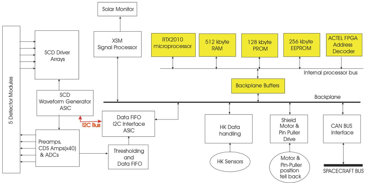
**Figure 5-6 Data Processor System**
