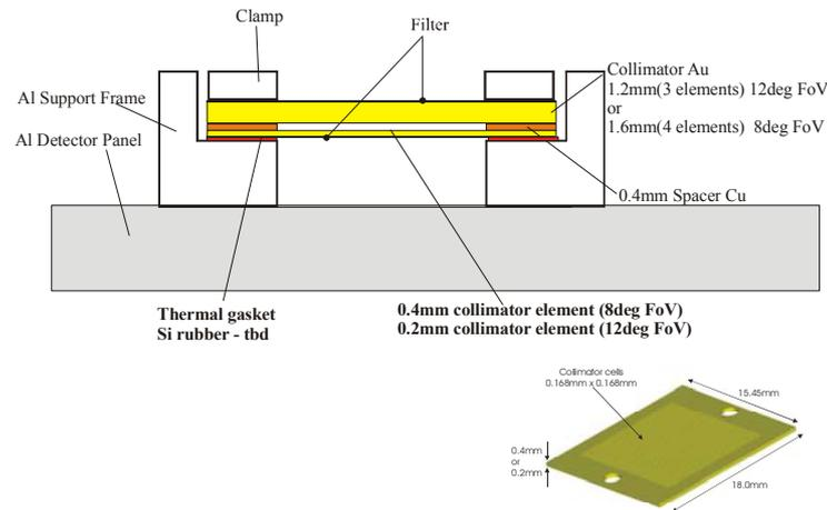
**Figure 5-2 Detector Assembly**
