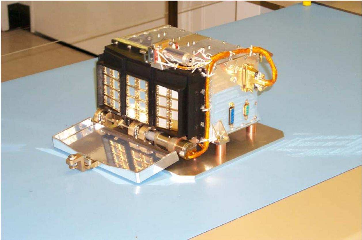
**Figure 5-7 Radiation Shield**
