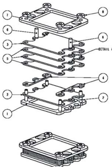
**Figure 5-4 Collimator/Filter Configuration**
