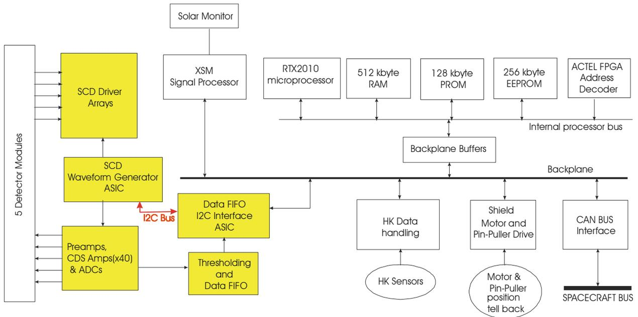
**Figure 5-5 Swept Charged Device Readout System**
