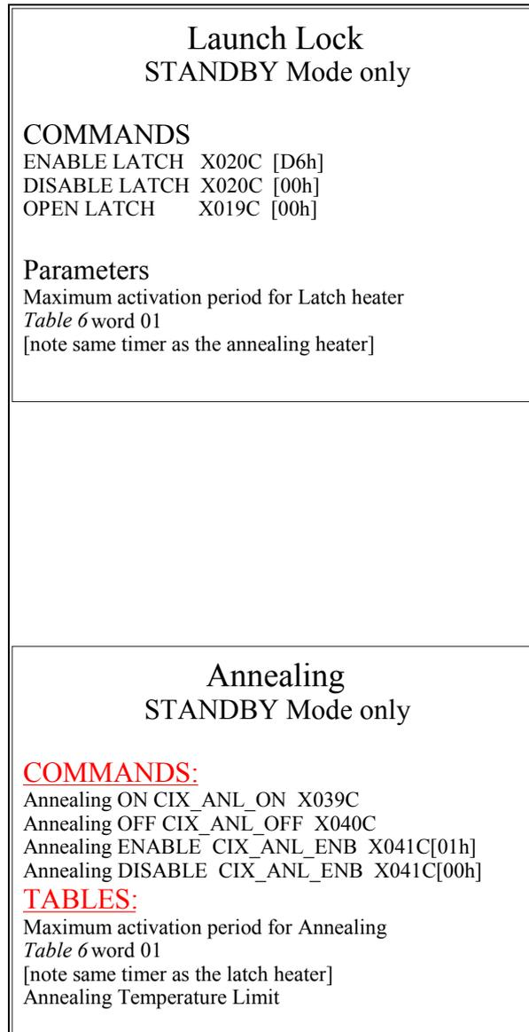
**Figure 5-16 DCIXS Launch Lock and Annealing Parameters**
