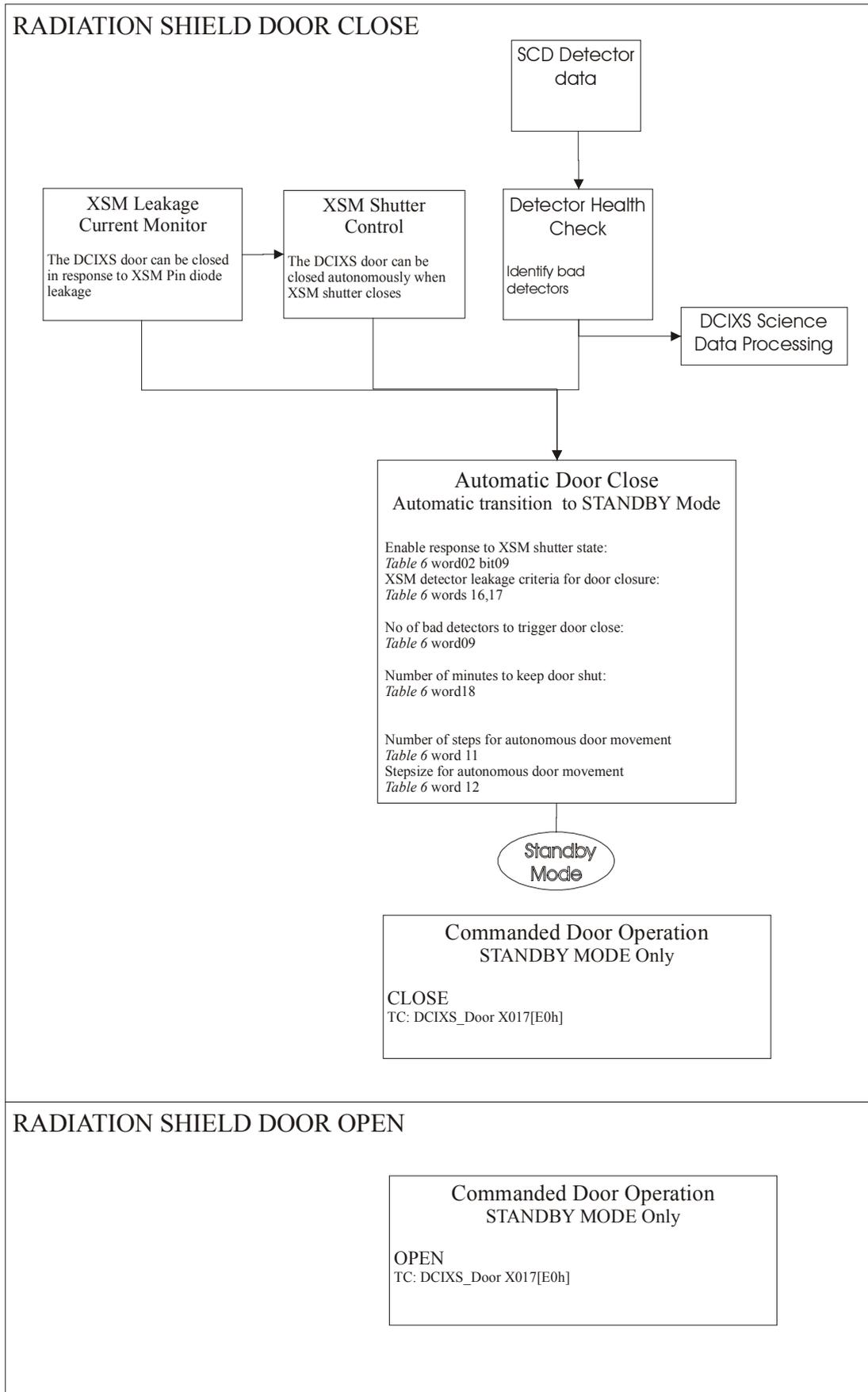
Figure 5-15 Radiation Shield Control Parameters
