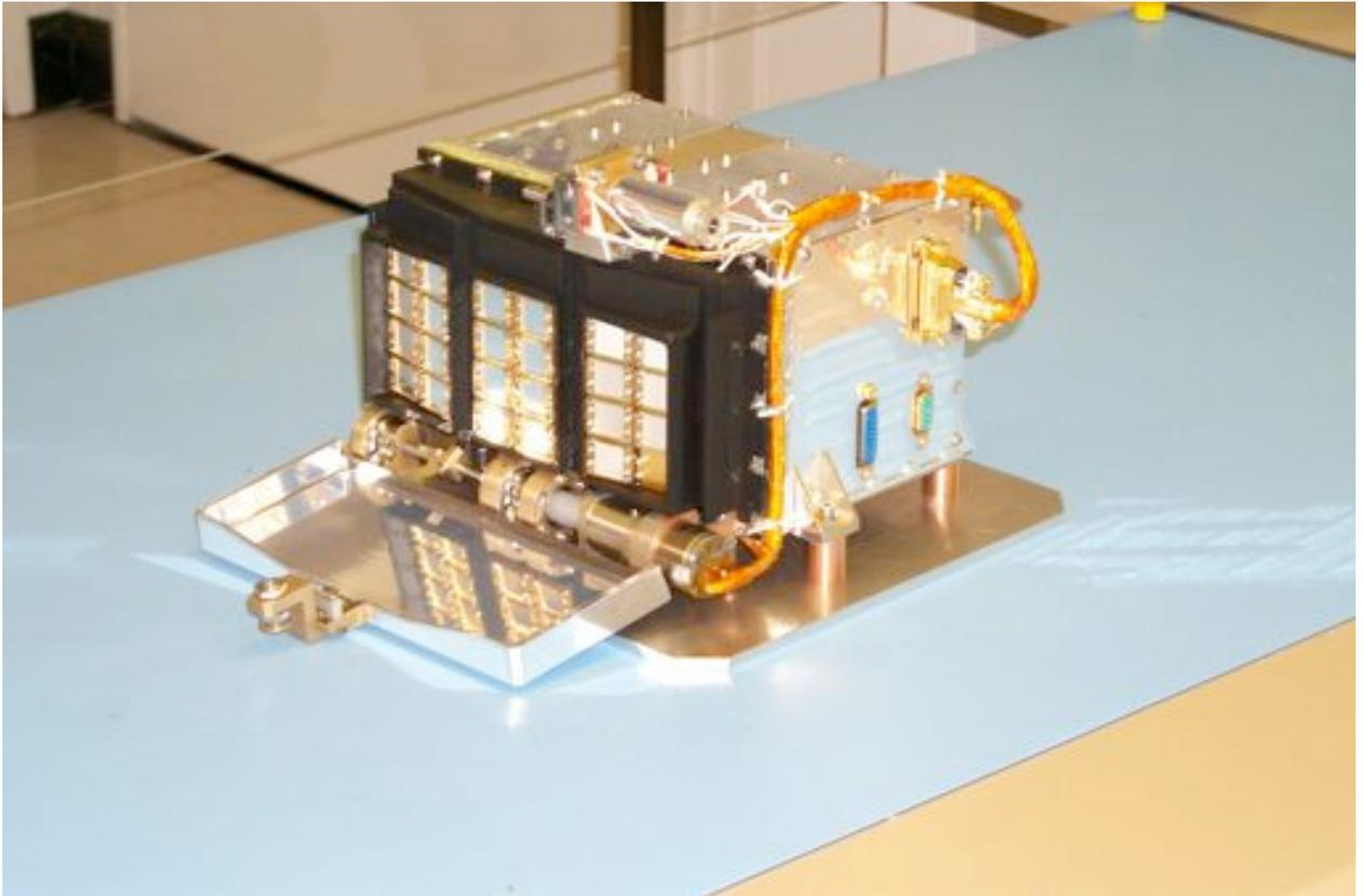
*Figure 2-6 Radiation Shield*
