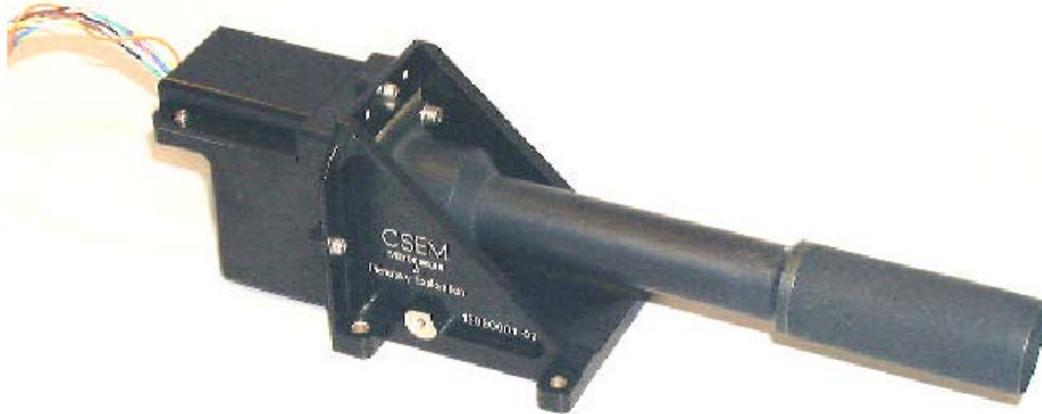
**Figure 2: Photograph of the AMIE camera head (Unit 1).**
