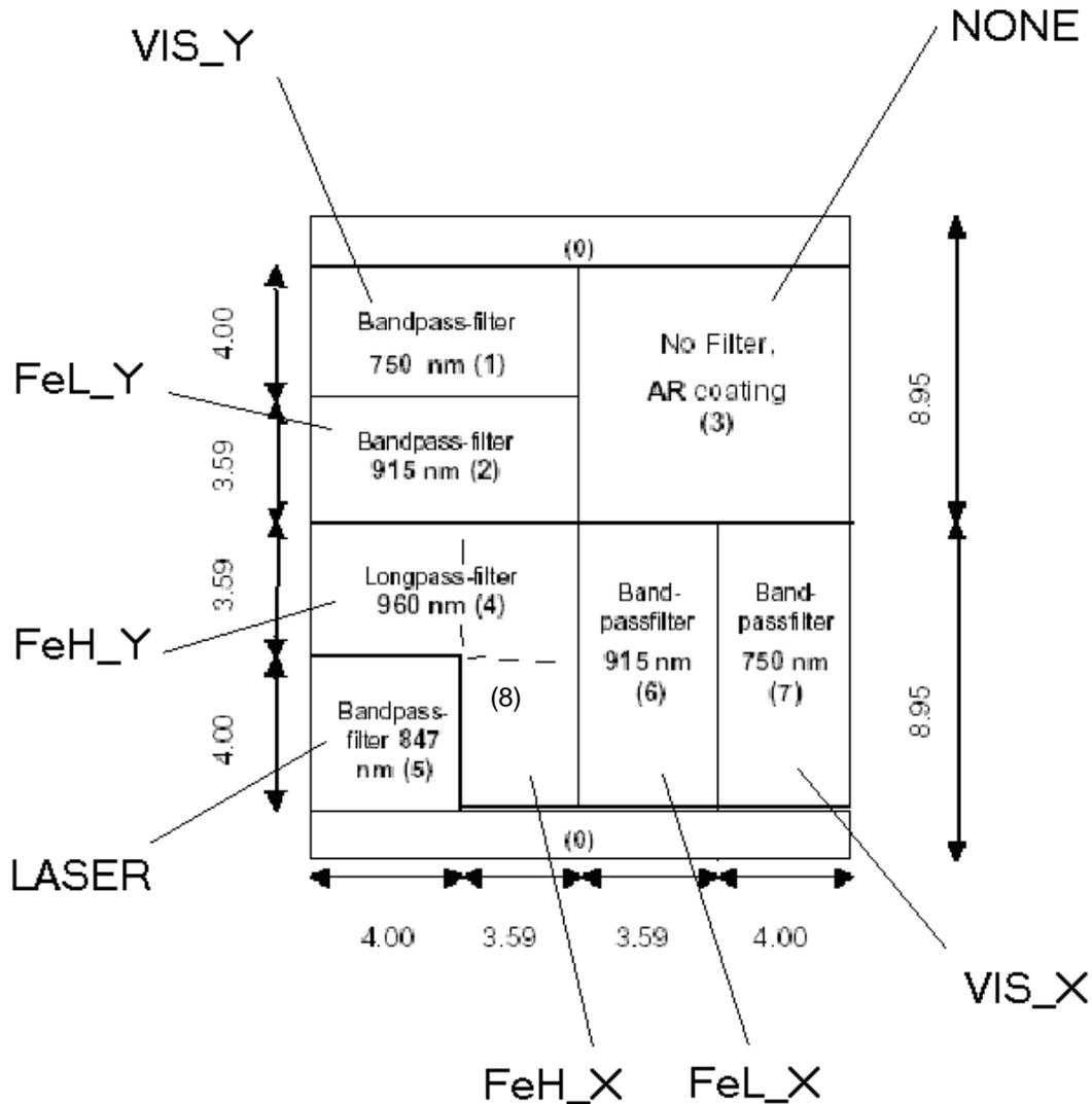
**Figure 4: Filter layout in front of the detector. '0' denotes that the filter area is outside the detector. The following filter names are used: '1' = VIS\_Y, '2' = FeL\_Y, '3' = NONE, '4' = FeH\_Y' (horizontal area) and FeH\_X (vertical area), '5' = LASER, '6' = FeL\_X, '7' = VIS\_X.**
