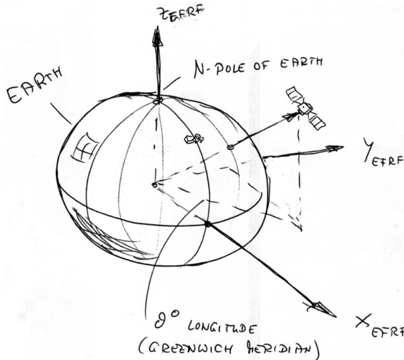
Figure 6: Definition of the Earth-fixed reference frame (EFRF).
