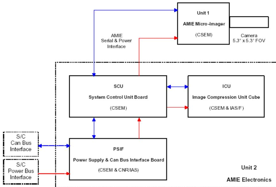
**Figure 1: Main hardware functions of AMIE.**
