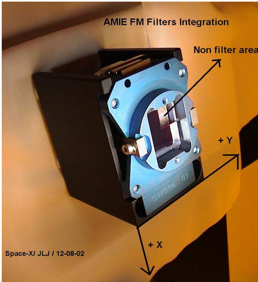
**Figure 3: Photograph of AMIE sensor head without optics.**
