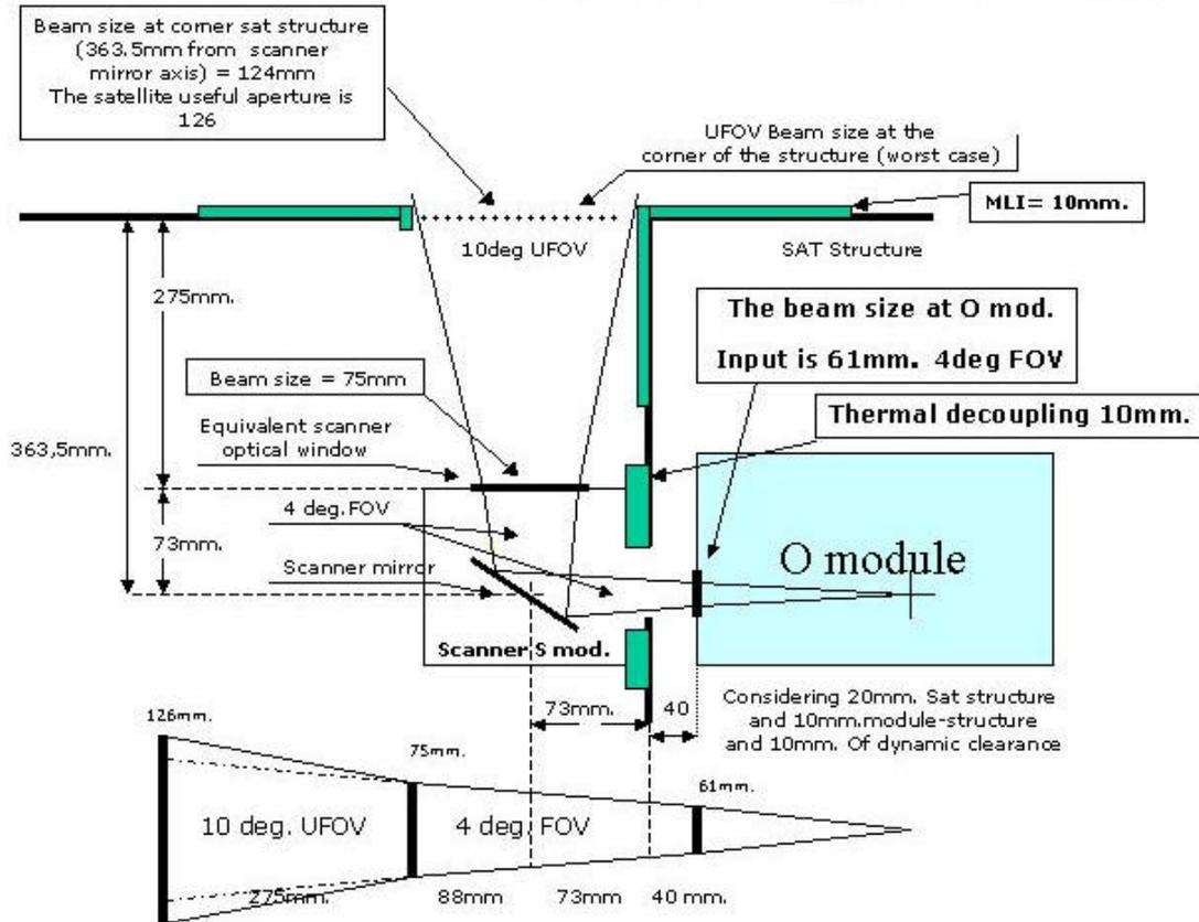
**Fig. 1.13 NOTE:** in the figure above the exit of O module should be 65 mm not 61 .
