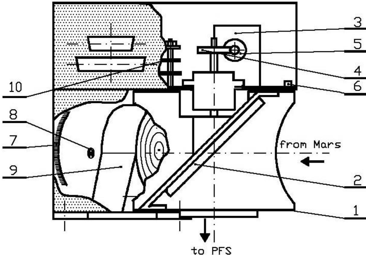
The cylindrical housing (1) has a round empty window (an entrance window with diameter  $\Phi 88\text{mm}$ ) through which the IR radiation to be measured comes to the mirror and goes through an exit window (diameter  $\Phi 78\text{mm}$ ) to PFS-O optical inlet. The axis of optical outlet of PFS-S must coincide with the axis of PFS-O's inlet within  $0.1^\circ$ .
