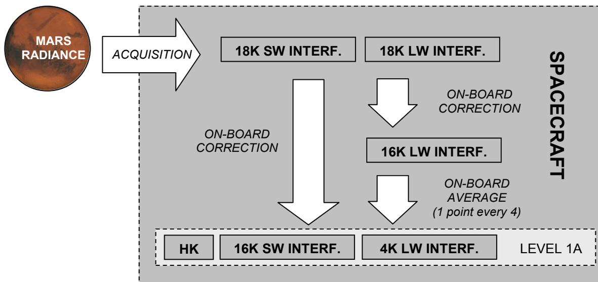
Fig.2 PFS data acquisition and processing scheme.
