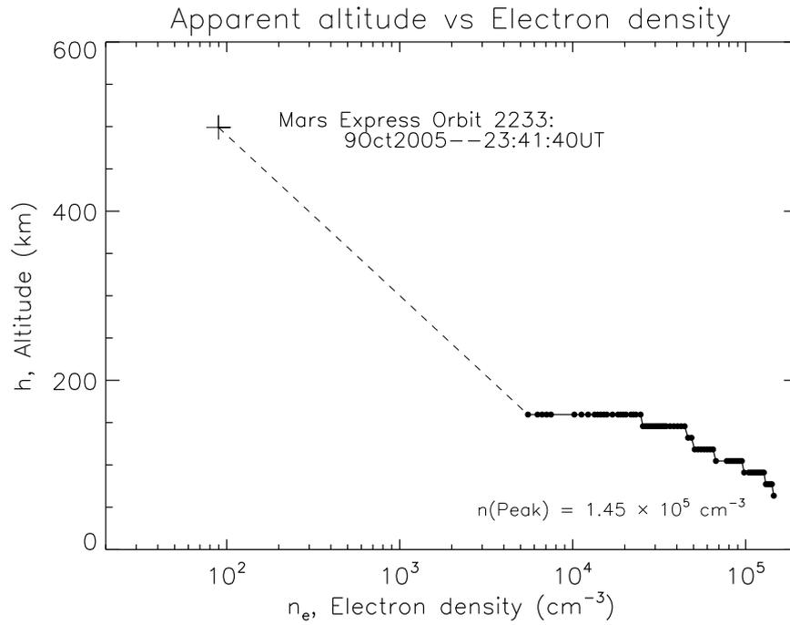
**Figure 2.** Apparent altitude vs electron density converted from the white curve of apparent range vs plasma frequency in Fig. 1. Apparent altitude is obtained by subtracting apparent range from the spacecraft altitude. Electron density is obtained from plasma frequency by equation 2. The black dots represent data points written to file from the original ionogram. The large plus sign represents the altitude and electron density at the spacecraft.
