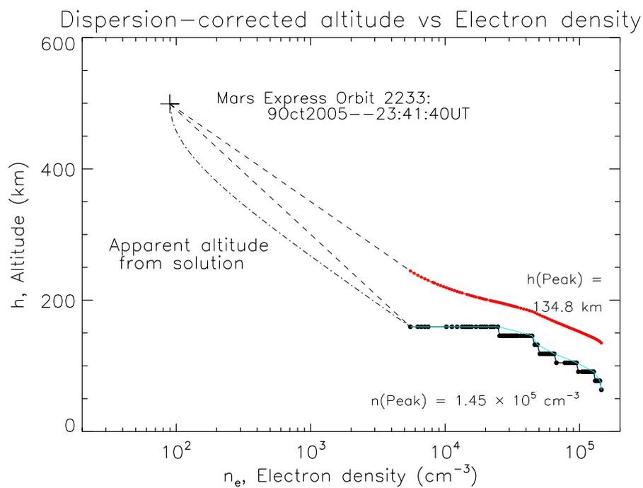
**Figure 4.** Identical to Fig. 3 except that the corrected altitude, according to equation 8 is now shown in red. The dot-dashed curve is the apparent altitude as a function of electron density inferred from the inversion solution. The ionospheric density peak is computed to occur at 134.8 km altitude.
