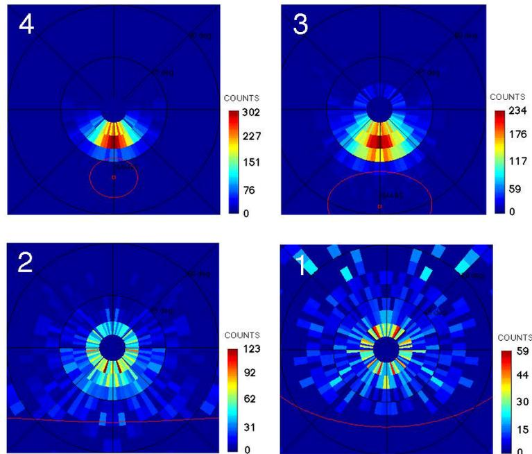
**Figure 8.** ENA images expected from NPI for four locations along the Mars Express orbit specified in Figure 2. The images were generated assuming the instrument characteristics given in Table 2. The projection is similar to Figure 3.
