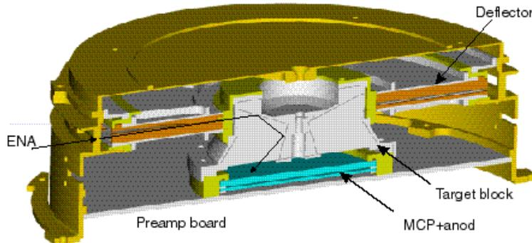
**Figure 7.** Cut-away view of the NPI sensor
