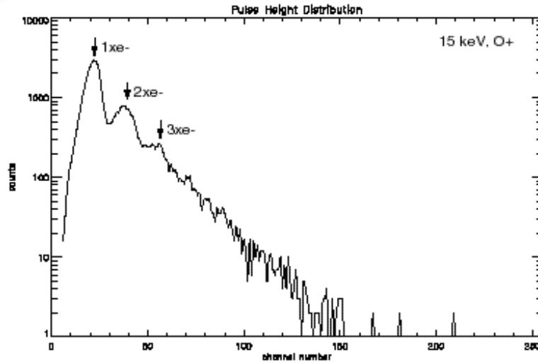
**Figure 15.** Pulse–height distribution of the valid (START-STOP) signals obtained from the STOP MCP under a beam of 15 keV  $\text{H}_2\text{O}^+$  ions.
