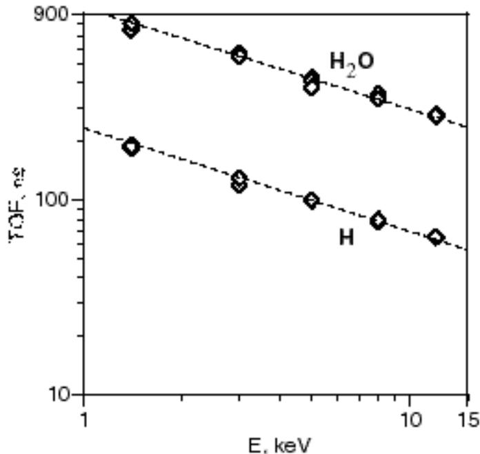
**Figure 14.** The time-of-flight measurements for different masses as a function of energy. The dashed lines give the theoretical dependence corresponding to the 34% energy loss.
