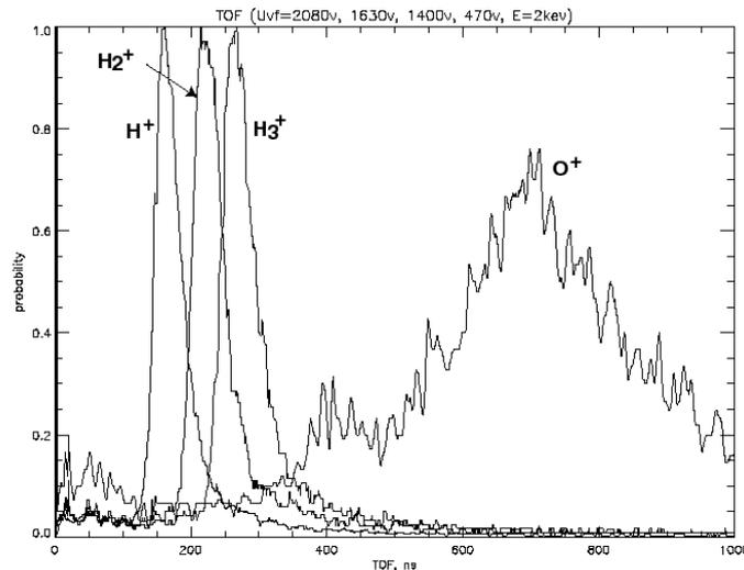
**Figure 13.** NPD TOF spectra for 2 keV beams of different masses.
