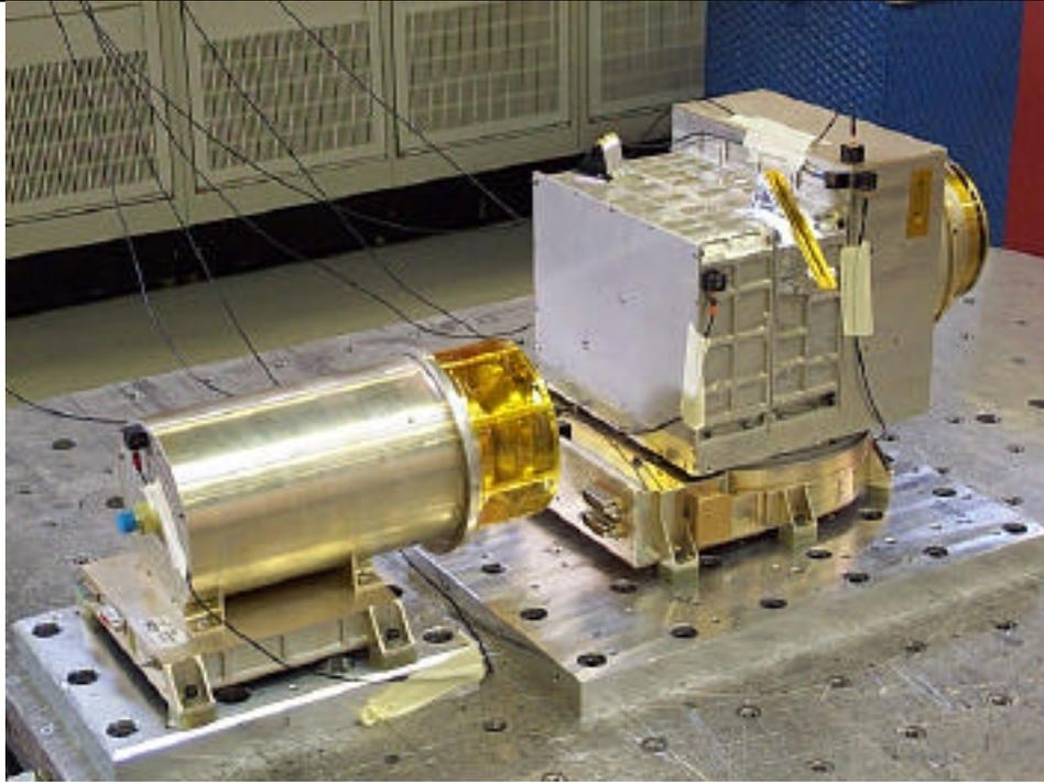
**Figure 6.** The ASPERA-3 instrument, IMA and the Main Unit during a vibration test.
