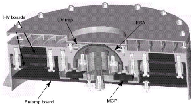
**Figure 16.** Cut-away view of the ELS sensor
