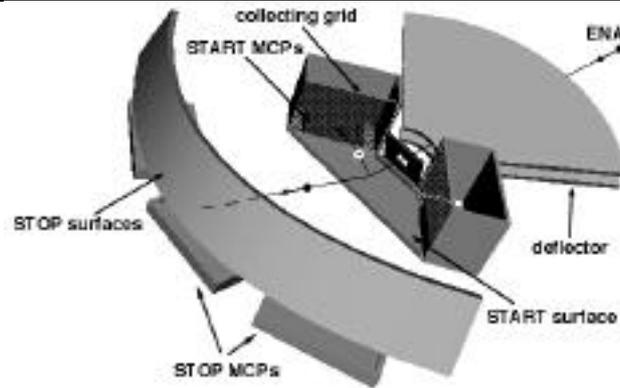
**Figure 9.** Three-dimensional view of the NPD principal components
