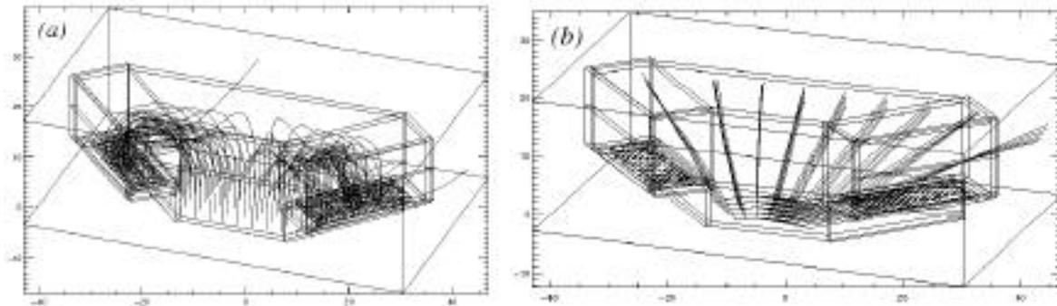
**Figure 10.** The ray-tracing of the electron (a) and 80 eV ion trajectories (b) in the START assembly electron optics.
