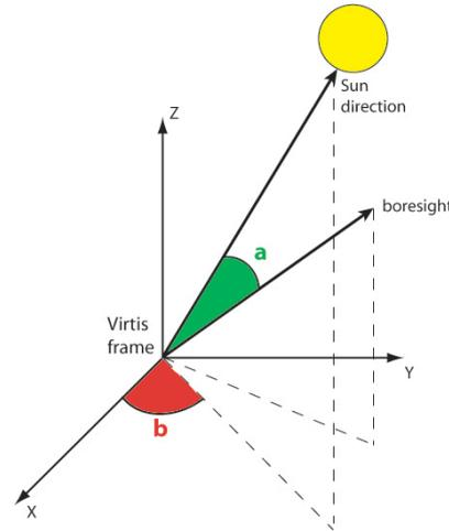
Figure 4: Sun direction in the instrument frame
