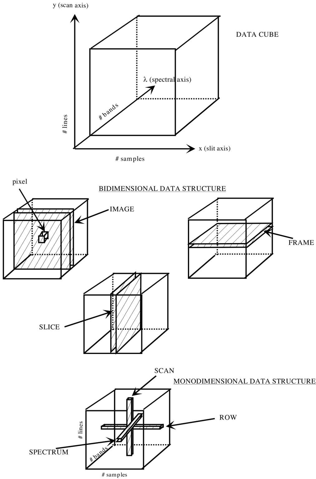
Figure 4-1: Structure of the cube data
