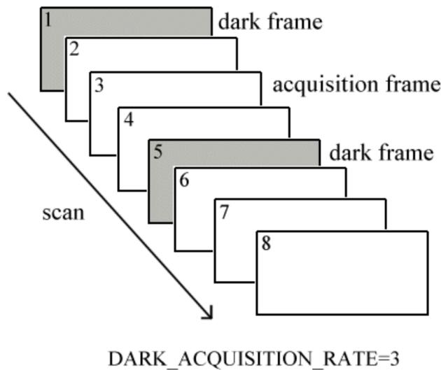
Figure 4-2: Structure of dark frames acquisition.
