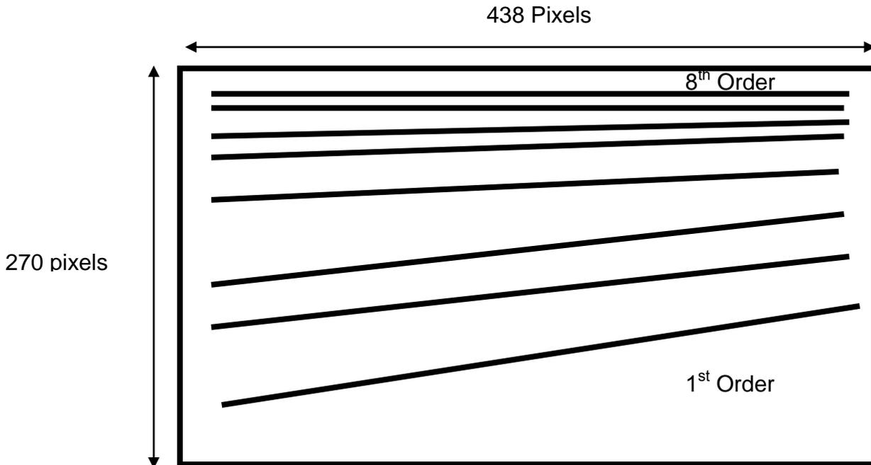
Figure 3.5 Spectral orders distributed over the IR FPA area. Only 15% of the matrix contains scientific data.
