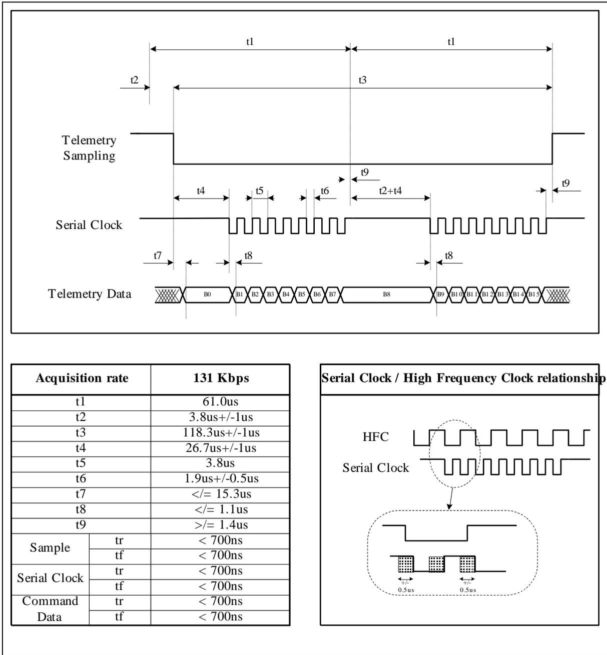
Figure 2.5 16Bit Serial Digital Telemetry (SDT) timing
