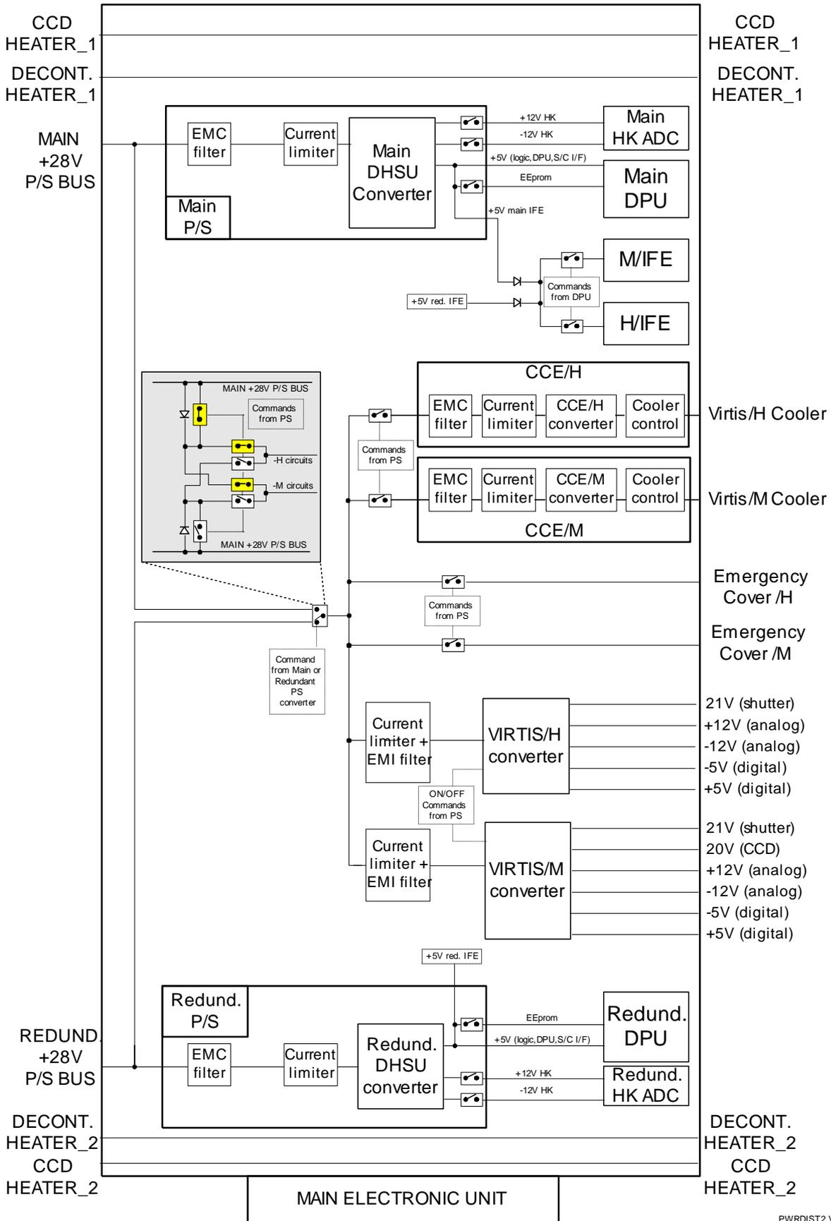
Figure 2.1 Power switching and Distribution block diagram.
