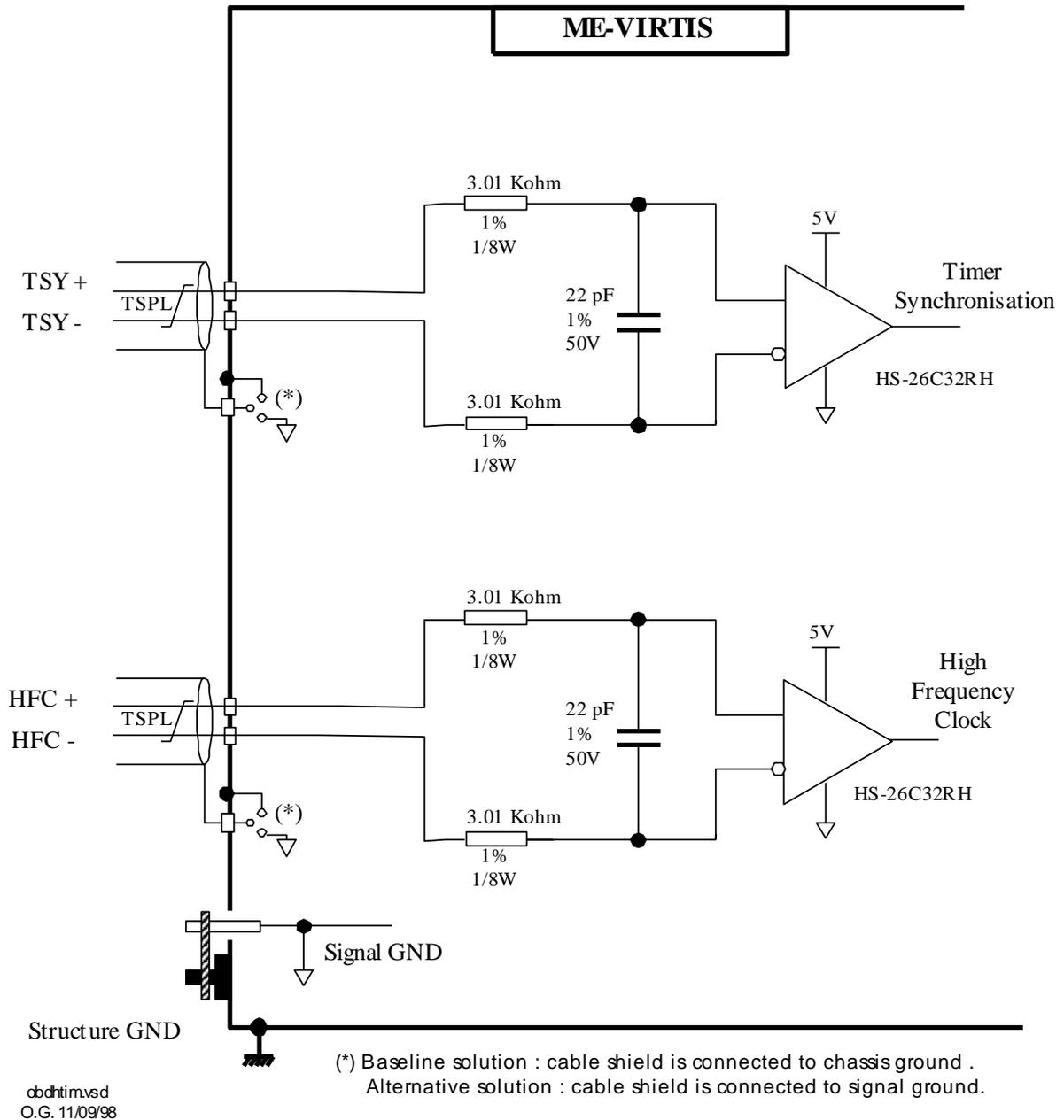
Figure 2.9 DMS timing & synchronisation signal (OTS) interface circuit
