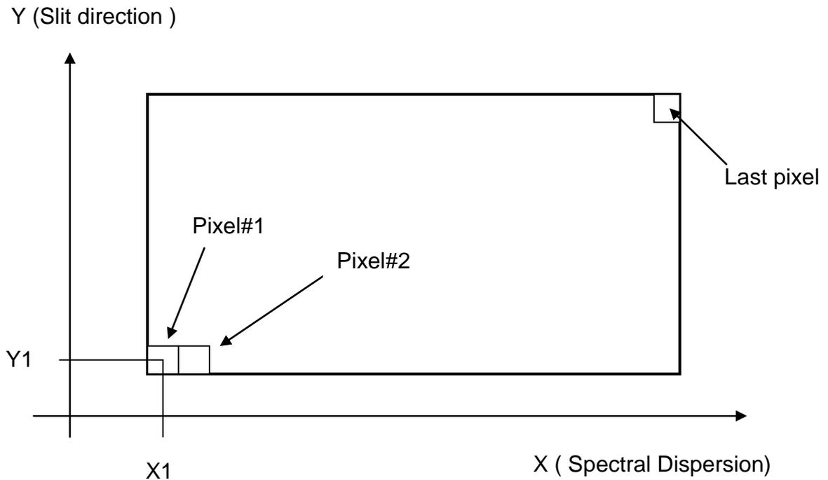
Figure 3.4 Data Organisation on the CCD and IR detectors of VIRTIS-M
