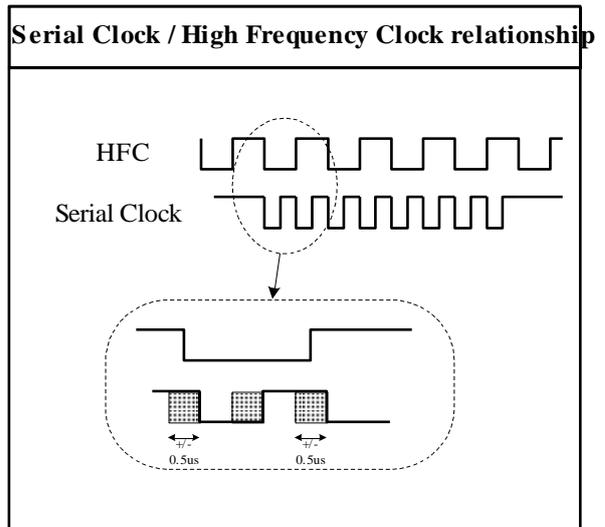
Figure 2.3 MLC (Memory Load Command) timing characteristics
