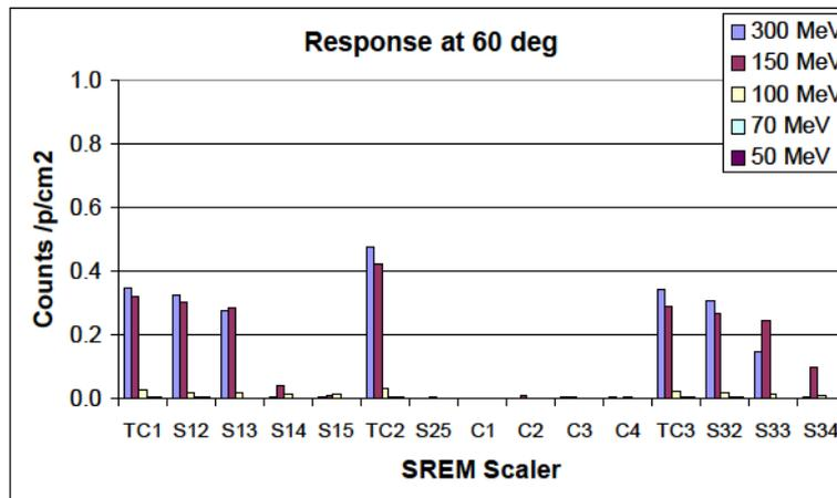
Figures 9: SREM scaler response for different energies and  $\Theta = 60^\circ$ .
