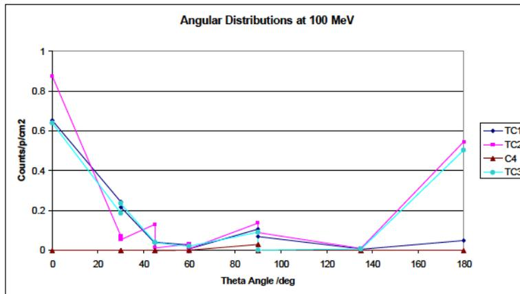
Figures 11: Angular response of TC1, TC2, TC3 and C4 scalers at 100 MeV.
