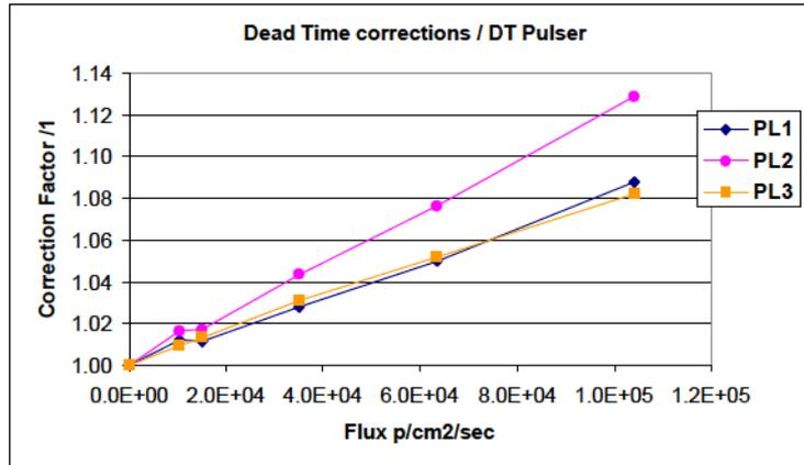
Figure 4. Deadtime corection factors from PLi scalers.
