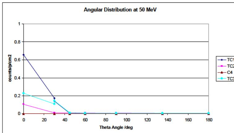
Figures 10: Angular response of TC1, TC2, TC3 and C4 scalers at 50 MeV.
