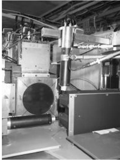
Photo: SREM unit, plastic detectors and ionization chamber during PIF calibrations.
