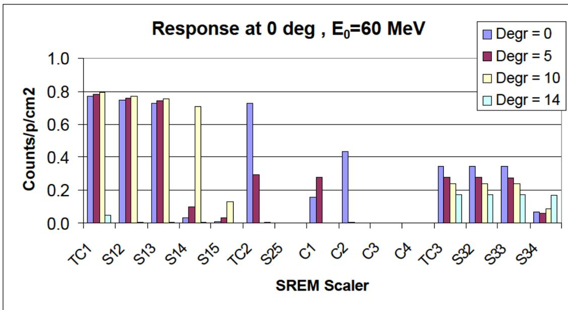
Figure 2. Normalized response of the SREM for 60 MeV protons at  $\Theta=0^\circ$  and different Al degrader thickness.
