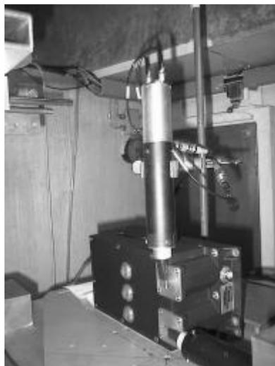
Photo: SREM unit placed on the angular stage with two plastic detectors in front.
