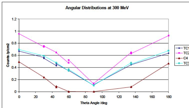
Figures 12: Angular response of TC1, TC2, TC3 and C4 scalers at 300 MeV.
