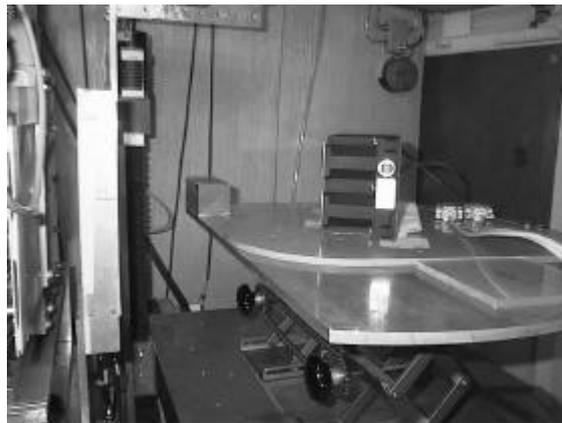
Photo: SREM unit placed on the angular stage during calibration runs at PIF.
