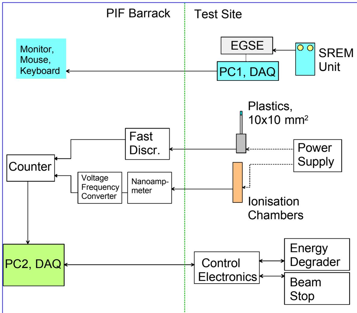
Figure 1: Data acquisition and measurement set-up for SREM proton tests.
