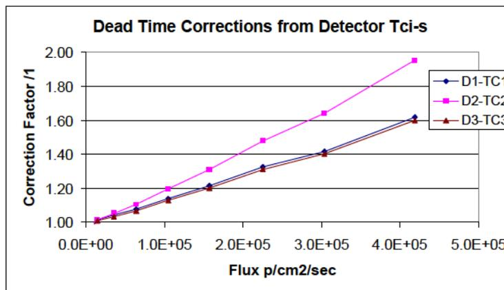
Figure 6. Deadtime corrections als function of the proton flux taken from TCi scalers.
