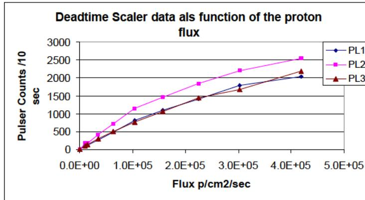
Figure 5. Nonlinear dependence of the deadtime scalers for higher particle fluxes.
