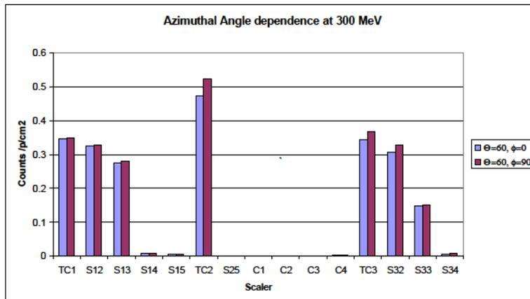
Figure 13. SREM response in function of the azimuthal angle  $\phi$  at 300 MeV ( $\Theta=60^\circ$ ).
