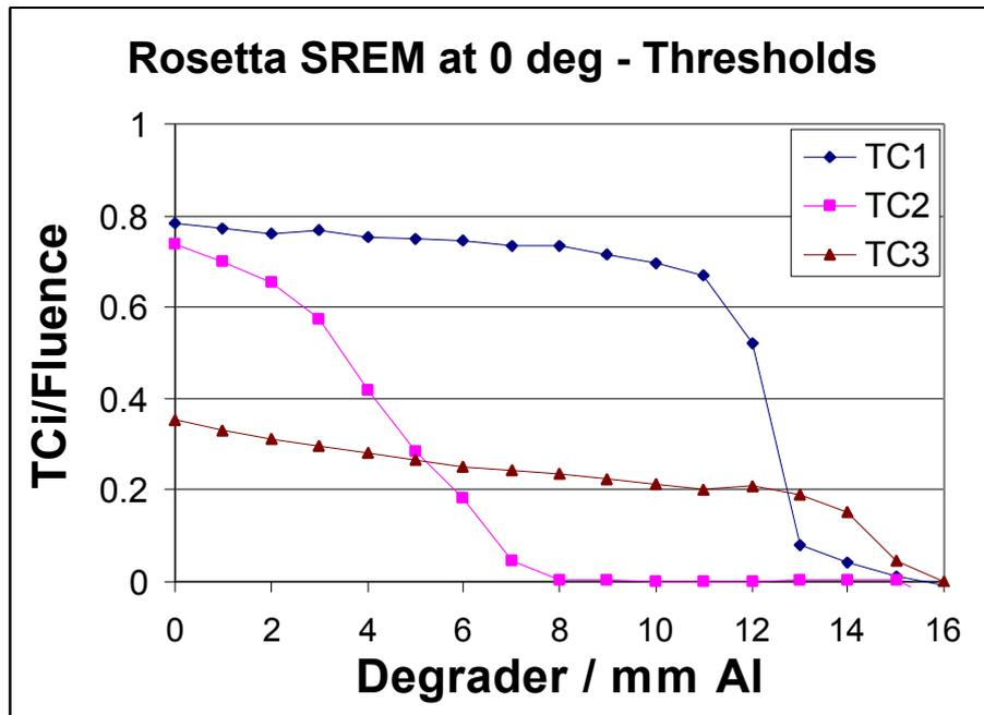
Figure 3: Response curves for SREM scalers TC1, TC2 and TC3 as function of the degrader (proton energy) used to determine low energy thresholds (raw data).
