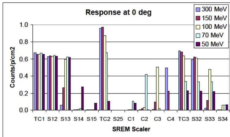
Figures 7: SREM scaler response for different energies and  $\Theta = 0^\circ$ .
