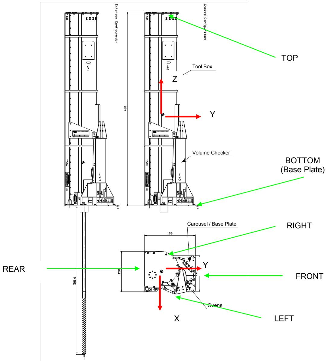
Figure 3 SD2 system in stowed and extended configuration
