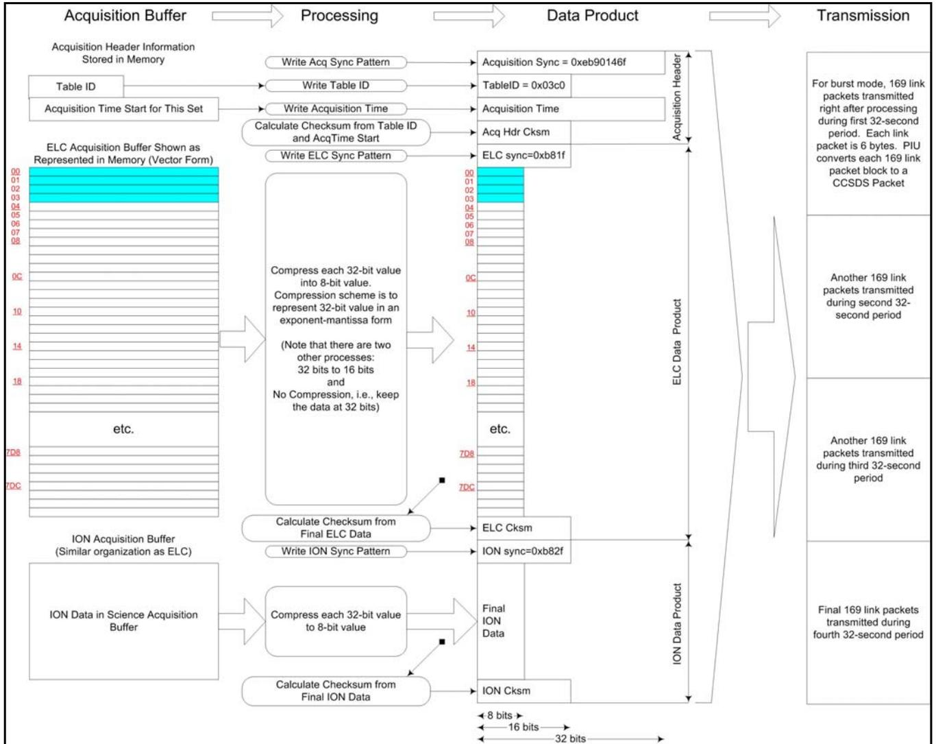
Figure 2.3-4: IES Science Acquisition, Processing Detail for a 128 s Cycle
