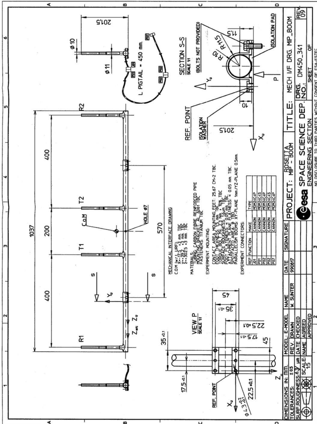
Figure 2.1-8: MIP Mechanical Interface Drawing
