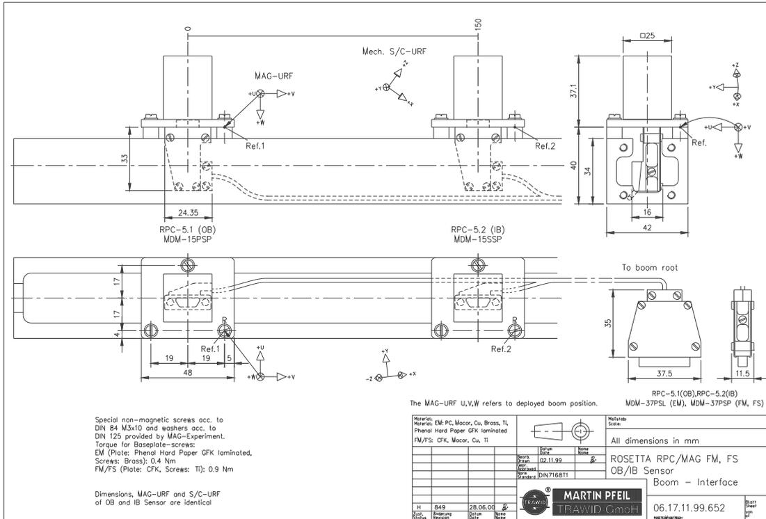
Figure 2.1-10: MAG Sensor Boom Interface
