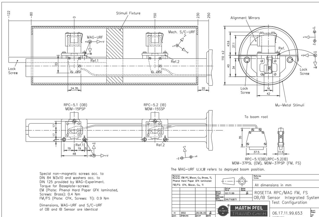
Figure 2.1-11: MAG Sensor Integrated System Test Configuration
