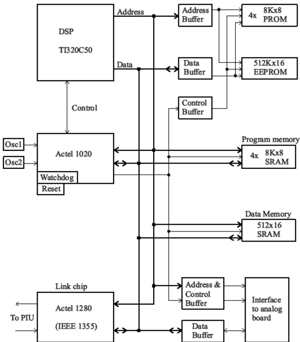
Figure 1.2-6: Langmuir Probe (LAP) Block Diagram for the digital electronics
