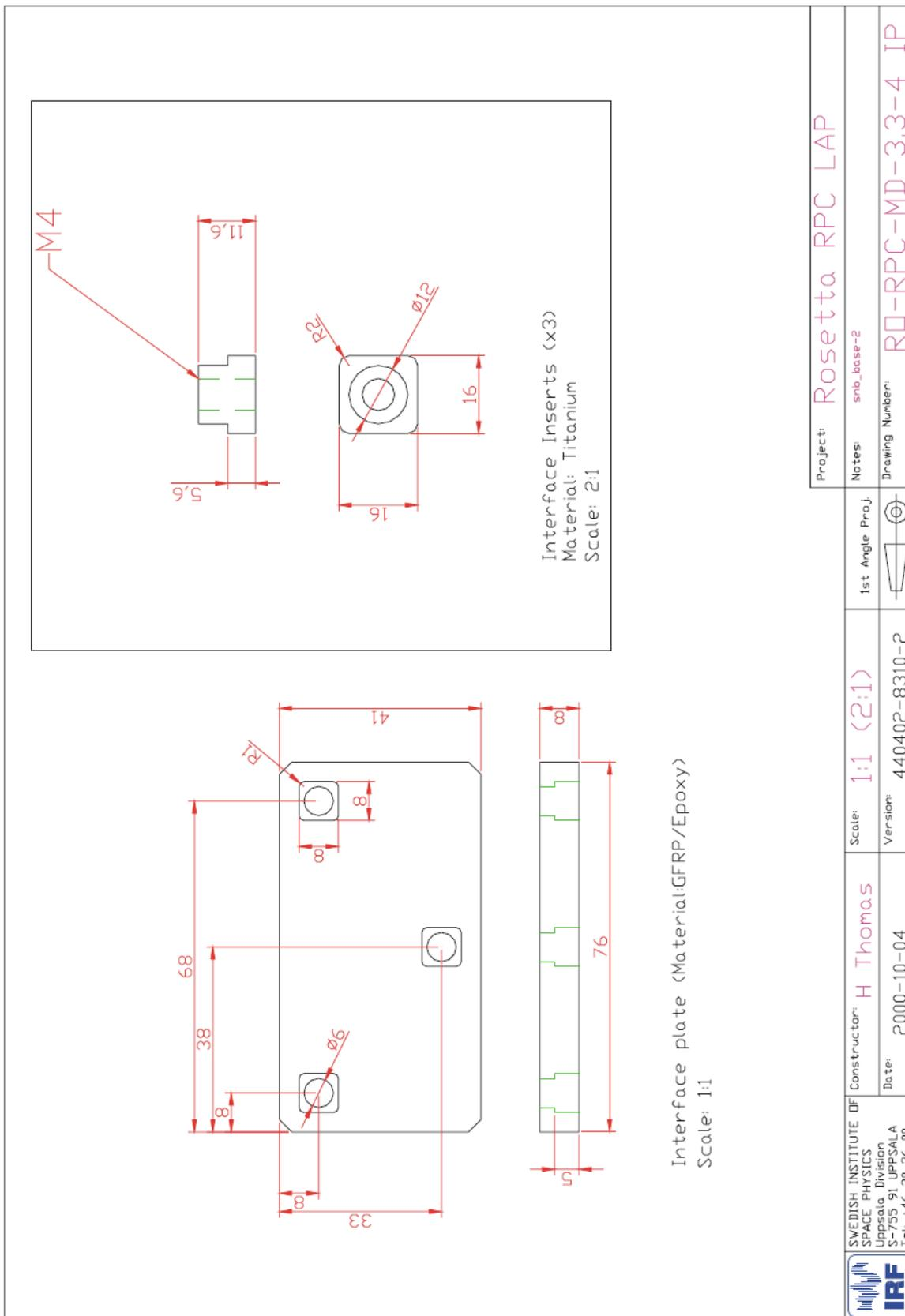
Figure 2.1-7: LAP Support Bracket (I/F Plate) MICD
