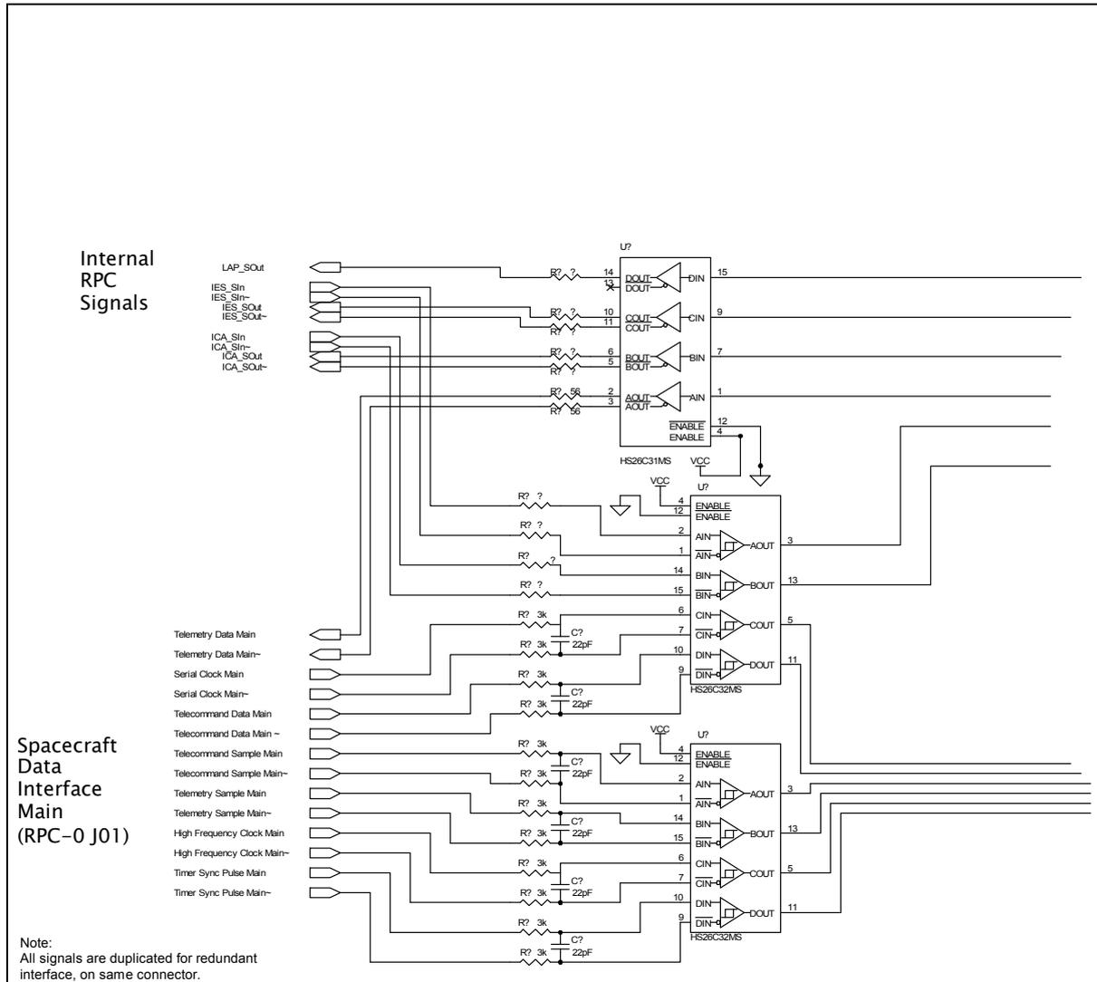
Figure 2.2-2: SDBL Interface Circuits
