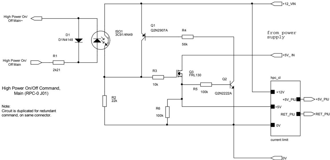
Figure 2.2-3: High Power Command Interface Circuit
