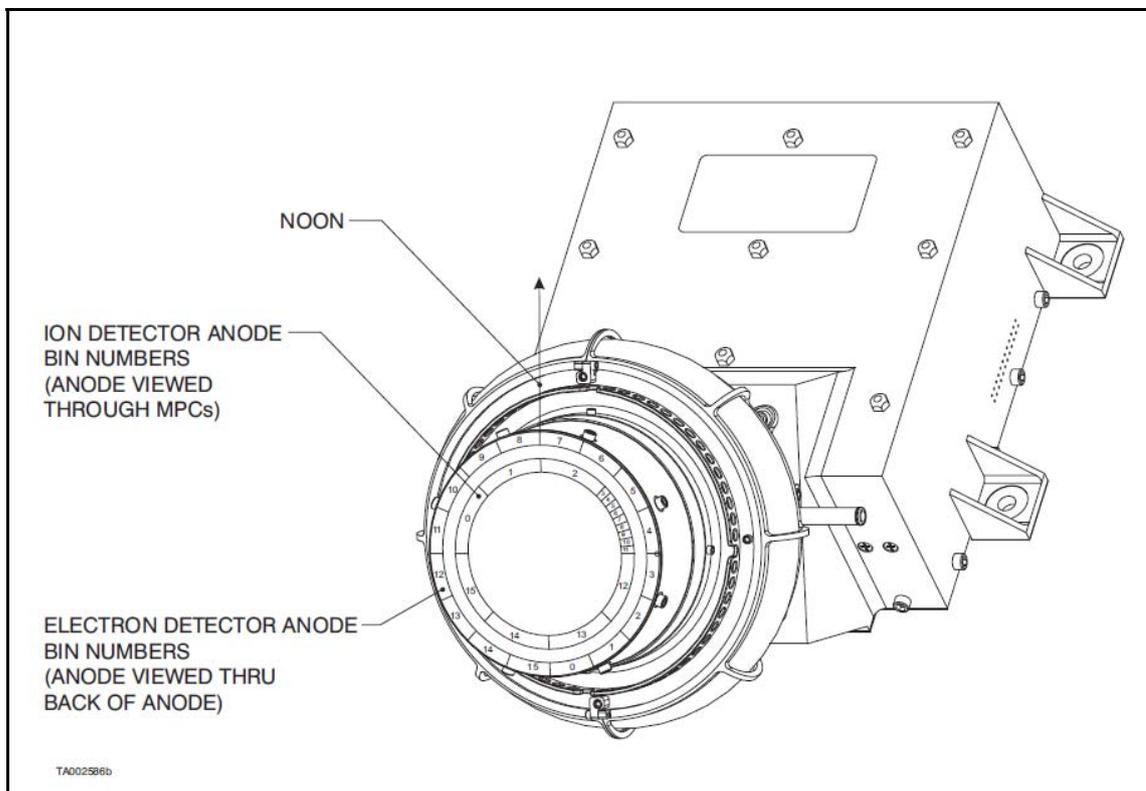
Figure 3.3-4: IES ion and electron MCP anodes layout
