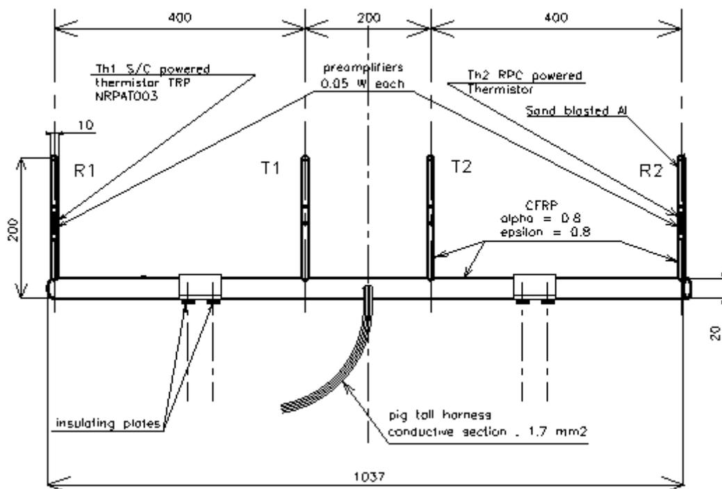
Figure 2.5-5: Thermal Interface Control Drawing for MIP
