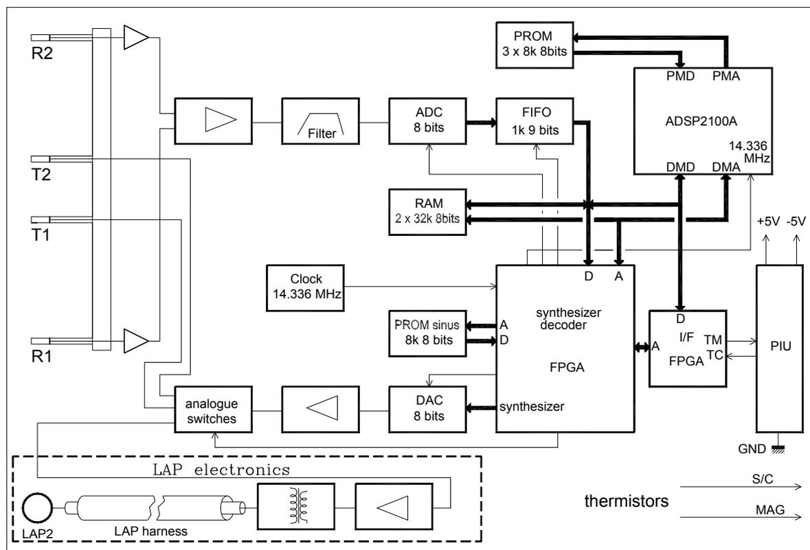
Figure 1.2-10: Mutual Impedance Probe (MIP) Block Diagram
