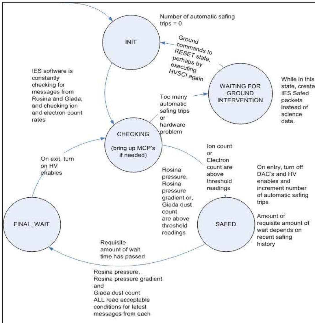
Figure 3.4-1: IES Safing and Autorecovery State Diagram
