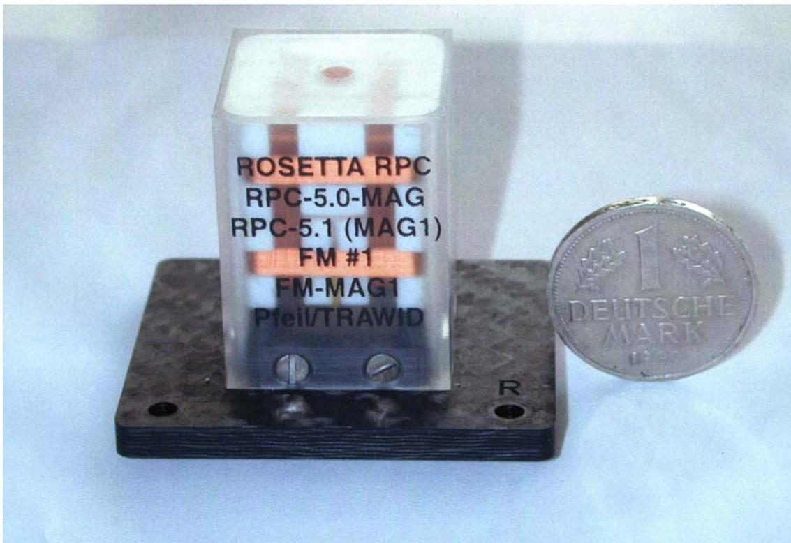
Figure 2.5-7: MAG Sensor with Thermistor
