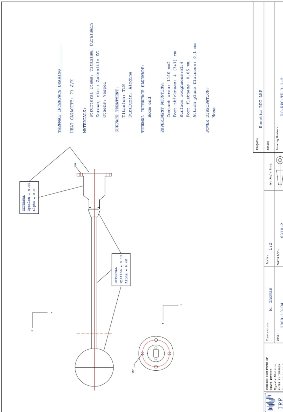
Figure 2.5-4: Thermal Interface Control Drawing for LAP
