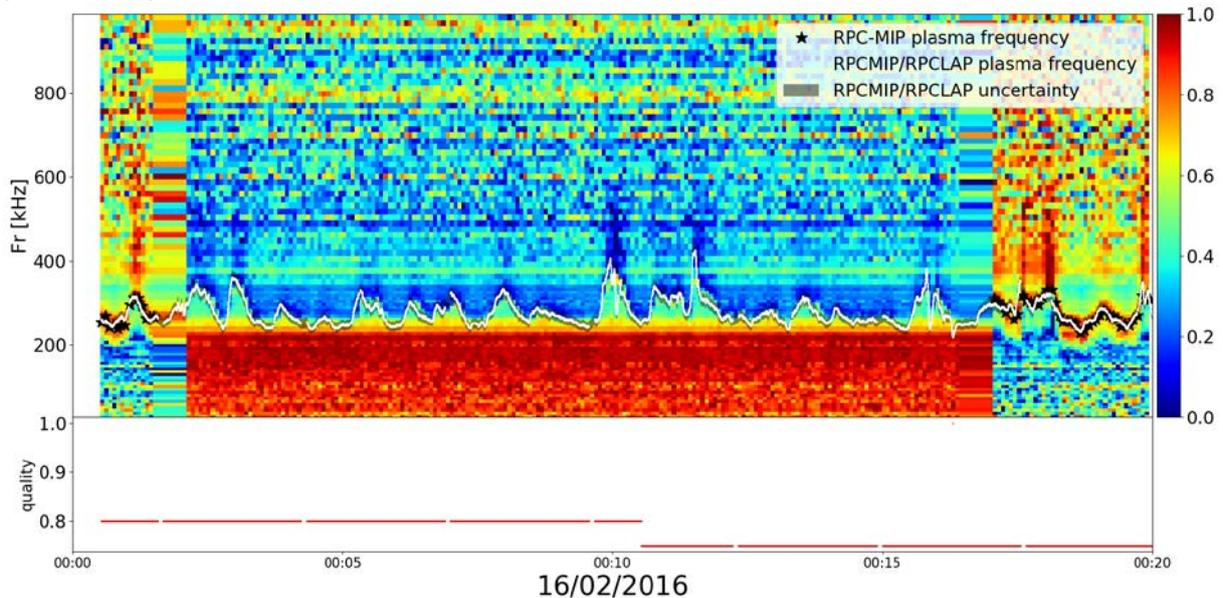
**Figure 7: RPCMIP/RPCLAP densities and small RPC-MIP data gaps.** Top panel: the background represents the color-coded normalized RPC-MIP calibrated power spectra; black stars represent RPC-MIP densities converted to plasma frequencies; white points and the black shaded area represent the RPCMIP/RPCLAP densities and their uncertainties respectively converted to plasma frequency. Bottom panel: red points represent the quality indexes of the cross-calibrated estimates from top panel.
