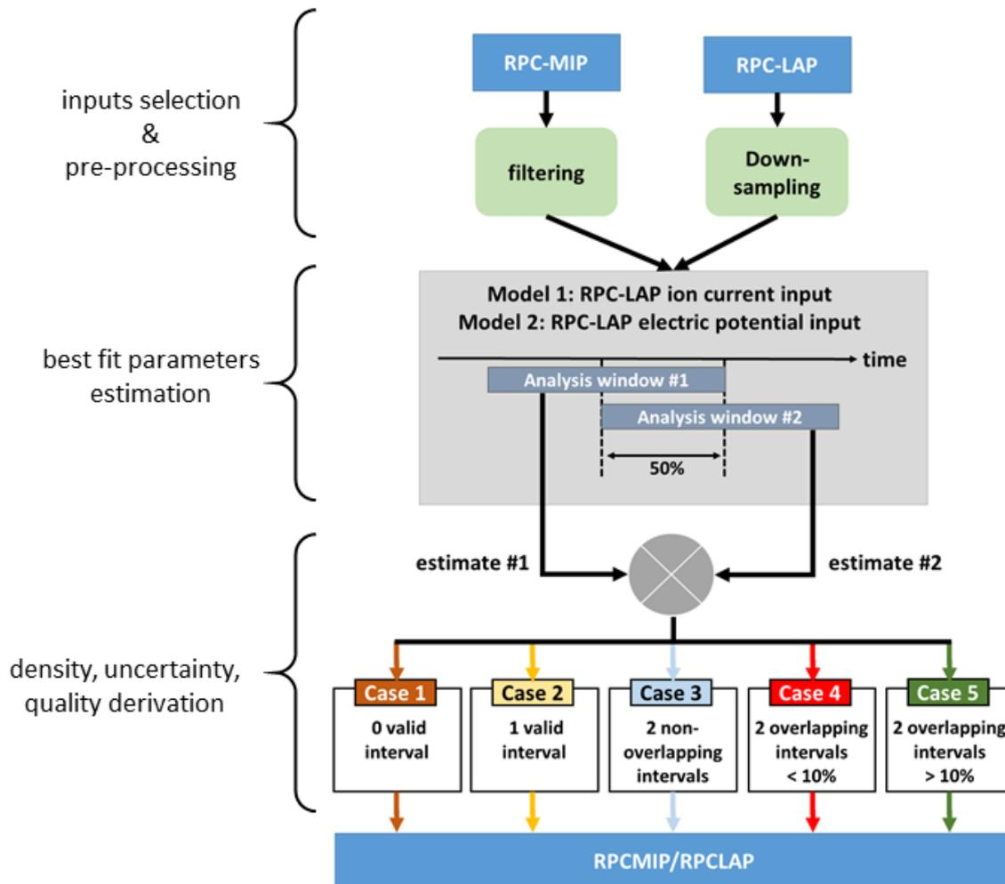
**Figure 1:** Overall cross-calibration procedure for the production of the RPCMIP/RPCLAP dataset.
