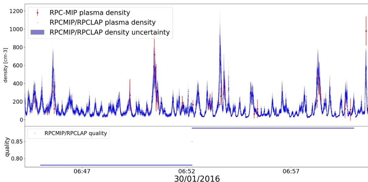
**Figure 6: RPC-MIP/LAP cross-calibration is able to produce low density measurements, not accessible with RPC-MIP only.** Top panel: Red bounded points represent the RPC-MIP densities with the associated density uncertainty. Blue points represent the cross-calibrated densities. Light blue shadow represents the uncertainty of the RPCMIP/RPCLAP density estimates. Bottom panel: blue points represent the quality of the RPCMIP/RPCLAP density estimates.
