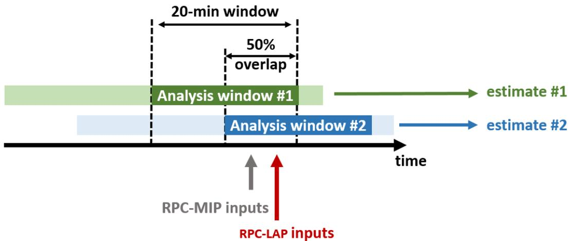
**Figure 2: Example of sliding window approach.** The green and blue boxes represent two analysis windows, each of 20 minutes time width and with an advancement step in time of half the window size. From each sliding windows, preliminary density estimates are obtained from RPC-MIP and RPC-LAP inputs. Due to the 50% overlap between sliding windows, two density estimates are, a priori, available for each RPC-LAP input measurement.
