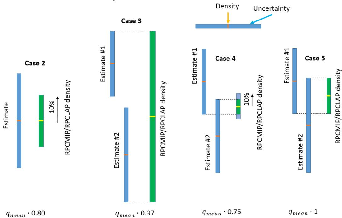
**Figure 3: Possible overlapping cases when comparing estimates from two consecutive analysis windows.** Each bar represents a density interval, where the box at the center and the boxes on the sides represent respectively the density values and the density uncertainties (image on top right side).
