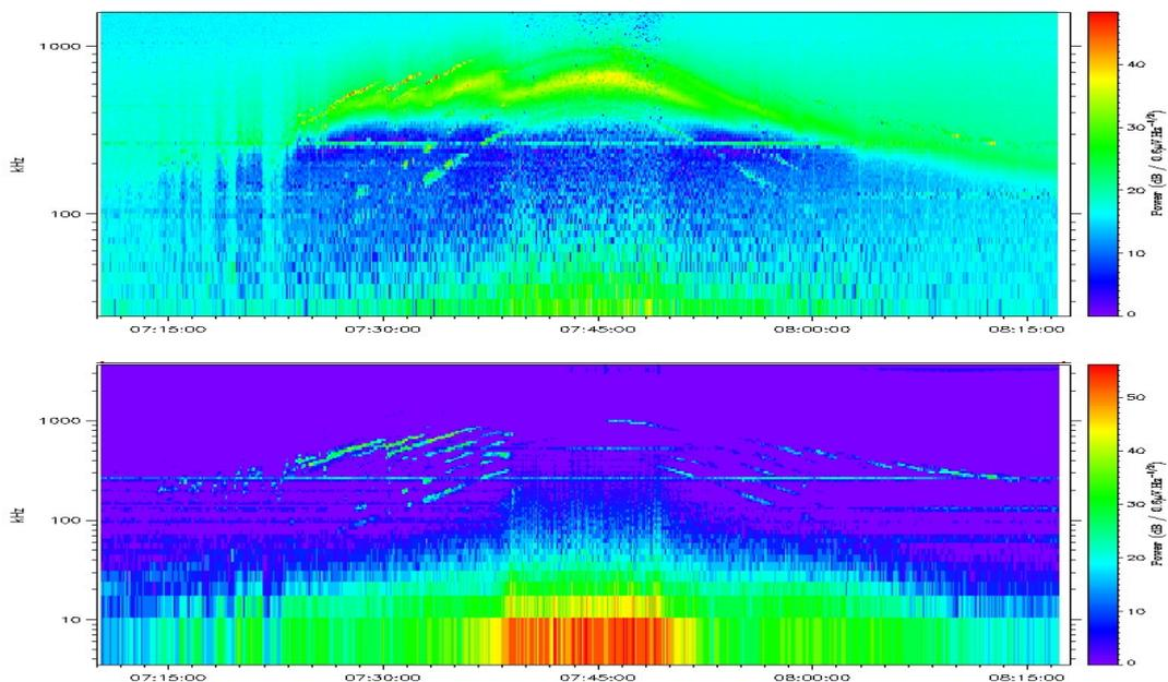
**Figure 4:** Active (top) and passive (bottom) spectrograms for RPC-MIP on 2009 November 13 (Earth Swing-By 3) between 07:10 and 08:20.
