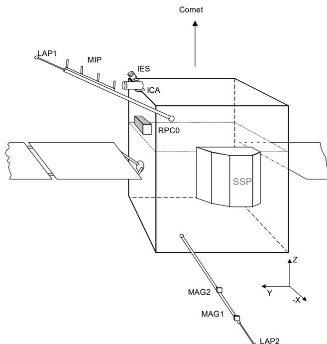
**Figure 1:** RPC Sensors Layout (deployed).
