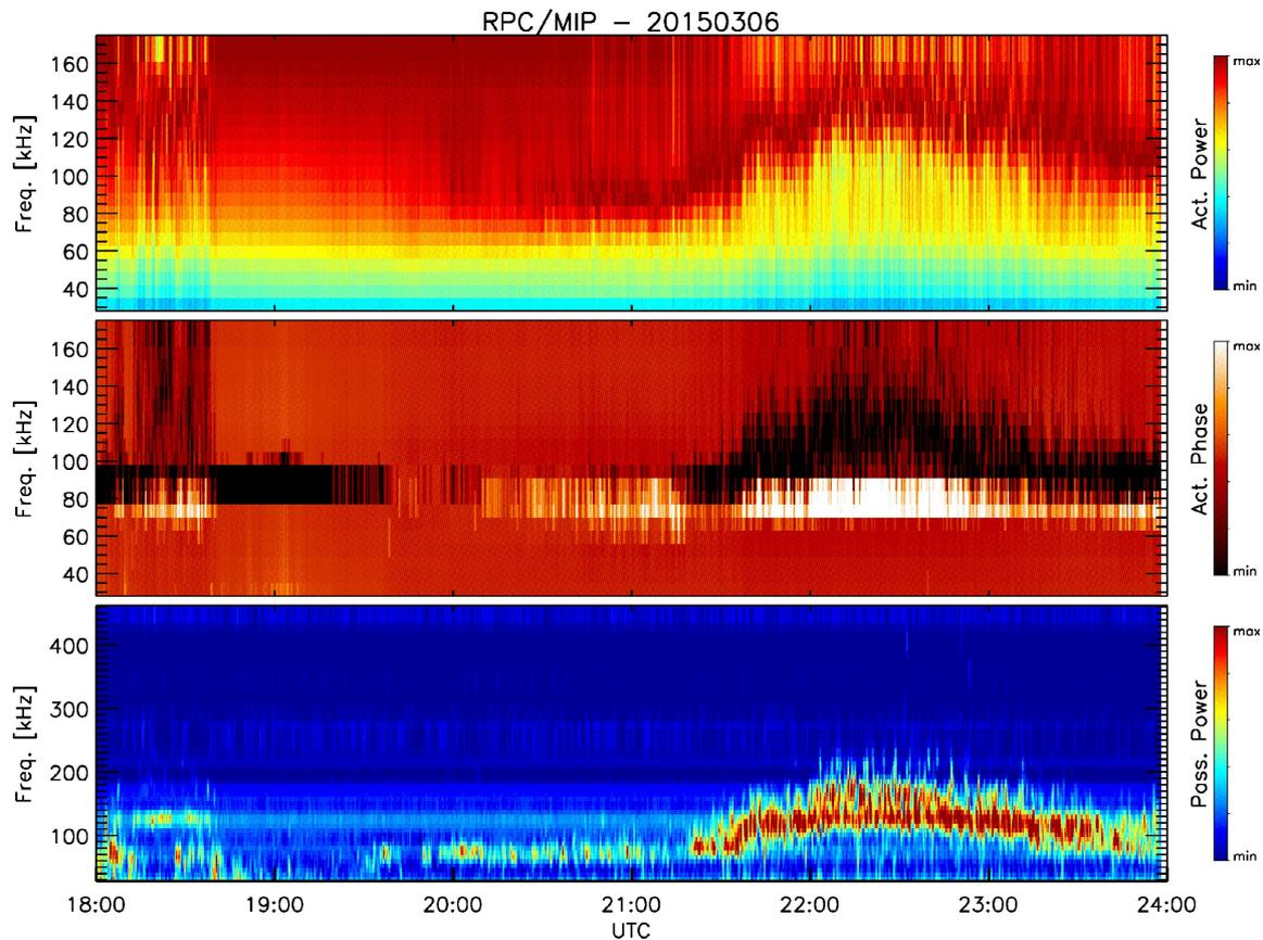
**Figure 3:** Case study of plasma line for 20150306. From top to bottom: LDL active power spectrogram, LDL active phase spectrogram, LDL passive power spectrogram. Data have been processed to remove artificial effects and intrinsic noise and have been normalized (as indicated by the min/max labels on the color scales)
