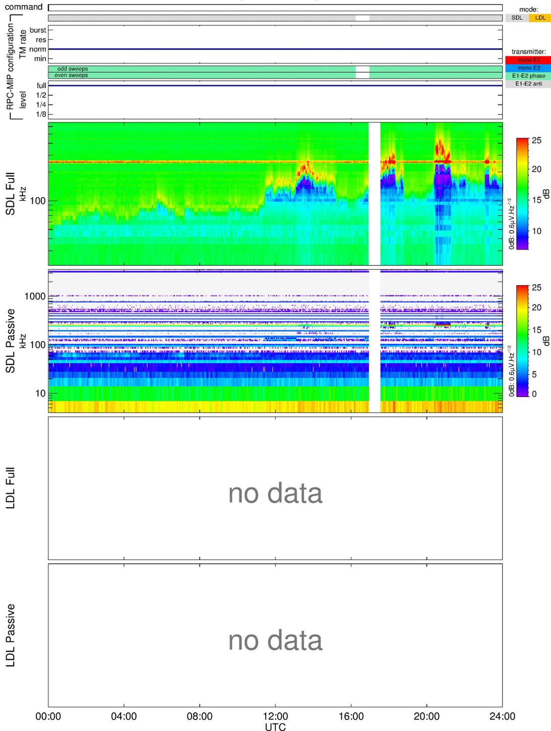
**Figure 2:** Example of a 24-hours browse file, for 20160814. Figure shows, from top to bottom: instrument related parameters (HK), power spectrogram in SDL active mode, power spectrogram in SDL passive mode, power spectrogram in LDL active mode, power spectrogram in LDL passive mode. For this day, RPC-MIP was operated in SDL mode, so that LDL plots are empty (as indicated by the “no data” caption).
