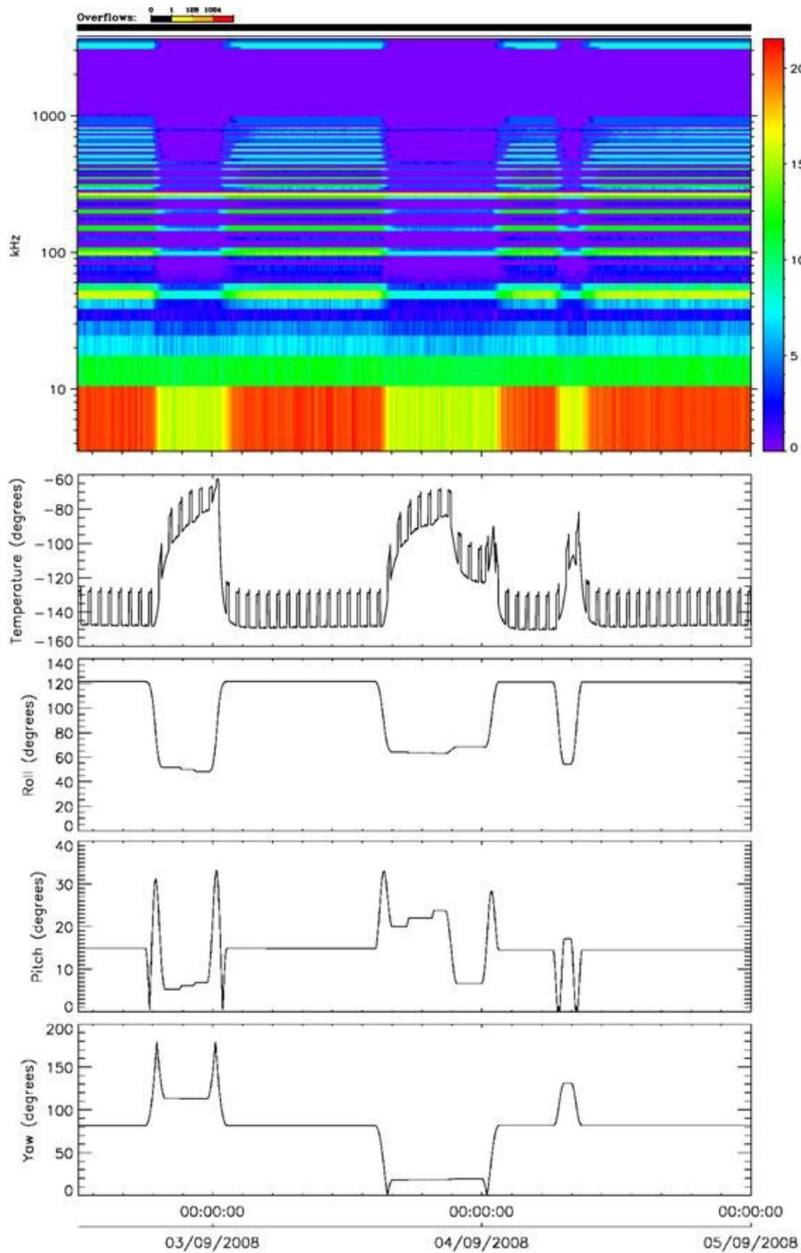
**Figure 5:** Example of temperature effect. From top to bottom: RPC-MIP E-field passive power spectrogram, R2 temperature, roll angle, pitch angle, yaw angle.
