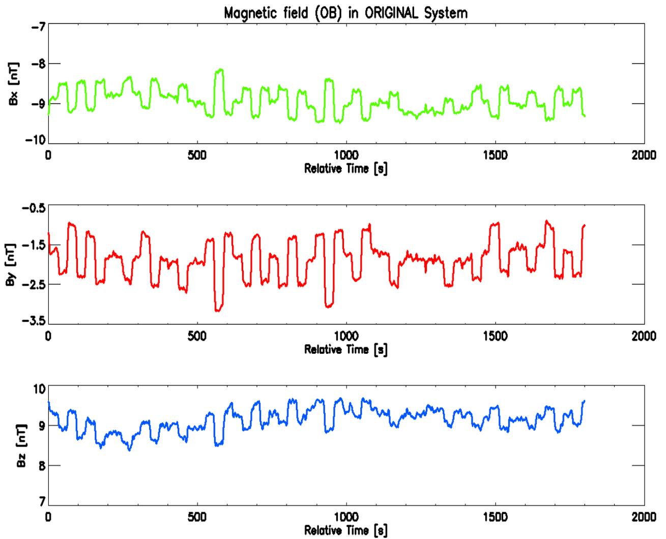
Figure 2: Original Signal disturbed by the LANDER heaters
