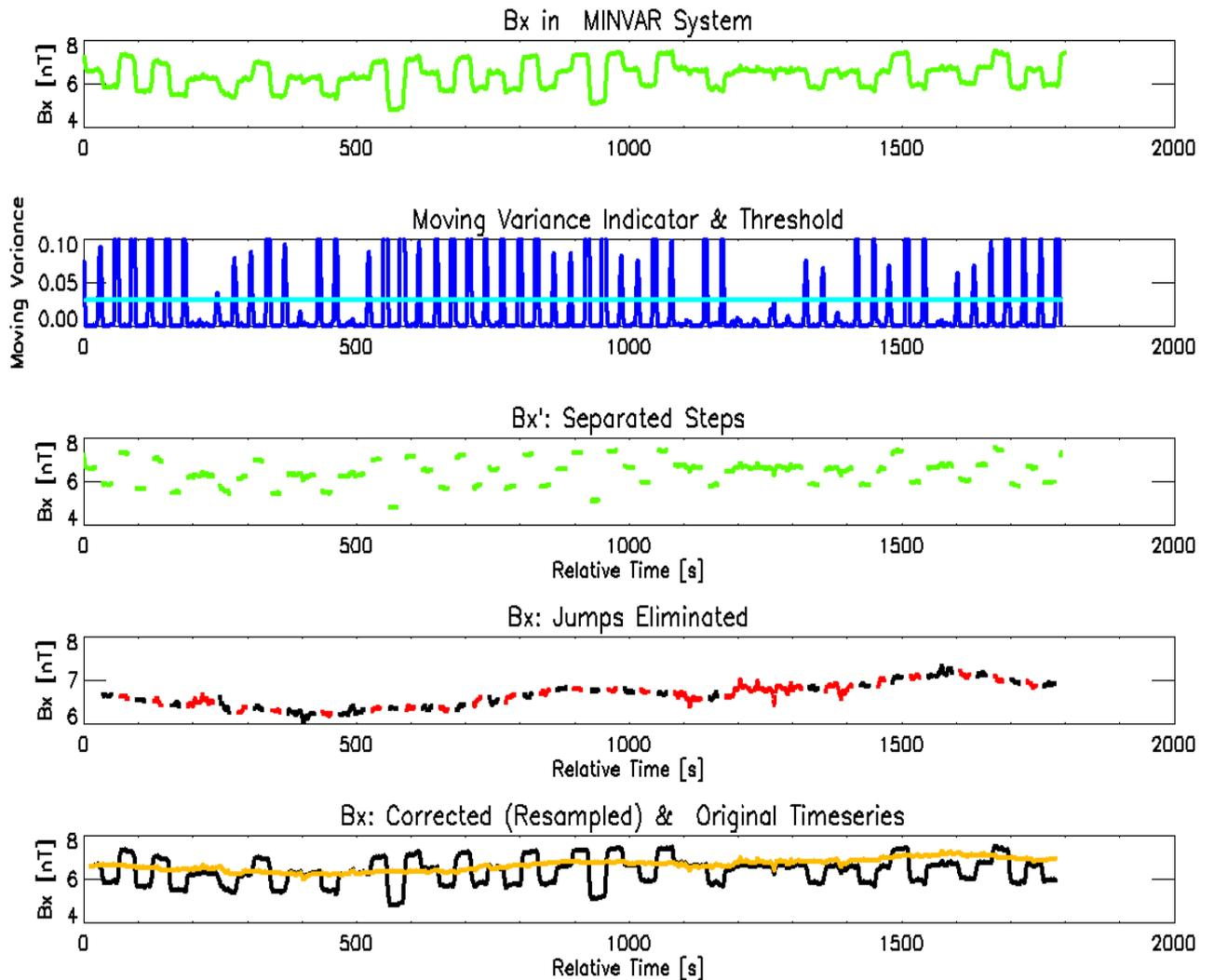
Figure 4: Processing of the heater disturbed Signal
